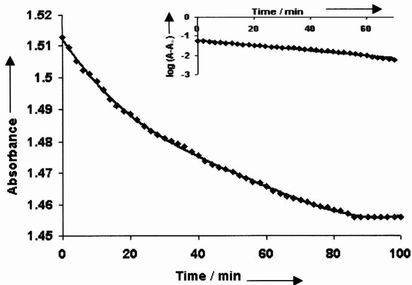
**Figure 4.** Observed changes in absorbance versus time and plot of  $\log (A-A_{\infty})$  vs. time (inset) plot measured at 260 nm for UV-absorbing intermediates generated during electrooxidation of adenosine at PGE, pH 7.0.
