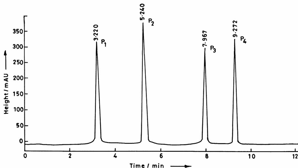
**Figure 5.** A typical HPLC chromatogram observed for the products of adenosine in Britton-Robinson buffer of pH 7.0.
