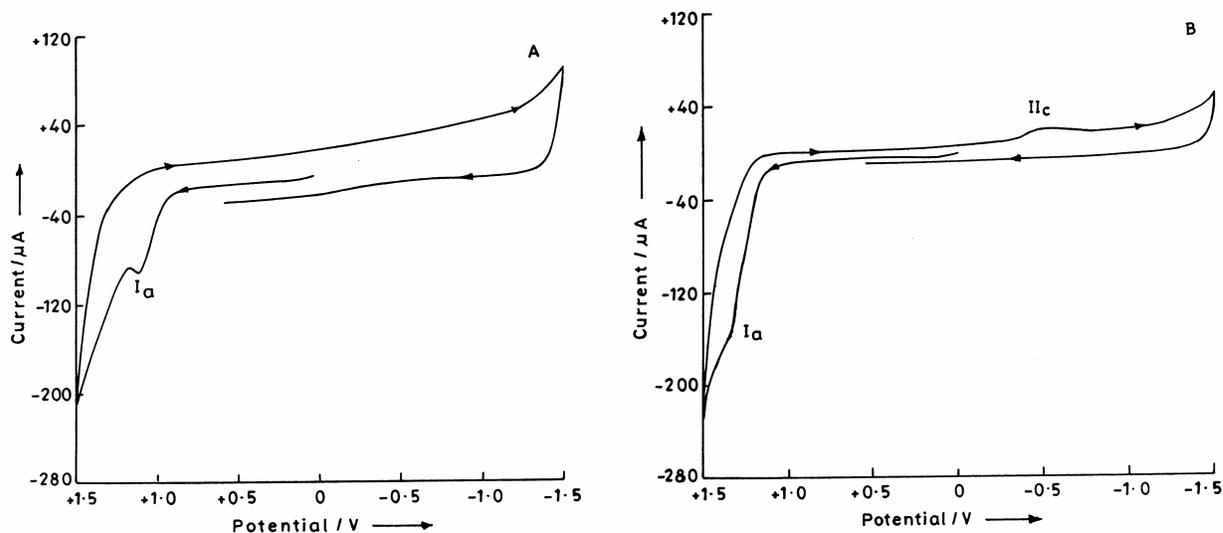
**Figure 1.** A comparison of cyclic voltammograms of 1.0 mM adenosine in Britton-Robinson buffer (A) and phosphate buffer (B) of pH 7.0 at PGE.
