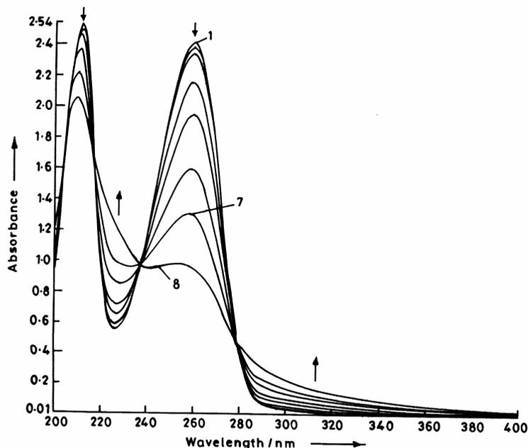
**Figure 3.** UV spectrum of 0.1 mM adenosine in Britton-Robinson buffer of pH 7.0 at PGE. Curves were recorded at (1) 0 (2) 5 (3) 10 (4) 20 (5) 30 (6) 50 (7) 70 (8) 100 min of electrolysis.
