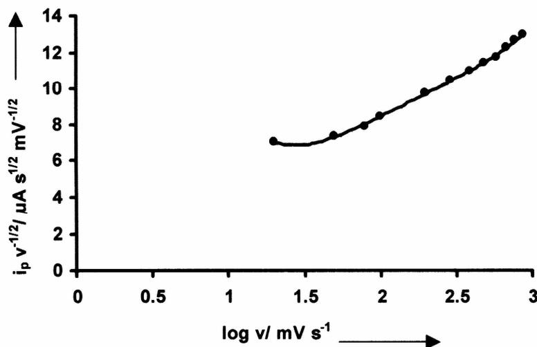
**Figure2.** Dependence of the peak current function ( $i_p/\sqrt{v}$ ) with the logarithm of the sweep rate ( $\log v$ ) for voltammetric peak  $I_a$  of adenosine at pH 7.0, PGE.
