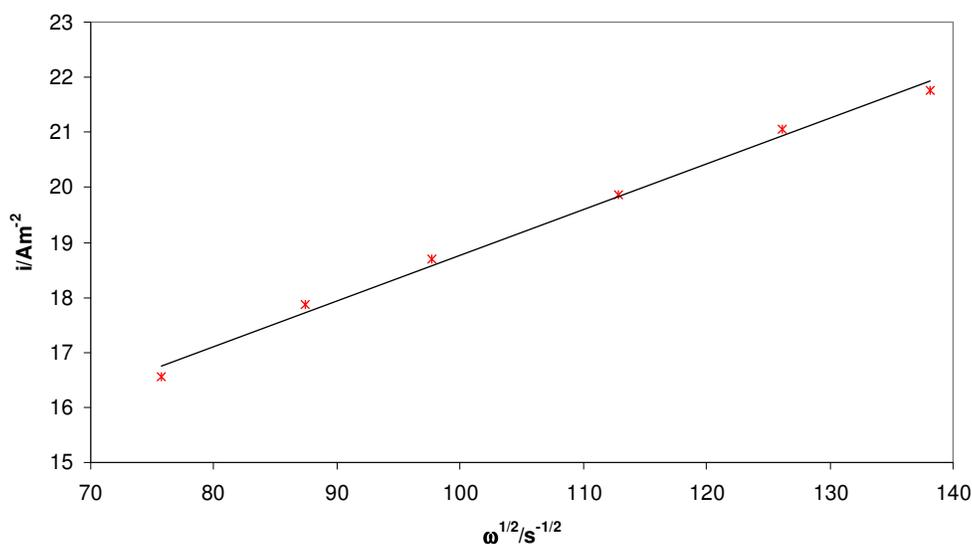
**Figure 4.** Limiting current density plotted versus the square root of the rotation rate of the electrode. The electrode potential is 1.13 V.
