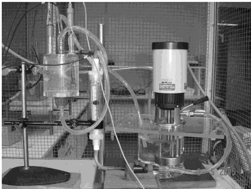
**Figure 2.** Wall-jet flow cell with pump unit.
