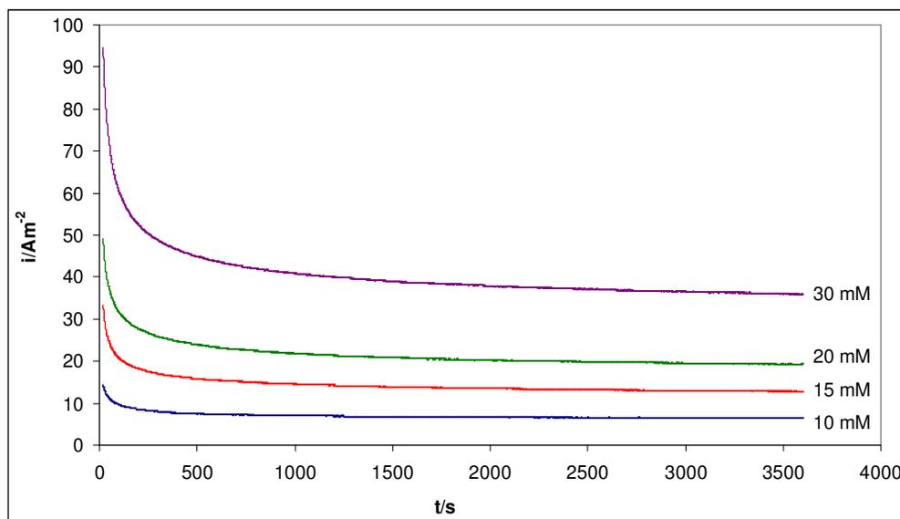
**Figure 6.** Current density plotted versus time for different concentrations of sulphite, at a constant potential of 1.0 V SCE. The data are taken from a wall-jet flow cell with a constant flow rate of 1.2 L/min. The pH is 11.
