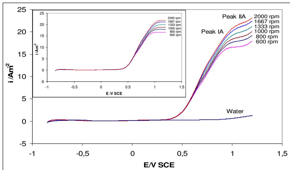
**Figure 3.** Cyclic voltammograms of a 10 mM sodium sulphite solution on a RDE (600-2000 rpm) with a scan rate of 40 mV/sec and for water (1000 rpm) with a scan rate of 20 mV/sec. In the insert the current contribution from the water oxidation has been subtracted. All experiments are performed at pH 11.
