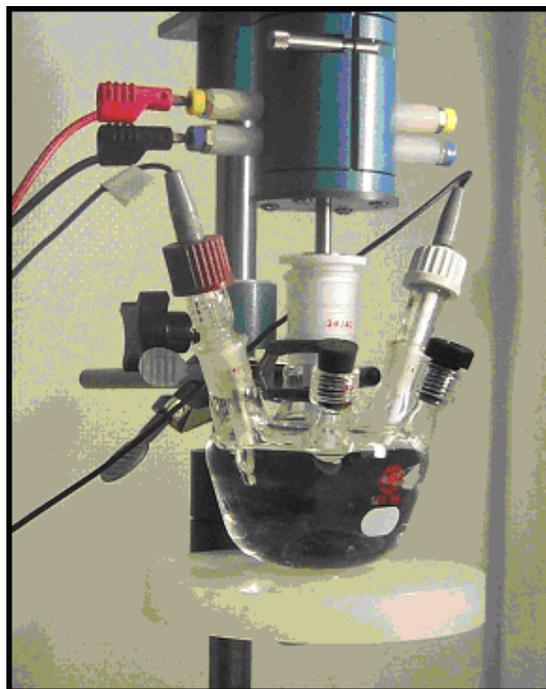
**Figure 1.** Cell with rotating disk electrode equipment.
