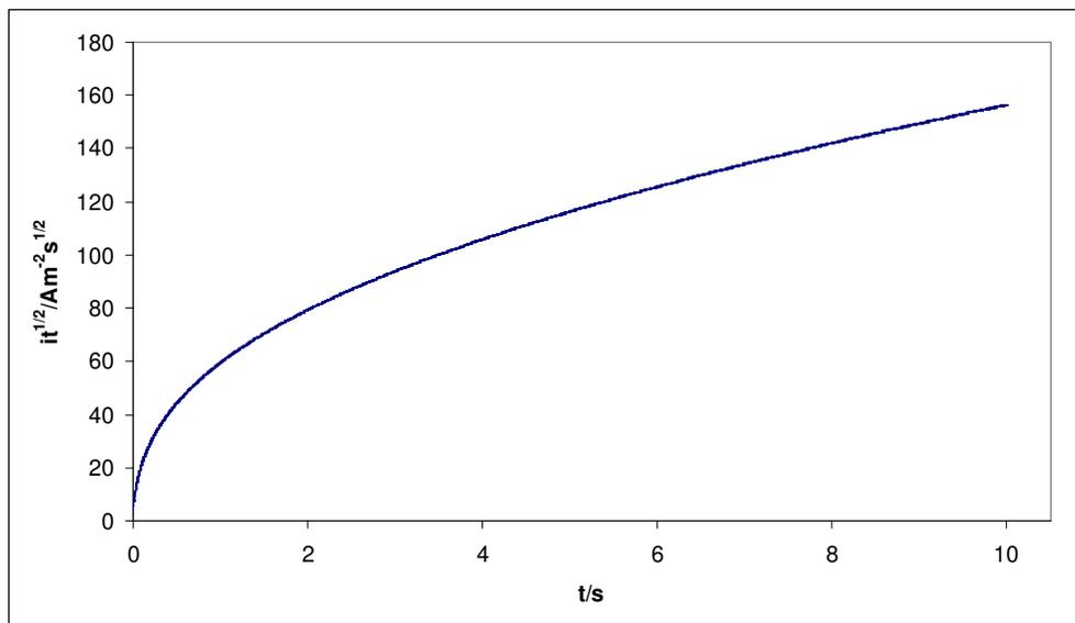
**Figure 5.**  $i \cdot t^{1/2}$  as a function of time for the oxidation of 20 mM sulphite solution on a stationary platinum electrode at 1.05 V, pH 11.
