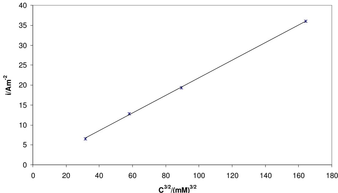
**Figure 8.** Current density plotted against  $(C_{SO_3^{2-}})^{3/2}$ . The current data are obtained after 3600 seconds in Figure 6.
