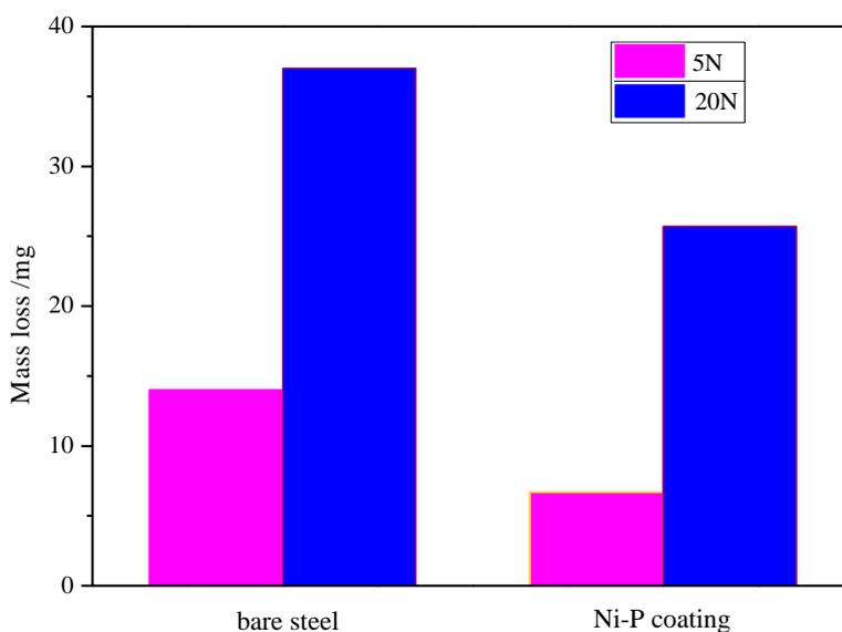
Figure 8. Mass loss of the bare anchor rod and Ni-P coating by dry-sliding wearing
