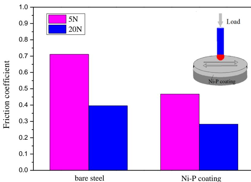
Figure 7. Friction coefficients of bare anchor rod substrate the Ni-P coating
