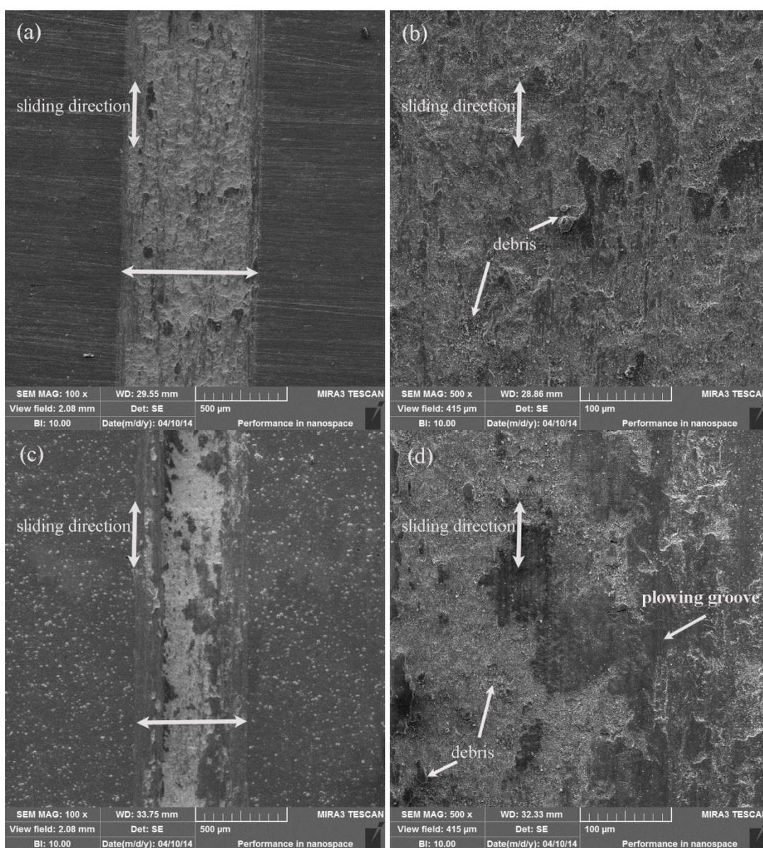
**Figure 9.** SEM images showing wore surface morphologies of raw material and the Ni-P coating under a load of 5 N (a)anchor rod 100× (b)anchor rod 500× (c)Ni-P coating 100× (d)Ni-P coating 500×
