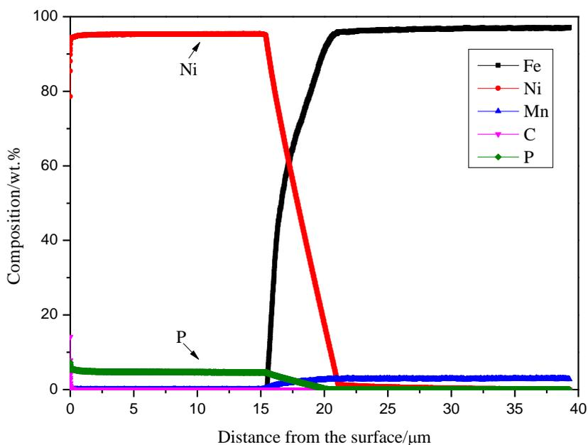
Figure 5. Glow discharge optical emission spectrometry (GDOES) profile of as-plated Ni-P coating
