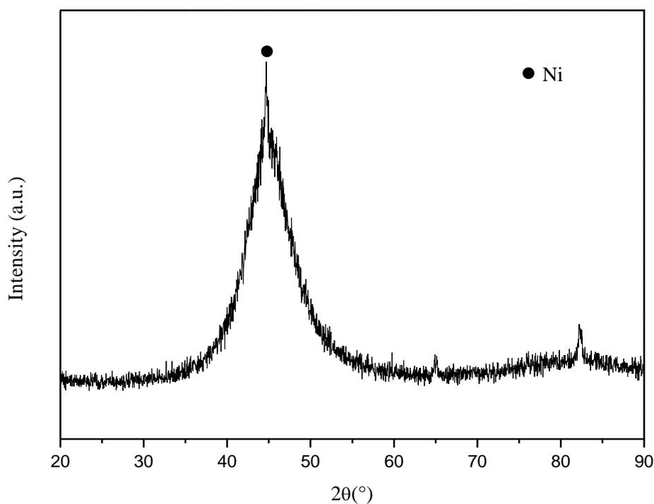
**Figure 3.** XRD pattern of as-plated Ni-P coating
