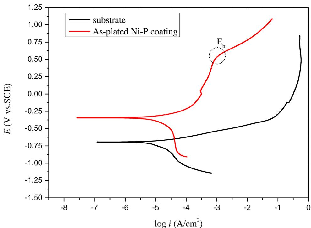
**Figure 11.** Electrochemical polarization curves of anchor rod substrate and as-plated Ni-P coating in 5 wt. % sodium chloride solution
