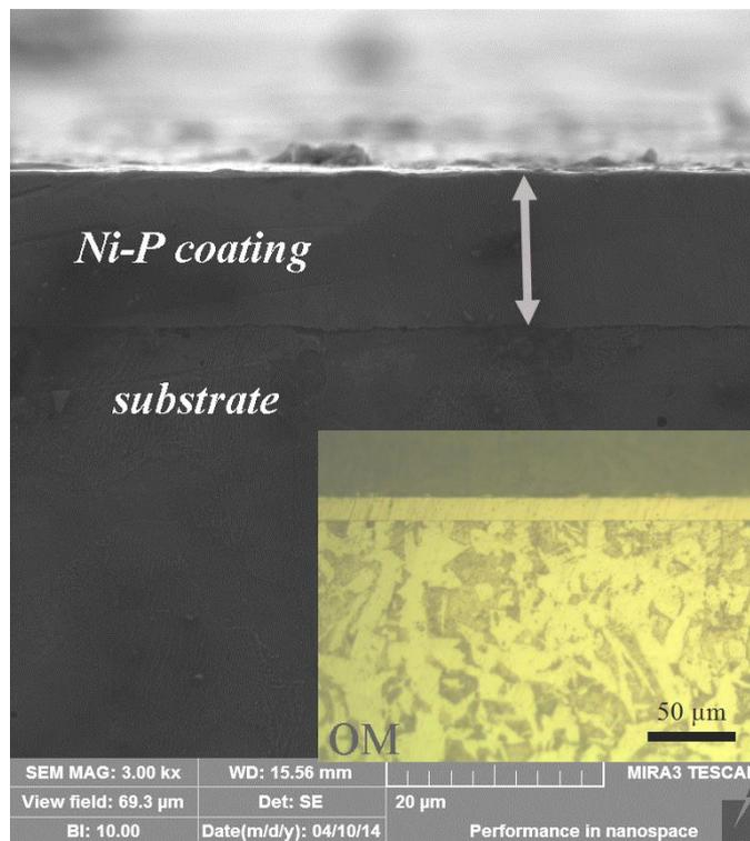
Figure 4. Cross section morphology of the Ni-P coating
