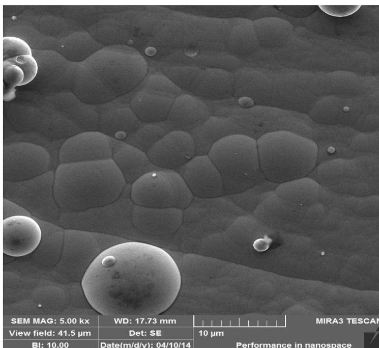
**Figure 2.** Surface morphology of as-plated Ni-P coating
