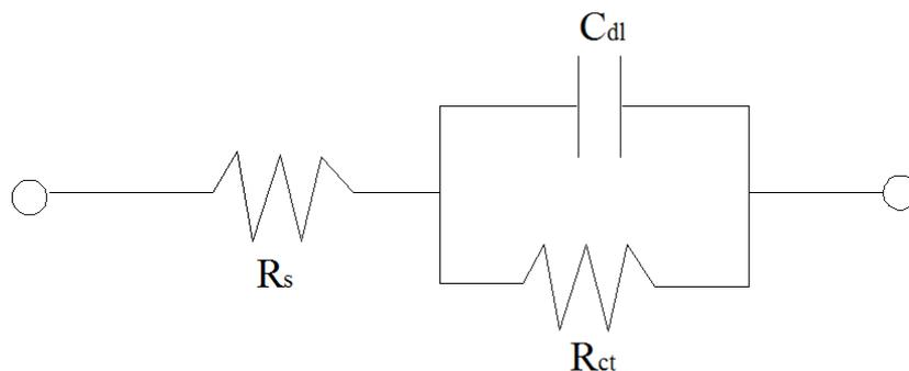
**Figure 13.** Equivalent electrical circuit model used to analyze the EIS data of plated Ni-P coating
