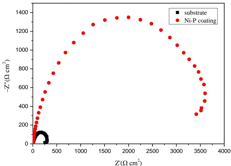
**Figure 12.** Nyquist plot for anchor rod substrate and as-plated Ni-P coating in 5 wt. % sodium chloride solution
