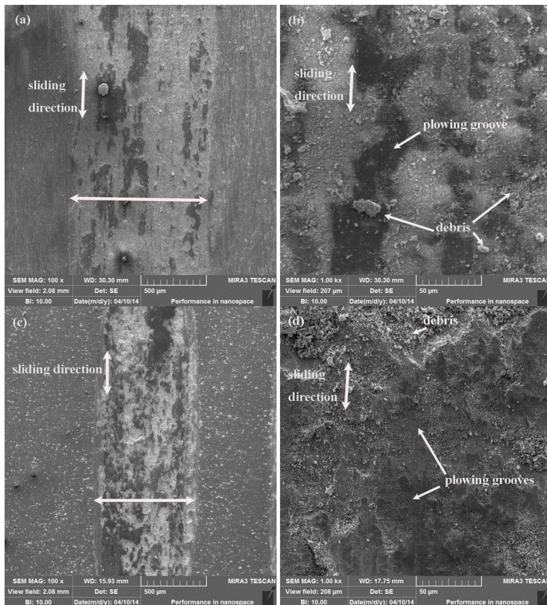
**Figure 10.** SEM images showing wore surface morphologies of raw material and the Ni-P coating under a load of 20 N (a)anchor rod 100× (b)anchor rod 1000× (c)Ni-P coating 100× (d)Ni-P coating 1000×
