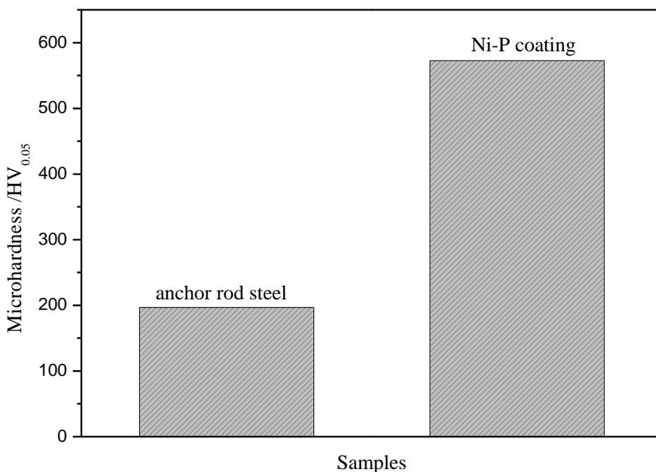
**Figure 6.** Surface microhardness of bare and Ni-P coated RB400 steel samples
