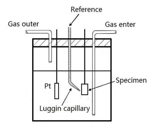
Figure 1. Schematic diagram showing the three electrode system used.
