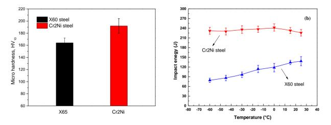
Figure 2. (a) Vickers hardness and (b) impact toughness values of X60 and Cr2Ni steels under different temperatures.
