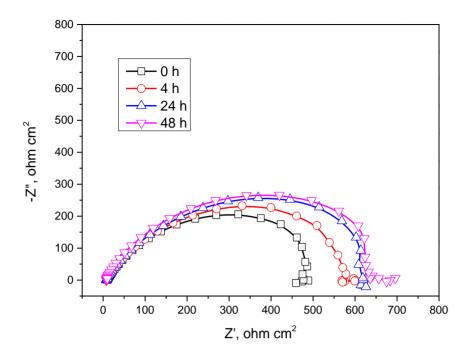
Figure 7. Nyquist diagrams of X60 steel obtained after the immersion of 0, 4, 24, and 48 h.
