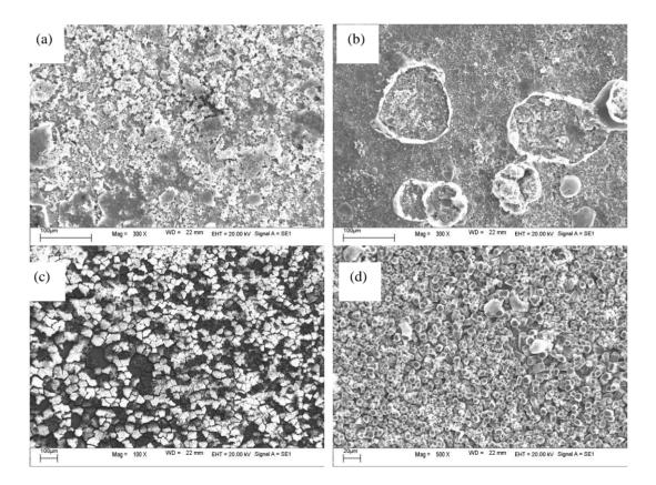
**Figure 5.** Microscopic morphologies of corrosion films on (a, b) X60 and (c, d) Cr2Ni samples though 30 days immersion in test solutions.
