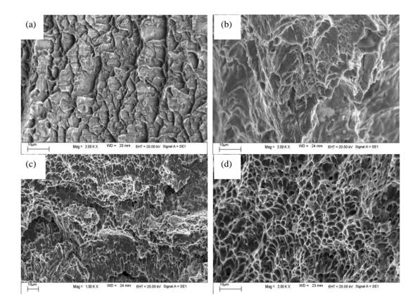
**Figure 3.** SEM photos showing the impact fracture surfaces of X60 and Cr2Ni steels under different temperatures (a) X60, -80 °C; (b) X60, 25 °C; (b) Cr2Ni, -80 °C; (b) Cr2Ni, 25 °C.
