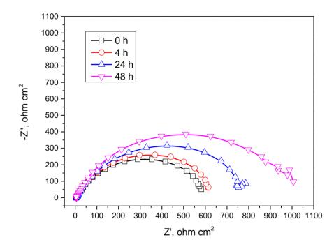
Figure 8. Nyquist diagrams of Cr2Ni steel obtained after the immersion of 0, 4, 24, and 48 h.
