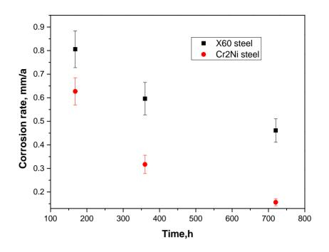
Figure 4. Corrosion rates of X60 and Cr2Ni steels after 7, 15, and 30 days immersion in test solutions.
