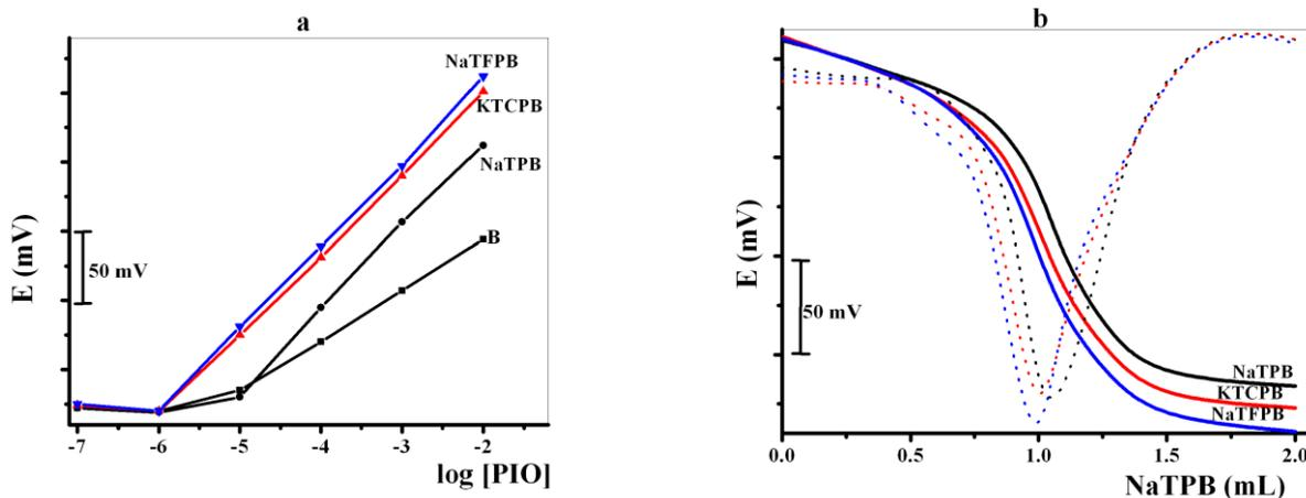
**Figure 3.** Effect of ionic sites on pioglitazone electrode performance; where dashed lines are for the first derivatives of the titration curves.
