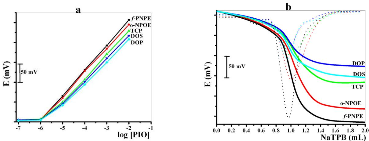
**Figure 4.** Effect of plasticizer on pioglitazone electrode performance; where dashed lines are for the first derivatives of the titration curves.
