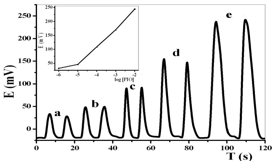
**Figure 4.** A) FIA potentiometric determination of PIO using 15-crown-5 ether based sensors: (a)  $10^{-6}$ , (b)  $10^{-5}$ , (c)  $10^{-4}$ , (d)  $10^{-3}$  and (e)  $10^{-2}$  mol  $\text{L}^{-1}$ .
