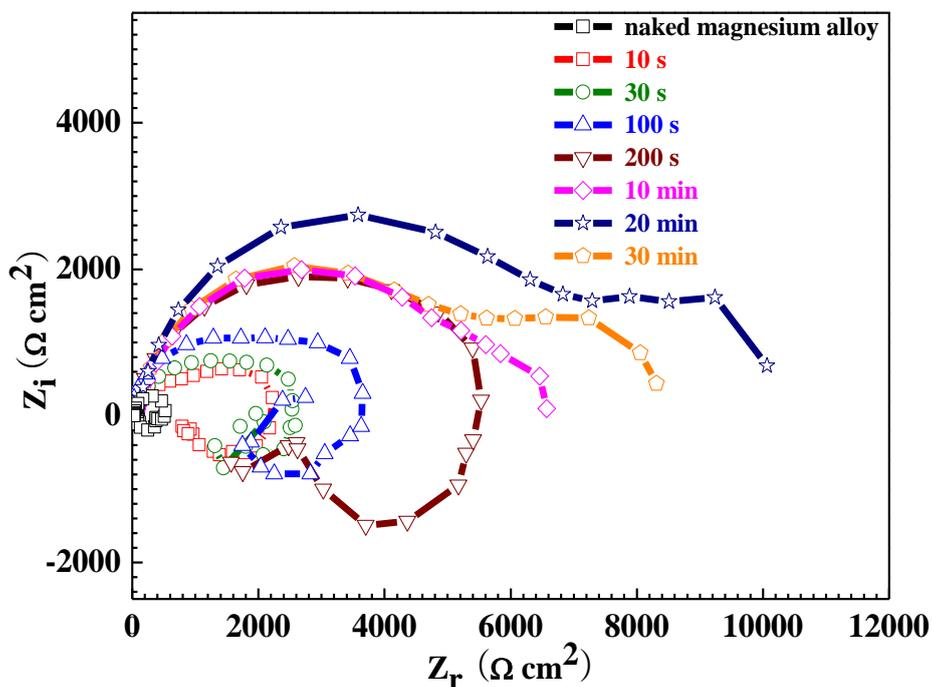
**Figure 3.** Nyquist plots of the naked magnesium alloy and the phosphated magnesium alloys immersed in the phosphating bath with different time.
