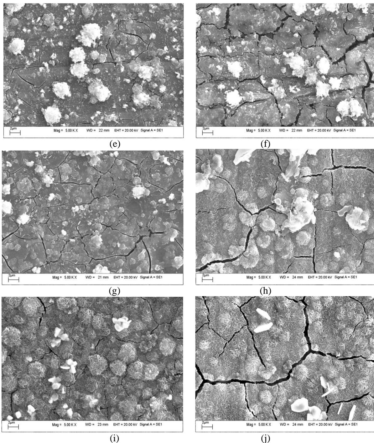
**Figure 2.** Surface SEM morphologies of the magnesium alloy sample immersed in the phosphating bath with different time: (a) 0 s, (b) 10 s, (c) 30 s, (d) 40 s, (e) 100 s, (f) 200 s, (g) 5 min, (h) 10 min, (i) 20 min and (j) 30 min.
