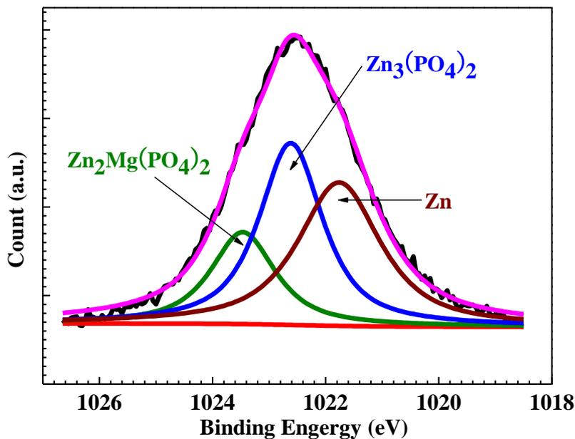
**Figure 6.** High-resolution XPS spectrum of Zn 2p of the phosphate conversion coating formed in the phosphating bath at 45 °C for 20 min.
