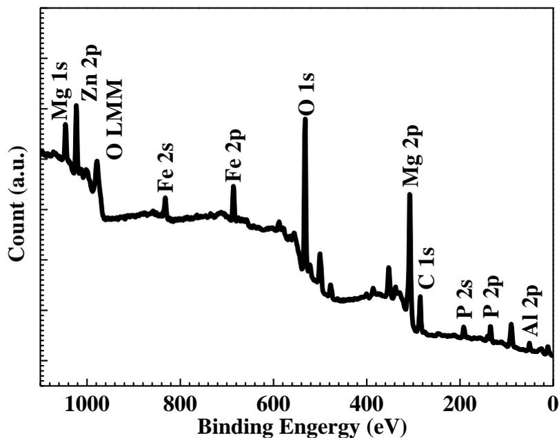
**Figure 5.** Wide-scan XPS spectrum of the phosphate conversion coating formed in the phosphating bath at 45 °C for 20 min.
