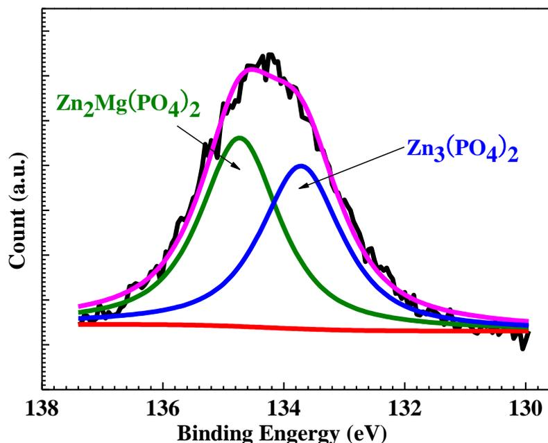
**Figure 7.** High-resolution XPS spectrum of P 2p of the phosphate conversion coating formed in the phosphating bath at 45 °C for 20 min.
