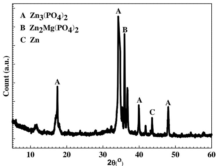
**Figure 4.** XRD spectrum of the phosphate conversion coating formed in the phosphating bath at 45 °C for 20 min.
