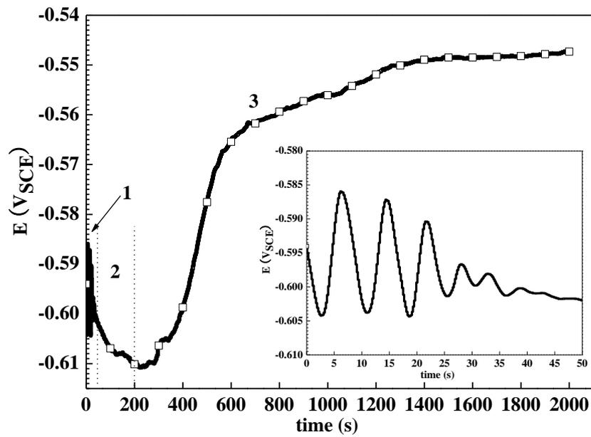
**Figure 1.** Potential-time curve of magnesium alloy AZ91D immersed in the phosphating bath at 45 °C.
