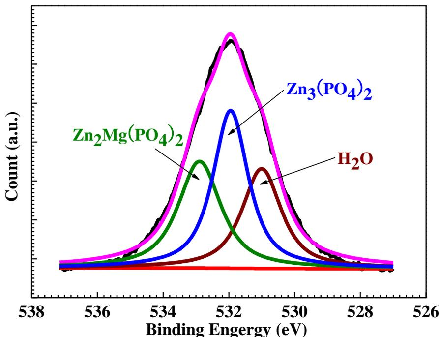
**Figure 8.** High-resolution XPS spectrum of O 1s of the phosphate conversion coating formed in the phosphating bath at 45 °C for 20 min.
