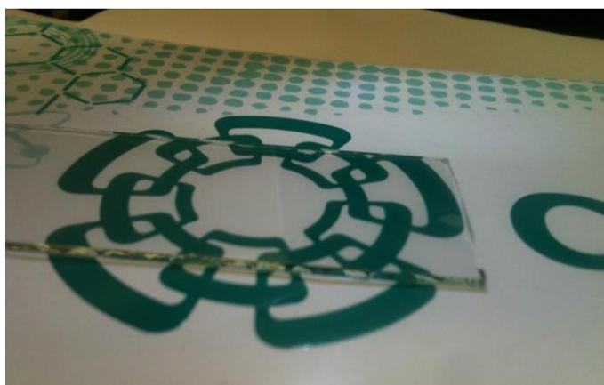
**Figure 1.** Photograph showing the image of the homogeneous and highly transparent PMMA-TiO<sub>2</sub> hybrid films.
