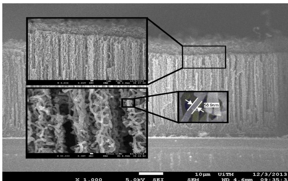
**Figure 2.** SEM image of synthesized MWCNTs
