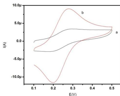
**Figure 5.** a) Cyclic voltammograms of the GOx/MWCNTs/GI/GCE at scan rate of  $20 \text{ mV/s}$  in  $0.1 \text{ M}$  nitrogen saturated PBS and  $0.5 \text{ mM}$  potassium ferricyanide, a) in absence of glucose, b) in the presence of  $1.3 \text{ mM}$  glucose.
