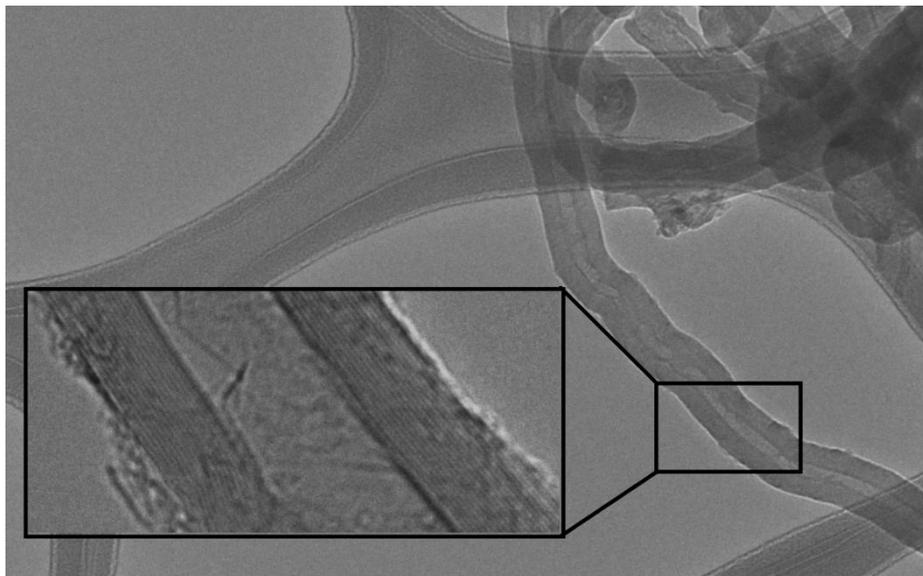
**Figure 3.** TEM image of synthesized MWCNTs
