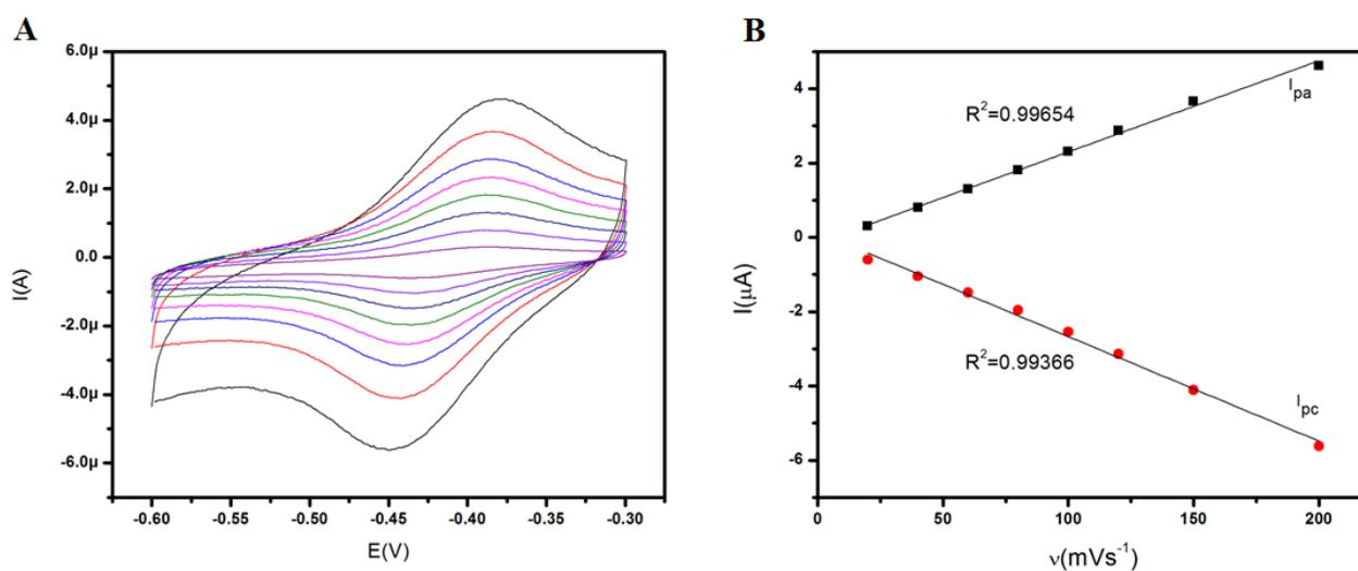
**Figure 4.** A) Cyclic voltammograms of the GOx/MWCNTs/GI/GCE in 0.1 M PBS with nitrogen saturated at different scan rates (from inner to outer curves: 20, 40, 60, 80, 100, 120, 150, 200 mV/s). B)  $I_{pa}$  and  $I_{pc}$  vs. scan rates.
