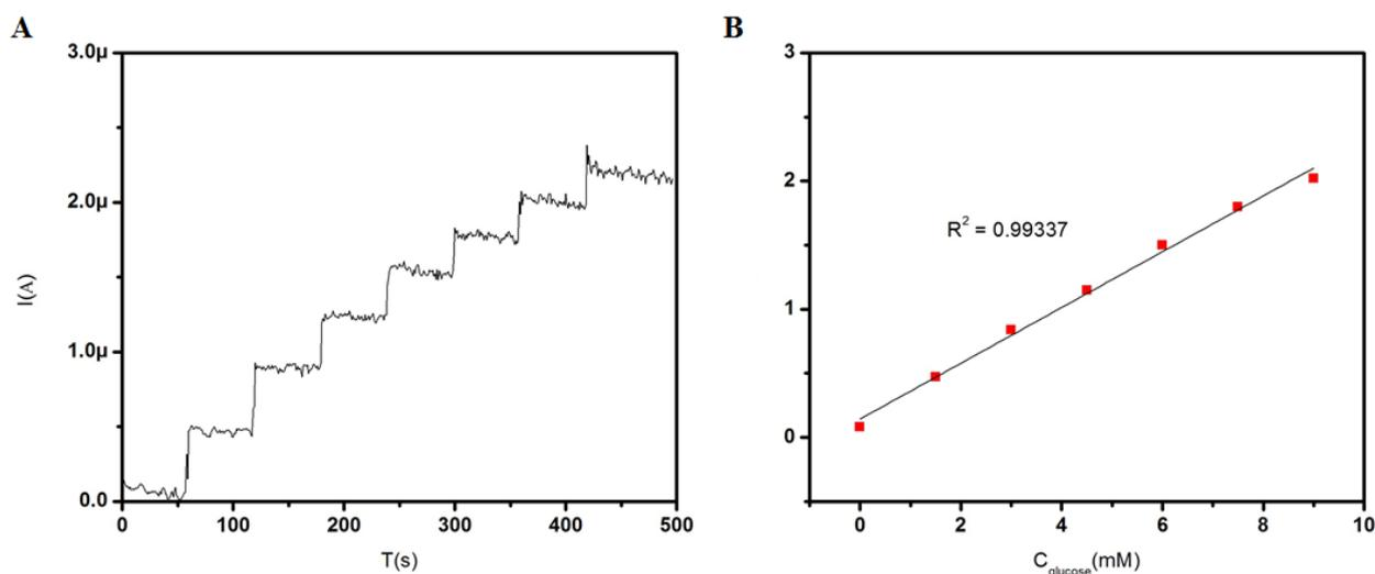
**Figure 6.** **A)** The chronoamperometric response of GOx/MWCNTs/GI/GCE on successive addition of 1.3 mM glucose in each successive adding at applied potential of +.3 V. **B)** The calibration curve of the electrocatalytic current on different concentration of glucose.
