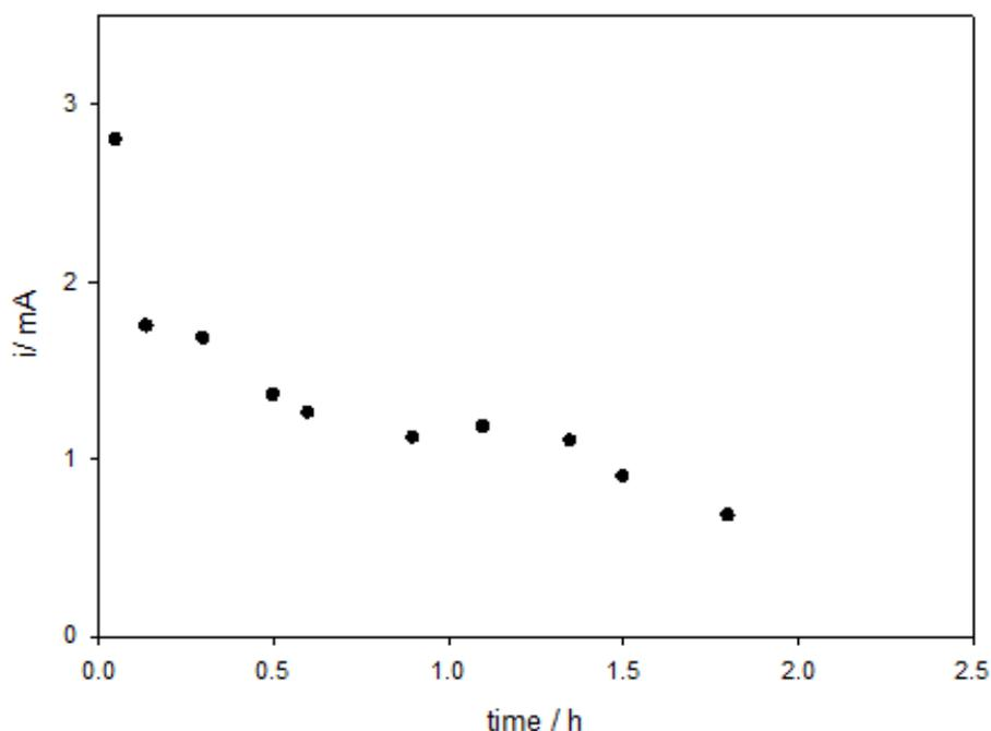
**Figure 4.** The current *versus* time: 0.11 mM  $\text{Fe}(\text{PFTPP})\text{Cl}$  in the presence of  $\text{CO}_2$  and 1.5 M  $\text{CF}_3\text{CH}_2\text{OH}$  in MeCN-5 % DMF containing 0.1 M  $\text{NBu}_4\text{BF}_4$ , at p-type Si electrode.
