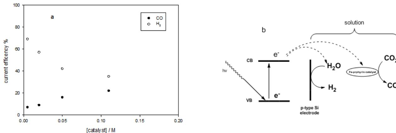
**Figure 6.** (a) Current efficiency of CO and H<sub>2</sub> formation for different concentrations of catalyst, (b) Heterogeneous catalytic role of p-type Si for H<sub>2</sub> reduction from H<sub>2</sub>O and the Fe-porphyrin role as CO<sub>2</sub> reduction catalysts [14].
