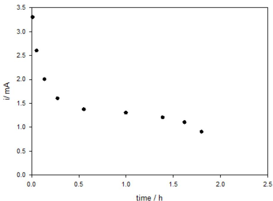
**Figure 3.** The current *versus* time: 0.11 mM Fe(PFTPP)Cl in the presence of CO<sub>2</sub> and 1.5 M CF<sub>3</sub>CH<sub>2</sub>OH in MeCN-5 % DMF containing 0.1 M NBu<sub>4</sub>BF<sub>4</sub>, at mercury pool cathode.
