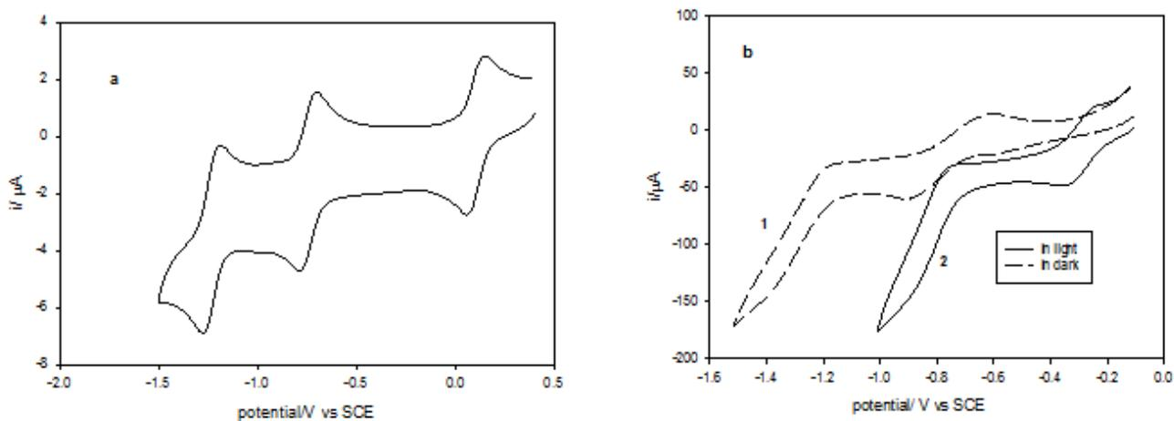
**Figure 1.** Cyclic voltammograms of Fe(PFTPP)Cl in a solvent mixture (MeCN-5 % DMF) containing 0.1 M NBu<sub>4</sub>BF<sub>4</sub> at a scan rate of 100 mV·s<sup>-1</sup>. (a) At a vitreous carbon electrode. (b) At an illuminated p-type H-Si electrode (1) in the dark, (2) illuminated under a Krüss halogen fibre optic lamp (90mW·cm<sup>2</sup>,  $\lambda_{\text{max}} = 650\text{nm}$ ).
