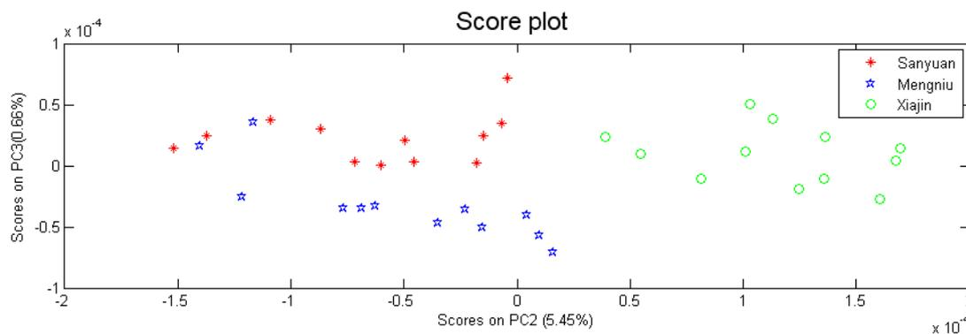
**Figure 3.** The score plot obtained from the current responses of the silver working electrode (PC2 and PC3)
