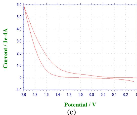
**Figure 1.** The current responses of staircase voltammetry from (a) the gold electrode, (b) the silver electrode and (c) the platinum electrode.
