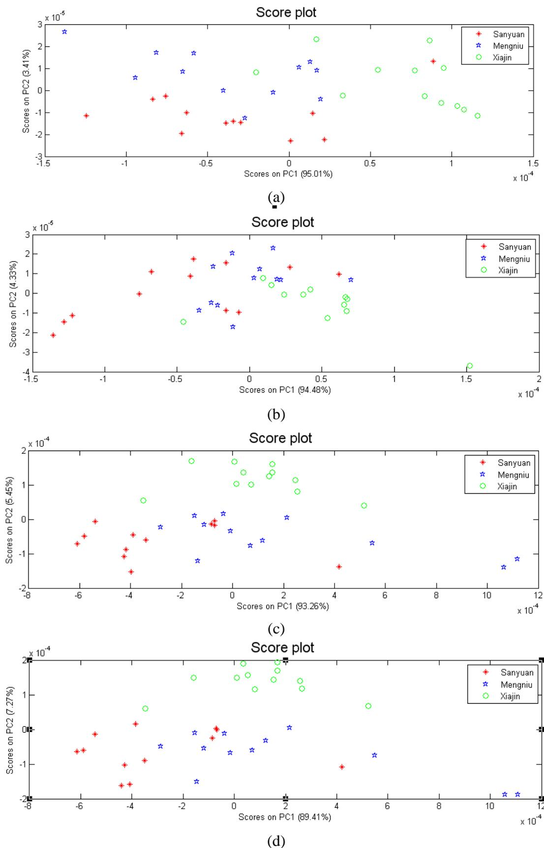
**Figure 2.** The score plots obtained from the current responses of (a) the gold working electrode, (b) the platinum working electrode, (c) the sliver working electrode and (d) all working electrode
