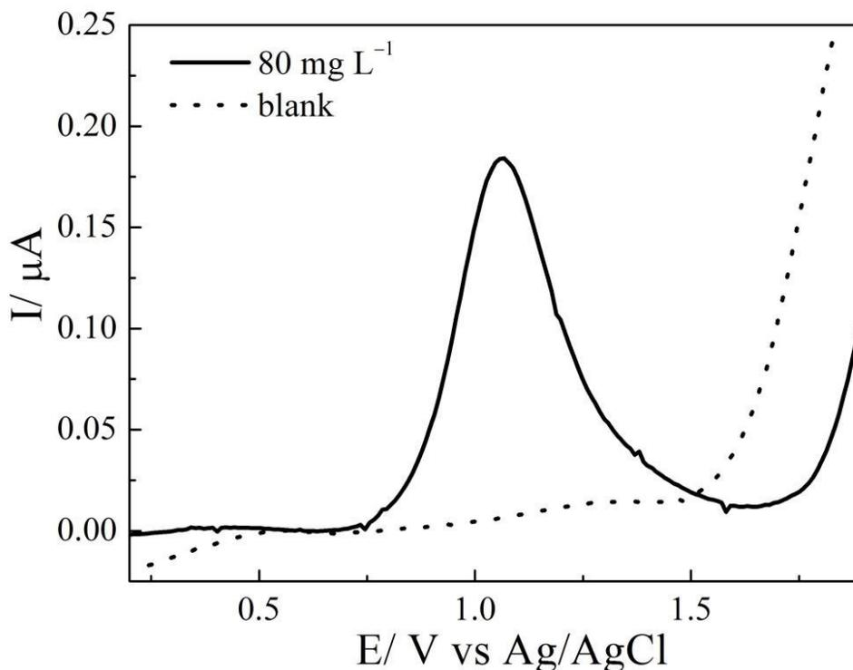
**Figure 1.** Voltammograms obtained by differential pulse voltammetry ( $E_{\text{step}} = 50 \text{ mV}$ ,  $a = 10 \text{ mV}$  and  $v = 20 \text{ mV s}^{-1}$ ) in the absence and presence of  $80 \text{ mg L}^{-1}$  morpholine in  $0.1 \text{ mol L}^{-1}$   $\text{LiClO}_4$  in acetonitrile using a platinum microelectrode.
