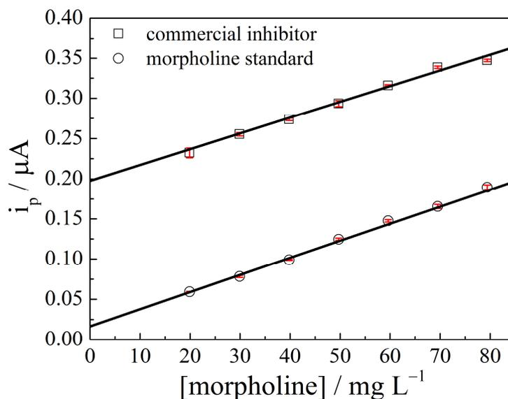
**Figure 5.** Analytical curves obtained in the absence and presence of the commercial inhibitor sample showing a linear response range from 20 to 80 mg L<sup>-1</sup>. Electrolyte solution: 0.1 mol L<sup>-1</sup> LiClO<sub>4</sub> in acetonitrile.
