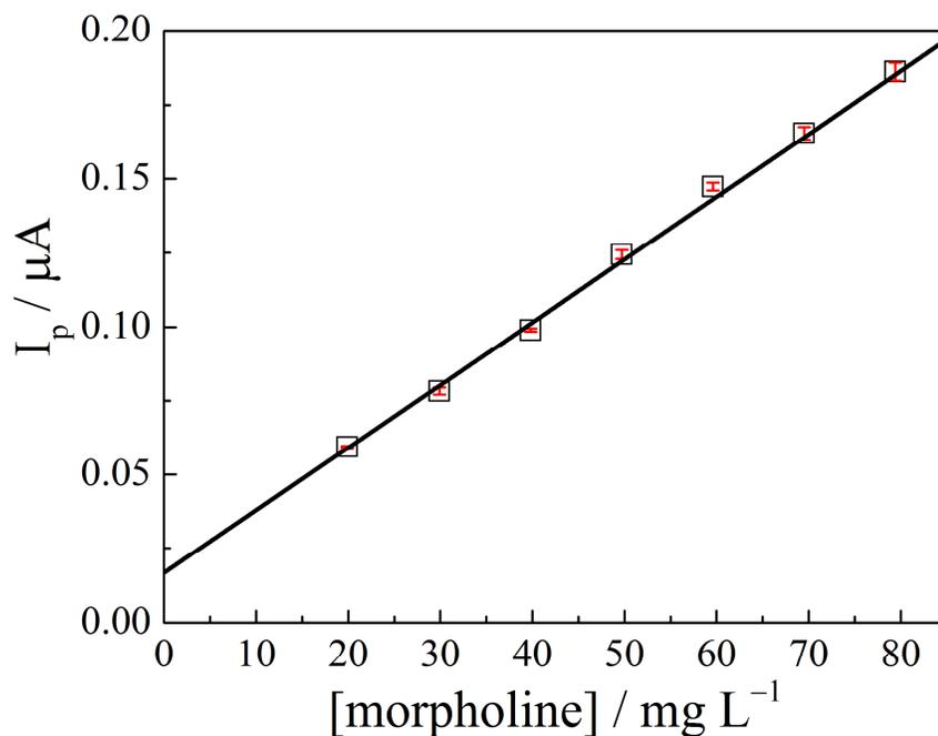
**Figure 2.** Analytical curve obtained for morpholine electro-oxidation showing a linear response range from 20 to 80 mg L<sup>-1</sup>. Electrolyte solution: 0.1 mol L<sup>-1</sup> LiClO<sub>4</sub> in acetonitrile.
