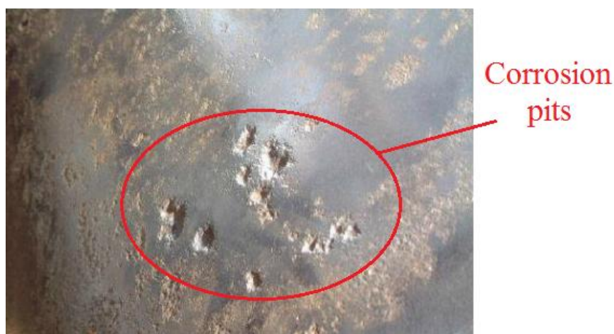
Figure 1. Corrosion pits of buried pipeline
