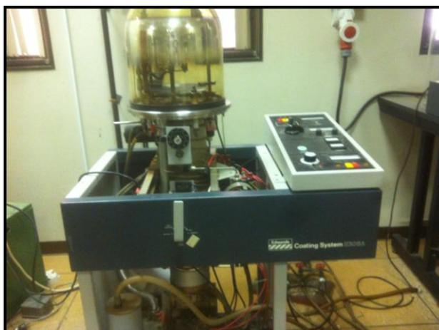
**Figure 1.** Edwards coating system type E303A that was employed as a thermal evaporator for Ni on the magnesium alloy AZ31.
