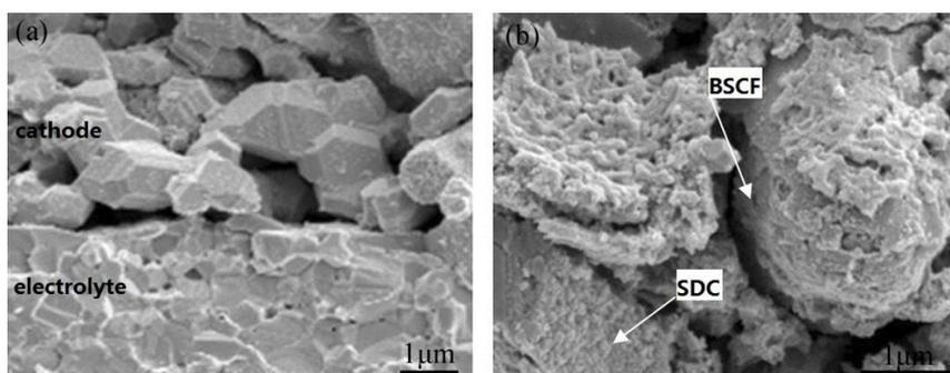
**Figure 1.** SEM micrographs: a) Cross-sectional view of BSCF matrix; b) Cross-sectional view of impregnated BSCF-SDC electrode.
