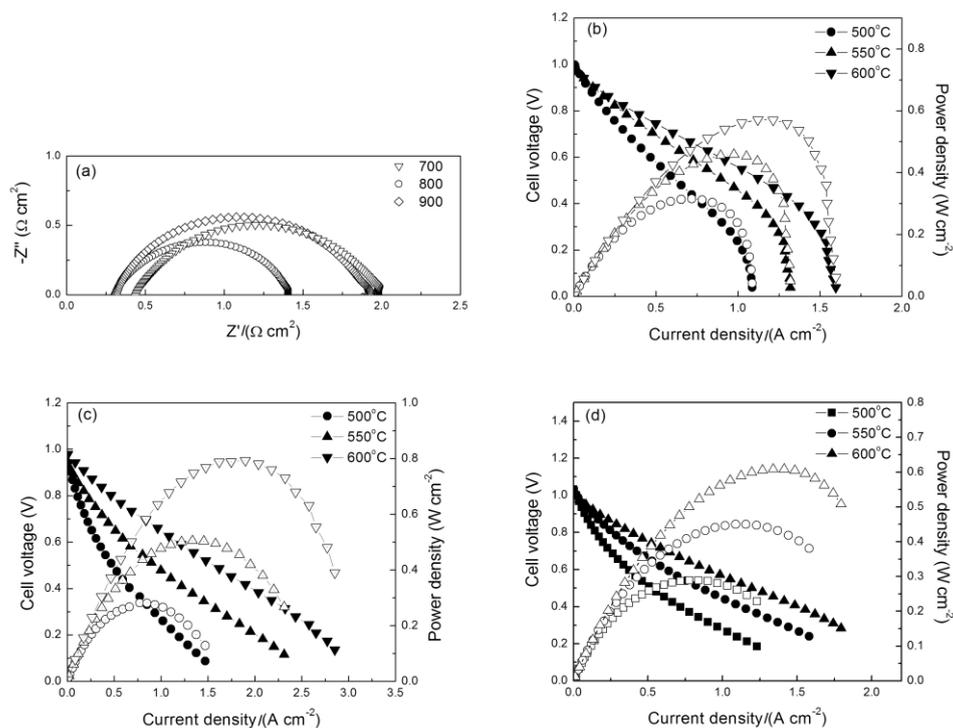
**Figure 3.** Electrochemical performance of single cells with impregnated SDC: a) Impedance spectra under open circuit conditions; b-d) Cell voltages (solid symbols) and power densities (open symbols) as function of current density of anode-supported cell using the impregnated cathodes with SDC heated to (b) 700 °C, (c) 800 °C and (d) 900 °C respectively.
