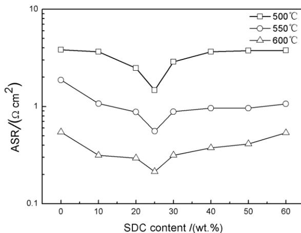
**Figure 2.** Area specific resistance (ASR) of the composite cathode as a function of the weight fraction of SDC
