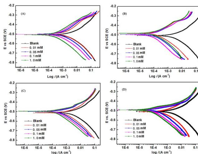
**Figure 2.** Tafel polarization curves for mild steel in 1.0 M HCl without and with different concentrations of inhibitors at 25 °C: (A) penicillin G, (B) oxacillin, (C) penicillin V, and (D) amoxicillin.
