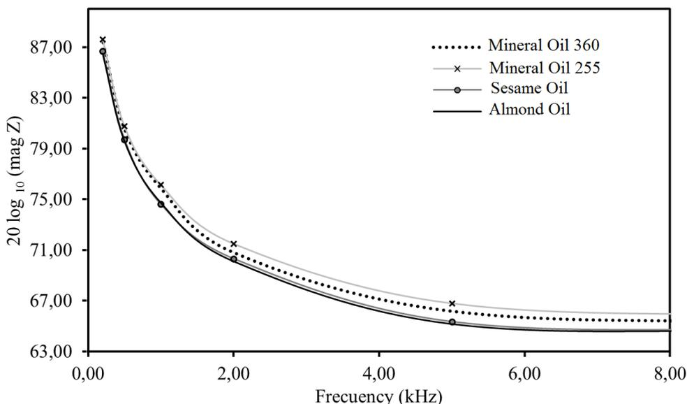
**Figure 6.** Comparison of the impedances of fresh vegetable and mineral oils.
