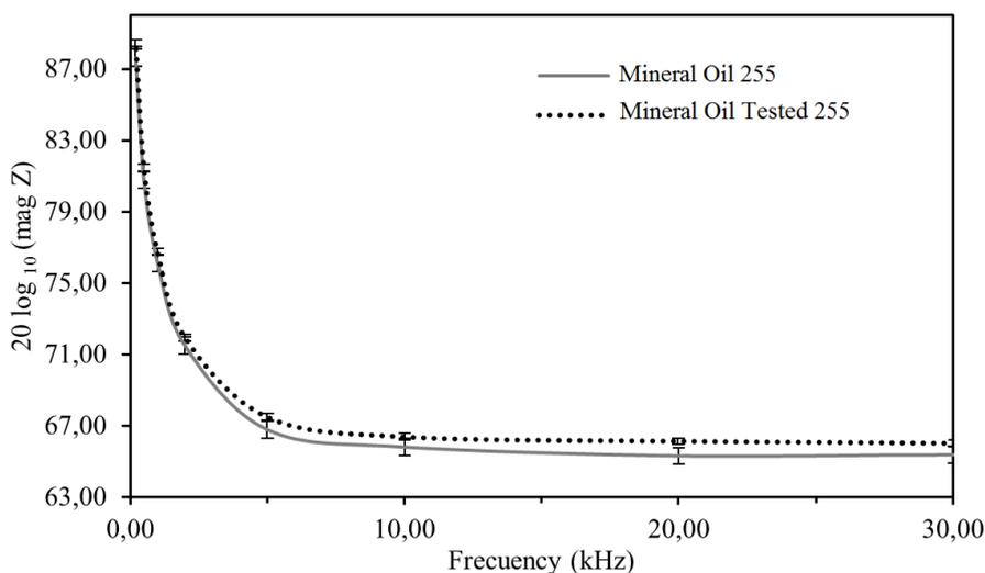
**Figure 4.** Comparison of the impedances of fresh and used mineral oil 255 in the AW tests. Frequency range from 0.2 to 30.0 kHz.
