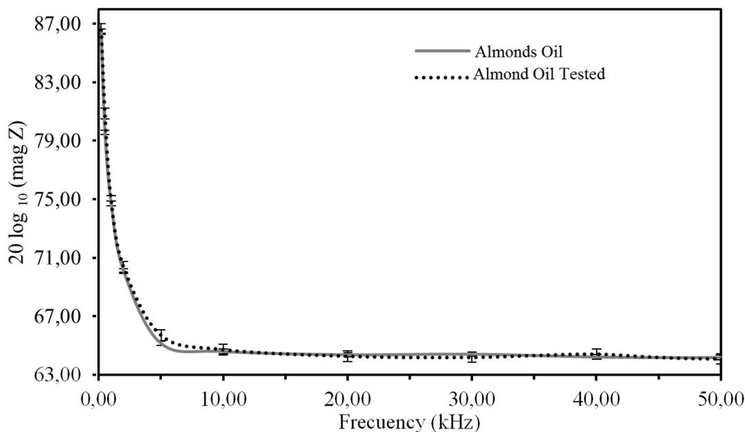
**Figure 3.** Comparison of the impedances of fresh and used sweet almond oil in the AW tests. Frequency range from 0.2 to 50.0 kHz.
