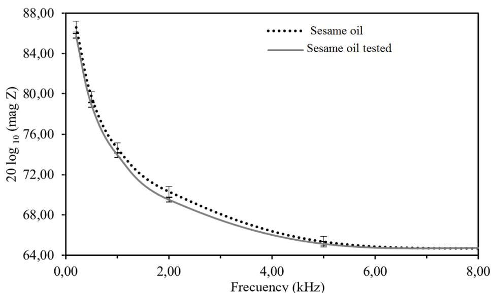
**Figure 2.** Comparison of the impedances of fresh and used sesame oil in the AW tests. Frequency range from 0.2 to 8.0 kHz.
