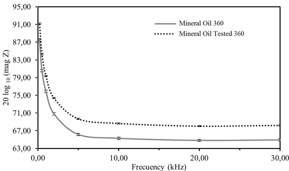
**Figure 5.** Comparison of the impedances of fresh and used mineral oil 360 in the AW tests. Frequency range from 0.2 to 30.0 kHz.
