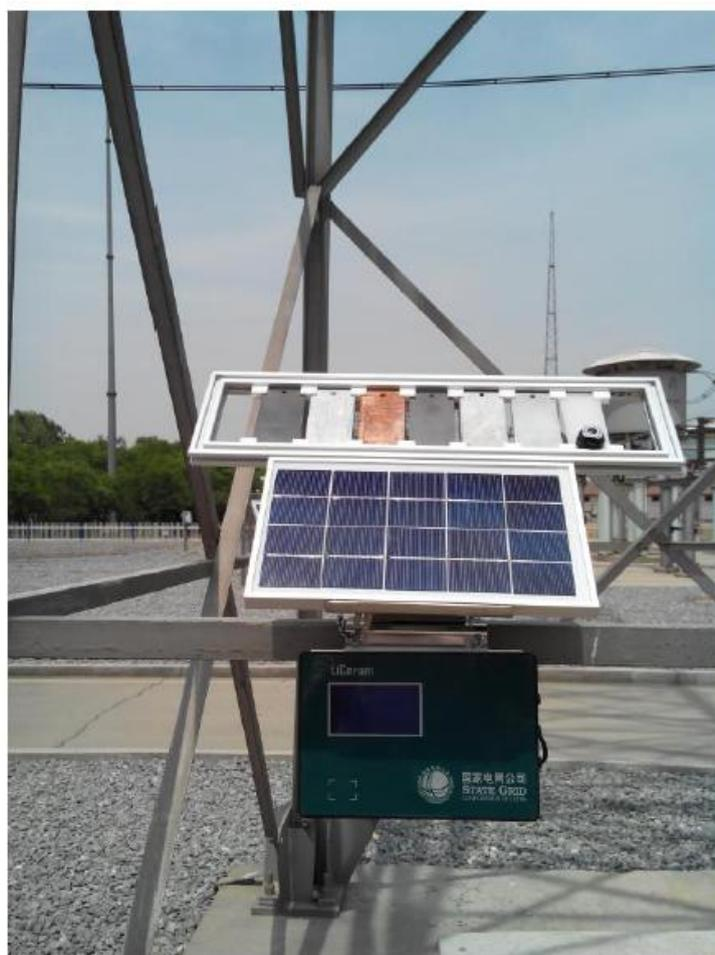
**Figure 3.** The photograph of the ACM in field exposure in Jiaodong site.
