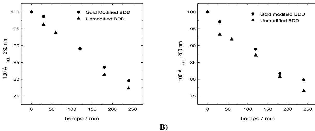
**Figure 5.** A) Relative absorbance decay for DEP electrolysis at 0,03 mA cm<sup>-2</sup> using gold modified BDD electrodes (circles) and unmodified BDD electrodes (triangles) for absorption band centered at 230 nm B) same as figure 5 A, for absorption band centered at 280 nm.
