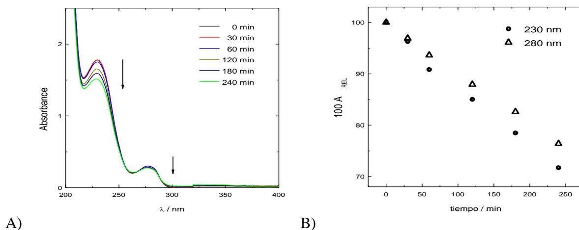
**Figure 3.** A) UV-vis spectra of 100 ppm DEP in 0.05 M  $\text{Na}_2\text{SO}_4$  electrolyte during the electrolysis using BDD anode at  $0.0 \text{ mA cm}^{-2}$ . B) relative absorbance decay for both absorption band (230 nm open circle, 280 nm open triangle) versus electrolysis time for data of figure 3 A.
