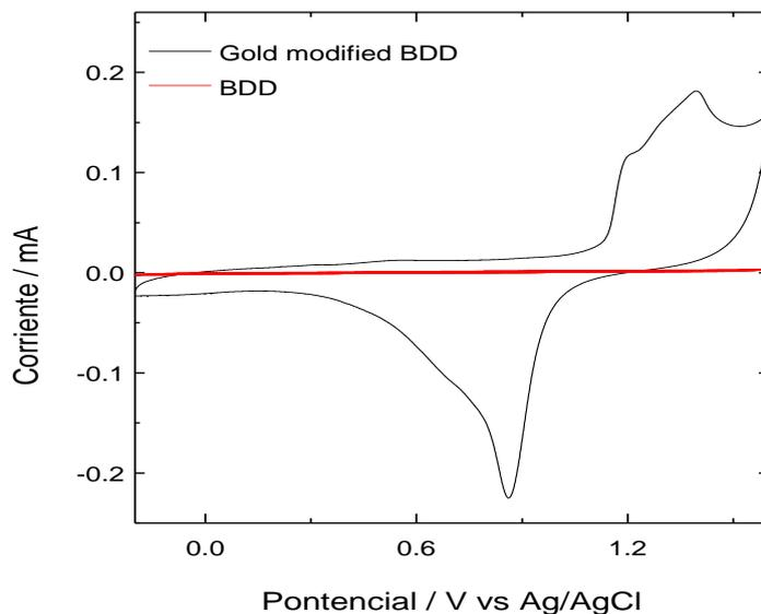
**Figure 1.** Voltammetric profile of a BDD electrode in 0.05 M H<sub>2</sub>SO<sub>4</sub> at 0,1 V s<sup>-1</sup>, before (red line) and after (black line) electrodeposited of gold particles in the BDD surface.
