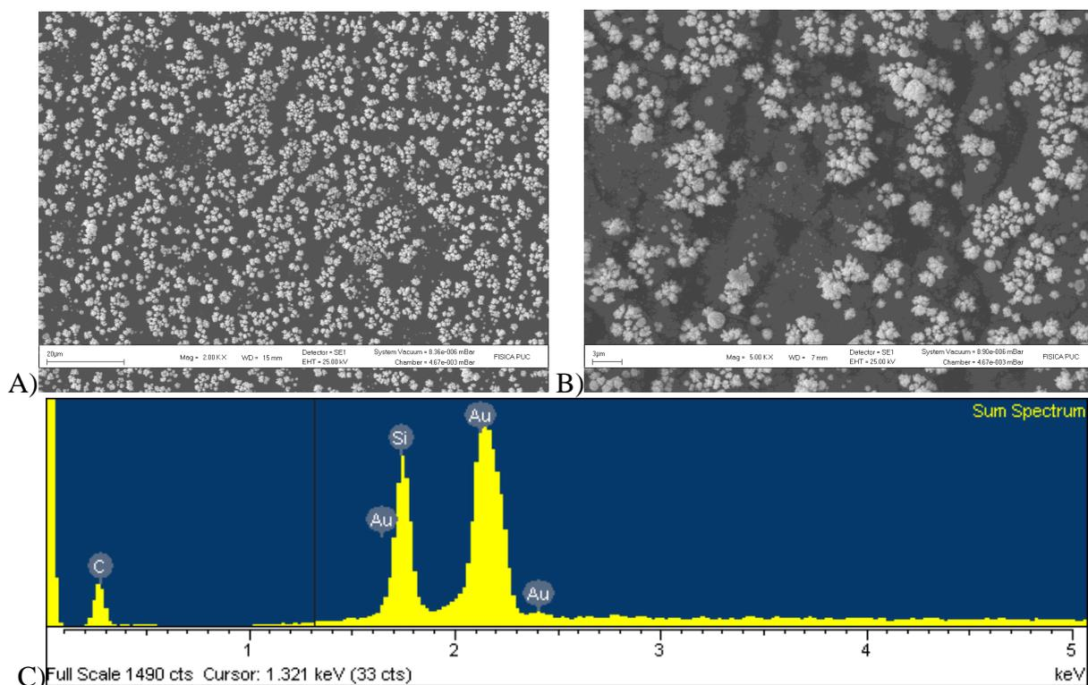
**Figure 2.** A) and 2 B) SEM images of the gold modified BDD electrode at different magnification. C) EDS analysis of the electrode surface obtained for the same sample.
