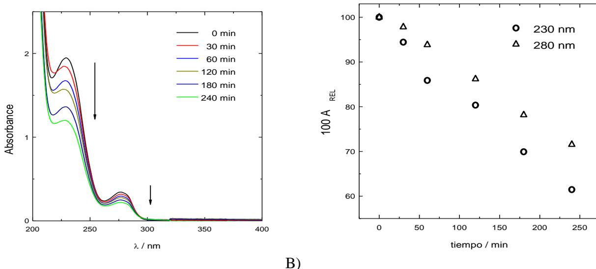
**Figure 4.** A) UV-vis spectra of 100 ppm DEP in 0.05 M Na<sub>2</sub>SO<sub>4</sub> electrolyte during the electrolysis using gold modified BDD anode at 0.03 mA cm<sup>-2</sup>. B) Relative absorbance decay for both absorption band (230 nm open circle, 280 nm open triangle) versus electrolysis time for data of figure 3 A.
