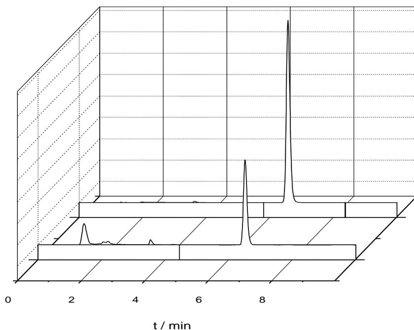
**Figure 6.** HPLC chromatograms obtained during the electrolysis of DEP using BDD anode in  $\text{Na}_2\text{SO}_4$  0.05 M, DEP 100 ppm, at  $t = 0$  min and  $t = 240$  min.
