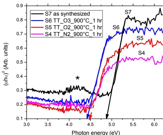
**Figure 5.** UV-Vis spectra of samples obtained as synthesized and with annealed at 900 °C in O<sub>3</sub>, O<sub>2</sub> or N<sub>2</sub>.
