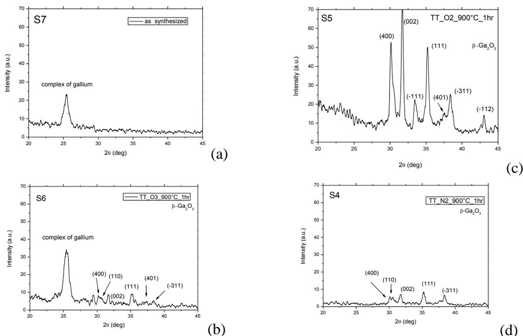
**Figure 1.** XRD patterns of samples obtained as synthesized (a), and with annealed at 900 °C in b) O<sub>3</sub>, c) O<sub>2</sub> and d) N<sub>2</sub>.
