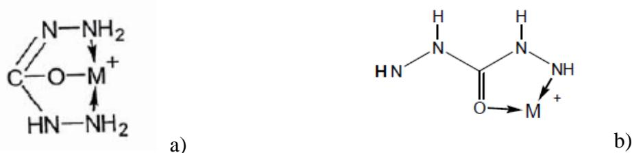
**Figure 3.** Metal-carbohydrazide complexes [18].
