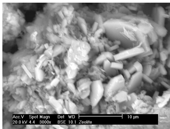
Figure 2. SEM image of morphology structure of clinoptilolite.
