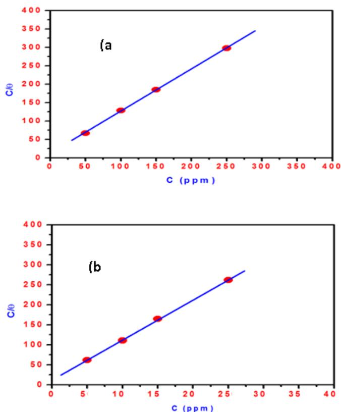
**Figure 8.** Langmuir adsorption plot of steel in 0.1 M HCl solution containing different concentrations of a) poly(AMPS) and b) PAMPS-DEA.
