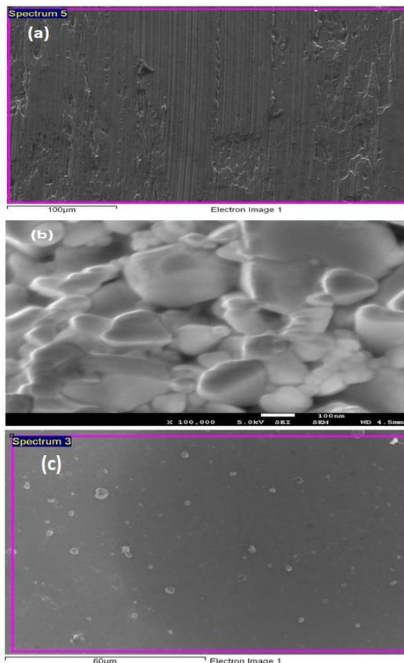
**Figure 9.** SEM micrograph of steel a) polished b) immersed in 1 M HCl (24 hr) and c) after electrochemical measurement treated with 15 ppm of PAMPS-DEA.
