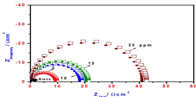
**Figure 7.** Nyquist plots of steel electrode obtained in 1M HCl solution and containing various concentrations of PAMPS-DEA.
