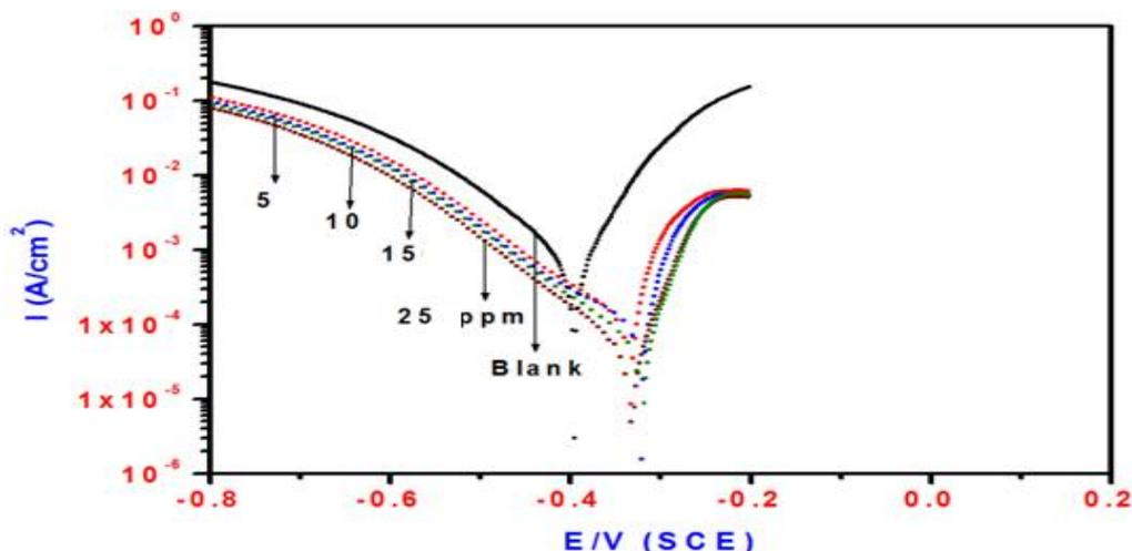
**Figure 5.** Polarization plots of steel electrode obtained in 1M HCl solution and containing various concentrations of PAMPS-DEA.
