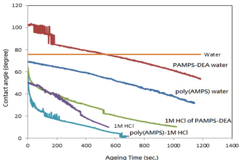
**Figure 3.** Effect of ageing time on contact angle measurements of the 100 ppm and 5 ppm of poly(AMPS) and PAMPS-DEA on the steel surface at 25 °C.
