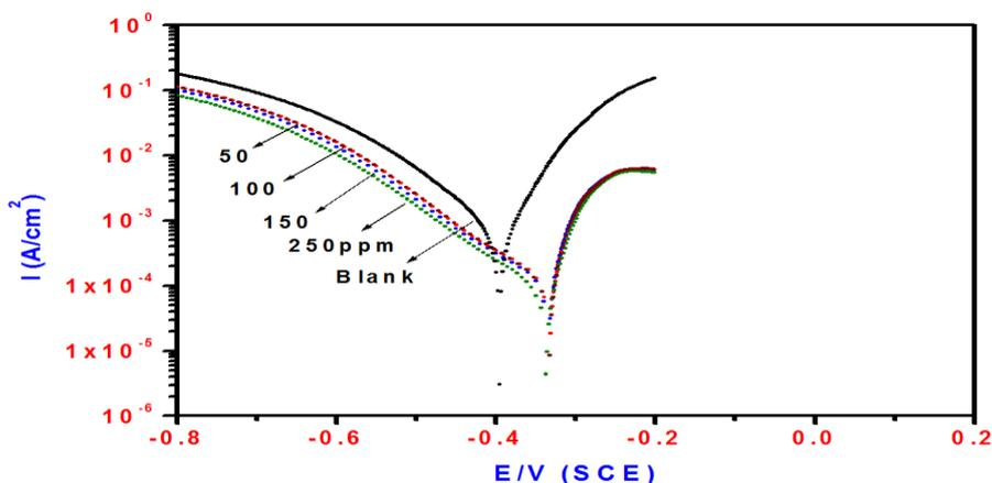
**Figure 4.** Polarization plots of steel electrode obtained in 1M HCl solution and containing various concentrations of poly(AMPS).
