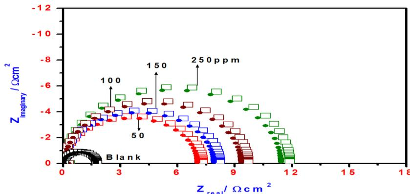
**Figure 6.** Nyquist plots of steel electrode obtained in 1M HCl solution and containing various concentrations of poly(AMPS).
