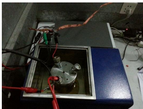
Figure 7. Keithley 6517A electrometer with controllable thermal chamber
