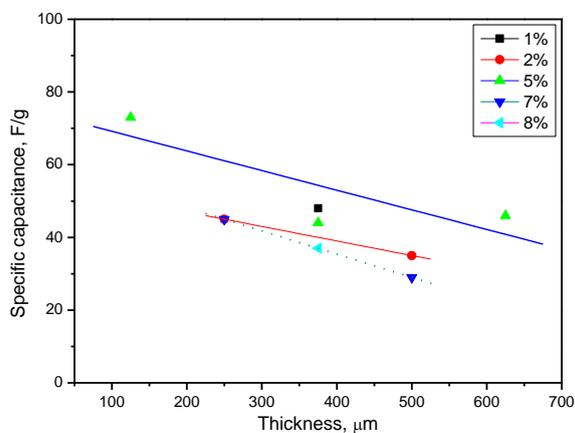
**Figure 6.** The effect of the activated carbon electrode layer thickness on the specific capacitance of EDLCs.
