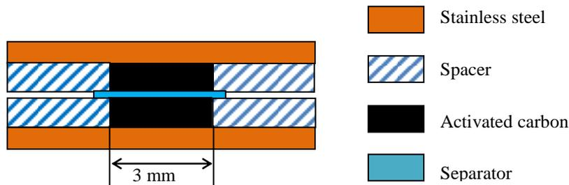
**Figure 1.** Schematic diagram of the strip supercapacitor.
