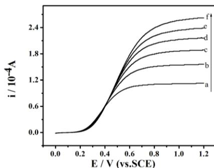
**Figure 4.** Rotating-disk electrode voltammograms of LDHs / SWNTs / PPO coated on GCE ( $d = 5 \text{ mm}$ ) in the presence of 2 mM hydroquinone in 0.05 M PBS (pH 6.0): (a) 200, (b) 400, (c) 600, (d) 800, (e) 1000, and (f) 1200 rpm/min. Scan rate at  $10 \text{ mV s}^{-1}$
