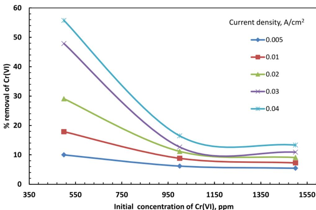
**Figure 4.** Effect of the initial Cr(VI) concentration on the removal of chromium ions at different current densities (NaCl conc. = 3.5 wt%; pH = 2.5; smooth anode).
