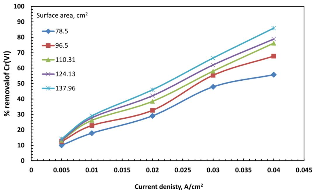
**Figure 7.** Effect of current density on the percentage of Cr(VI) removed at different surface areas (initial concentration of Cr(VI) = 500 ppm; NaCl conc. = 3.5 wt%; pH = 2.5).
