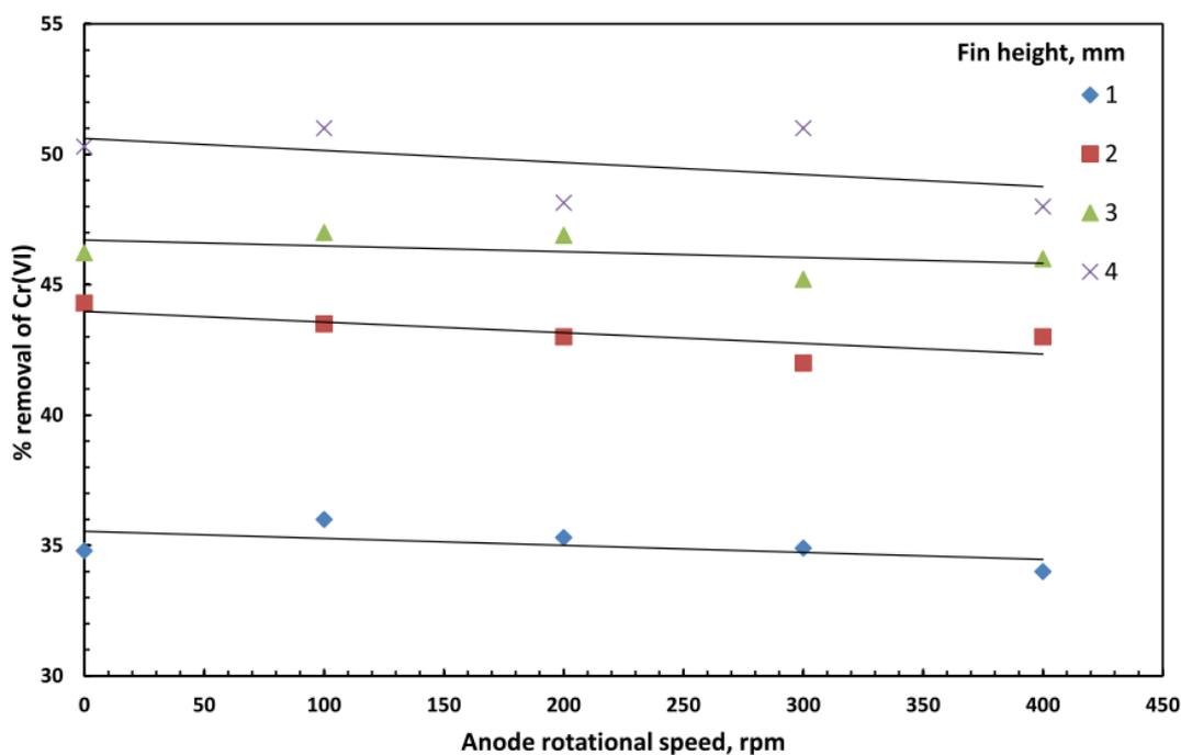
**Figure 3.** Effect of anode rotational speed on the removal of Cr(VI) at different degrees of roughness (initial concentration of Cr(VI) = 500 ppm; c.d =  $0.01 \text{ A cm}^{-2}$ ; NaCl conc. = 3.5 wt%; pH = 2.5; contact time = 15 min).
