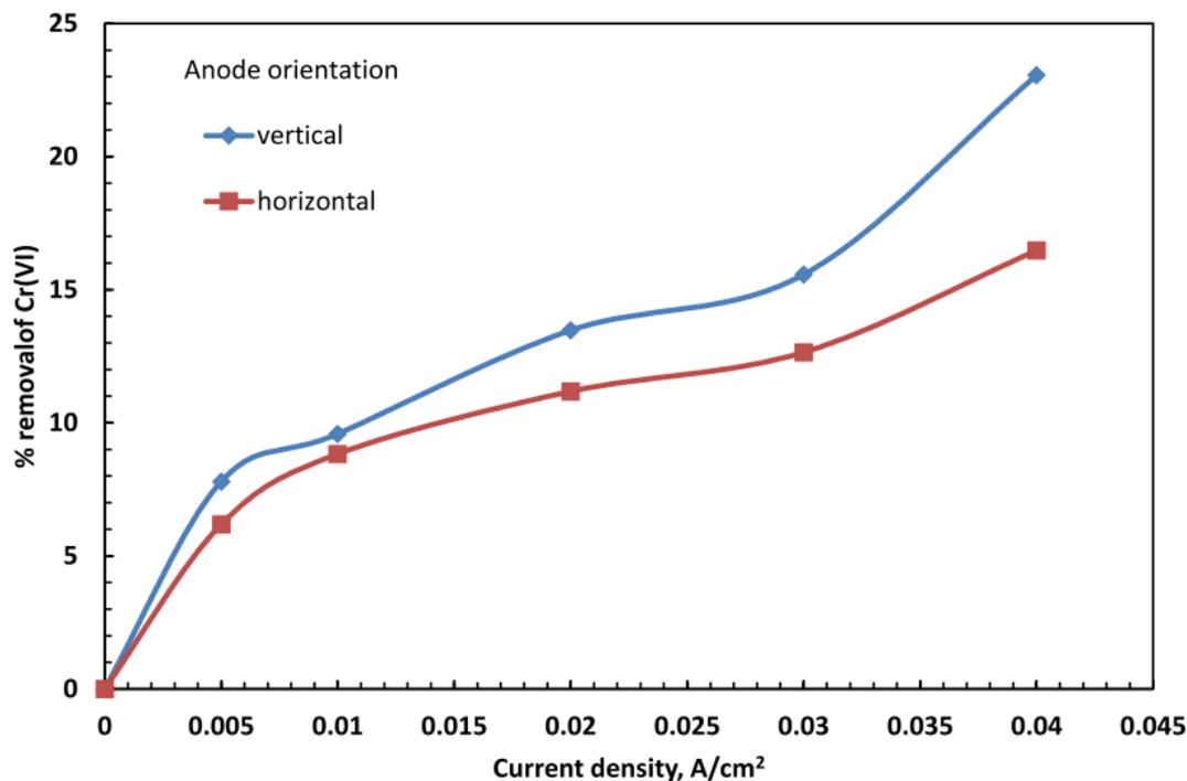
**Figure 5.** Effect of current density on the percentage of Cr(VI) removed using vertical and horizontal anode orientations (initial concentration of Cr(VI)= 1000 ppm; smooth anode; NaCl conc. = 3.5 wt%; pH = 2.5).
