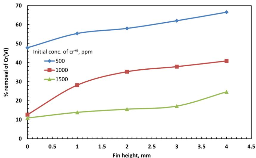
**Figure 6.** Effect of anode roughness on the percentage of Cr(VI) removed at different initial concentrations of Cr(VI) ions (NaCl conc. = 3.5 wt%; pH = 2.5; current density = 0.03 A cm<sup>-2</sup>).
