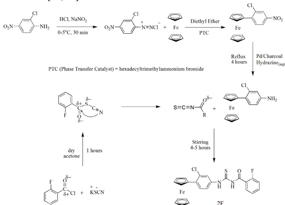
**Scheme 1.** Schematic representation for the synthesis 1-(2-florobenzoyl)-3-(2-chloro, 4-ferrocenylphenyl) thiourea (2F)
