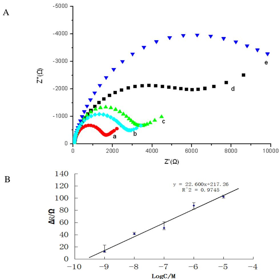
**Figure 3.** (A) EIS of different concentrations of TET: impedance change with  $10^{-9}$  to  $10^{-5}$  g/mL TET(a) 1ng/mL ; (b) 10ng/mL ; (c) 100ng/mL ; (d) 1μg/mL ; (e) 10μg/mL (B) Detection standard curve of aptasensor to tetracycline
