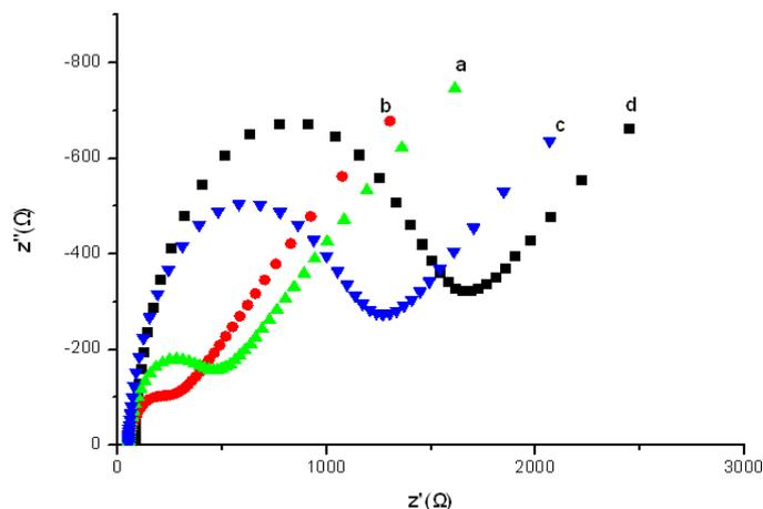
**Figure 2.** EIS of aptasensor (a) bare electrode (b) ionic liquid-Fe<sub>3</sub>O<sub>4</sub> (c) TET aptamer (d)TET; under testing solution of 5 mM [Fe(CN)<sub>6</sub>]<sup>3-/4-</sup> and 0.1 mol/L KCl( pH 7.0 PBS)
