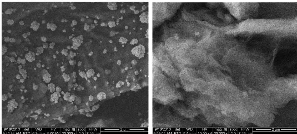
**Figure 1.** SEM photos of PB-GR (A), and CS-PB-GR composite (B).
