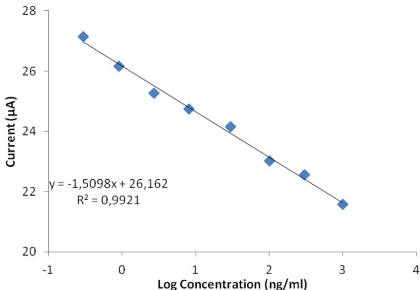
**Figure 5.** The calibration curve of melamine standard solution.
