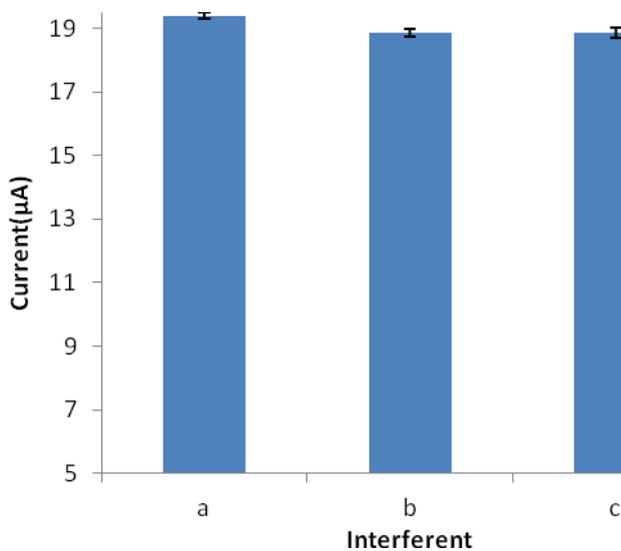
**Figure 6.** The peak current of the proposed immunosensor to the interference. (a) 100 ng/mL melamine; (b) 100ng/mL melamine + 100 ng/mL ammelide and; (c) 100 ng/mL melamine + 100 ng/mL ammeline.
