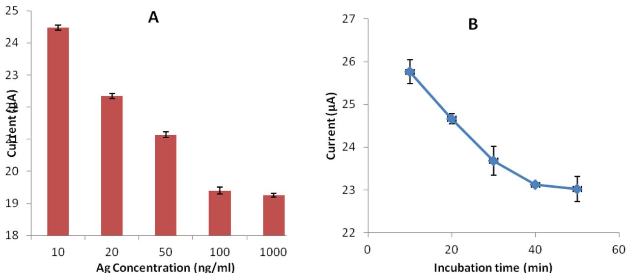
**Figure 3.** Optimization of experimental parameters. (A) the effect of immobilized antigen concentration; (B) the effect of the incubation time.
