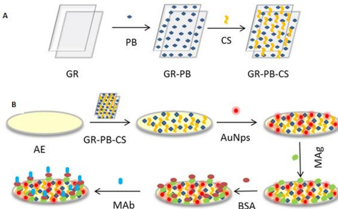
**Scheme 1.** Schematic illustration for the preparation of the immunosensor. (A) CS-PB-GR nanocomposite; (B) illustration of the preparation process of the modified electrode.
