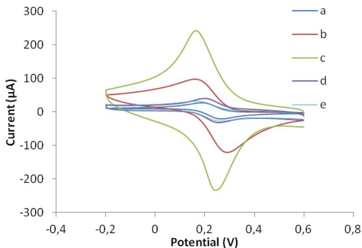
**Figure 2.** Cvs of the electrodes at different stages. (a)Bare AE, (b)CS-PB-GR/AE, (c)AuNps/CS-PB-GR/AE, (d)MAg/ AuNps/ CS-PB-GR/AE, (e)MAb/ MAg/ AuNps/ CS-PB-GR/AE at a scan rate of 50 mV/s and in 2.0 mM  $K_3[Fe(CN)_6]/K_4[Fe(CN)_6]$  (1:1) solution, respectively.
