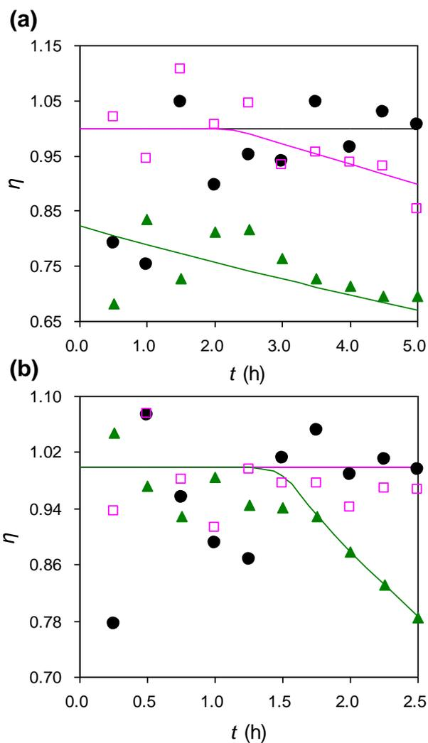
**Figure 3.** The variation of average current efficiency during electrochemical oxidation at applied current densities of 200 A/m<sup>2</sup> (●), 300 A/m<sup>2</sup> (□) and 400 A/m<sup>2</sup> (▲) in the absence (a) and in the presence (b) of GAC under flow rate of 1 L/h at a constant temperature of 25 °C. The solid curves represent the model prediction using Eq. (19).
