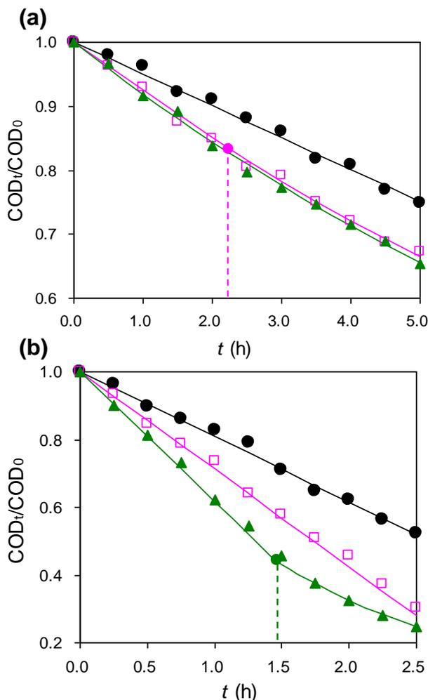
**Figure 2.** Effect of the applied current density (● 200 A/m<sup>2</sup>; □ 300 A/m<sup>2</sup>; ▲ 400 A/m<sup>2</sup>) on the variation of  $COD_t/COD_0$  in the absence (a) and in the presence (b) of GAC under flow rate of 1.0 L/h at a constant temperature of 25 °C. The solid curves represent the model prediction using Eqs. (11) and (12).
