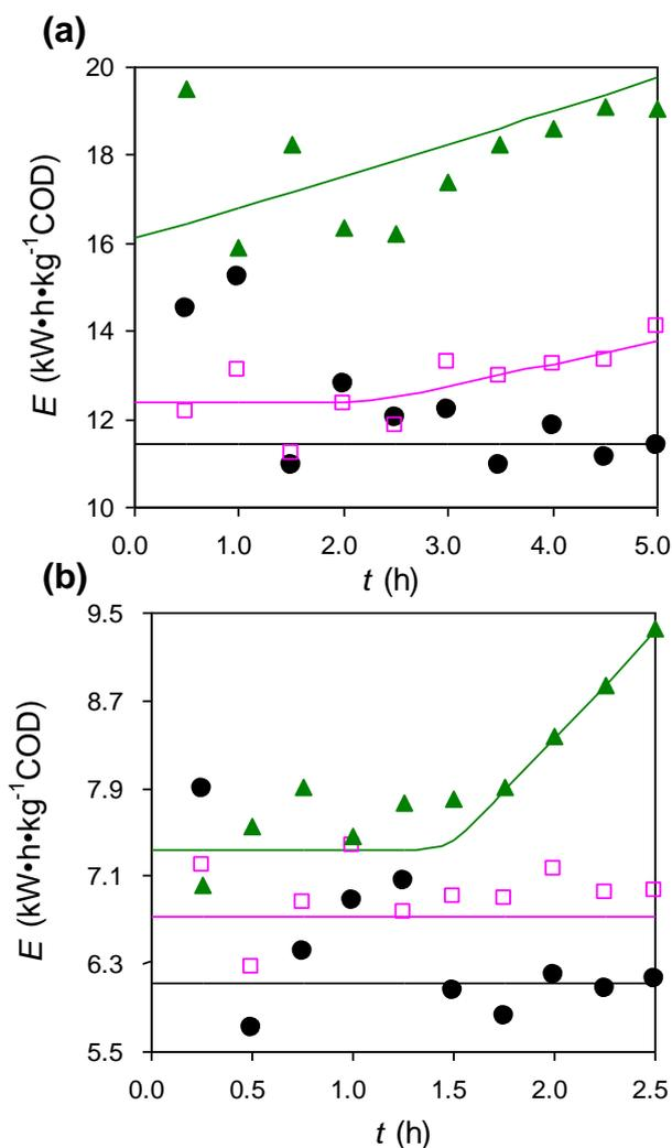
**Figure 4.** The variation of power consumption during electrochemical oxidation at applied current densities of 200 A/m<sup>2</sup> (●), 300 A/m<sup>2</sup> (□) and 400 A/m<sup>2</sup> (▲) in the absence (a) and in the presence (b) of GAC under flow rate of 1 L/h at a constant temperature of 25 °C. The solid curves represent the model prediction using Eqs. (22) and (23).
