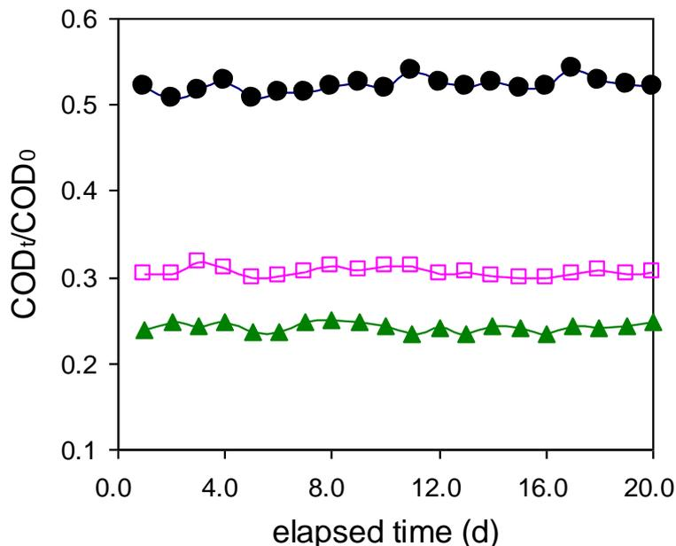
**Figure 1.** The variation of effluent COD with 20 days continuous operation of PBEC under applied current density (● 200 A/m<sup>2</sup>; □ 300 A/m<sup>2</sup>; ▲ 400 A/m<sup>2</sup>) at a constant temperature of 25 °C.
