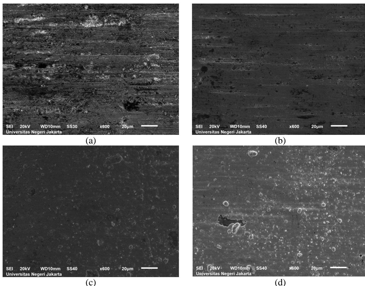
**Figure 2.** SEM analysis on surface morphology of Ni-TiAlN composite film at TiN and AlN particle concentration of (a) 2 gr/lit, (b) 4 gr/lit, (c) 6 gr/lit and (d) 8 gr/lit.
