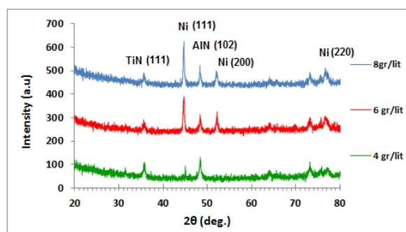
**Figure 4.** XRD analysis on structure of Ni-TiAlN composite film at TiN and AlN particle concentration of (a) 4 gr/lit, (b) 6 gr/lit and (c) 8 gr/lit.
