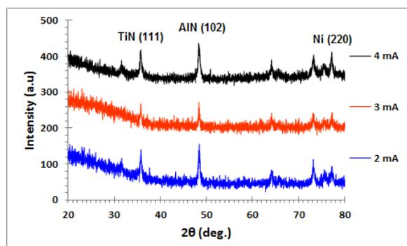
**Figure 3.** XRD analysis on structure of Ni-TiAlN composite film at electrodeposition current of (a) 2 mA, (b) 3 mA and (c) 4 mA.
