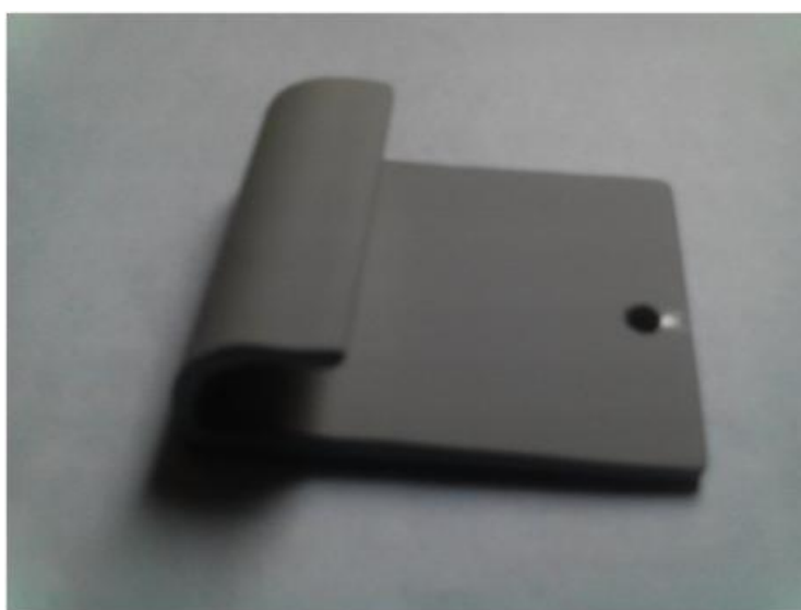
Figure 1. AA 6063 by micro-arc oxidation treatment
