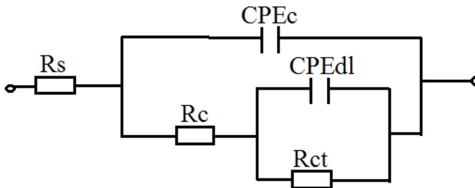
**Figure 5.** Equivalent circuit for HRB500 reinforcement in SCP solutions
