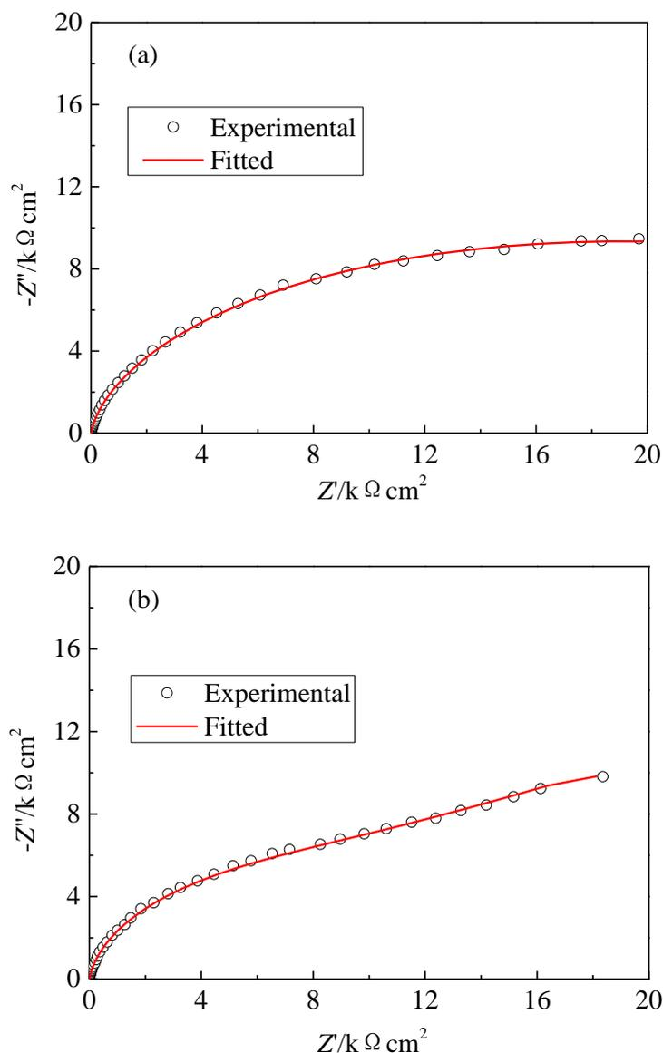
**Figure 6.** Comparison of the experimental and the fitted curves for HRBF500 reinforcement in SCP solutions with an  $[\text{NO}_2^-]/[\text{Cl}^-]$  ratio of 0.2: (a) 0.171 mol/L and (b) 0.598 mol/L NaCl
