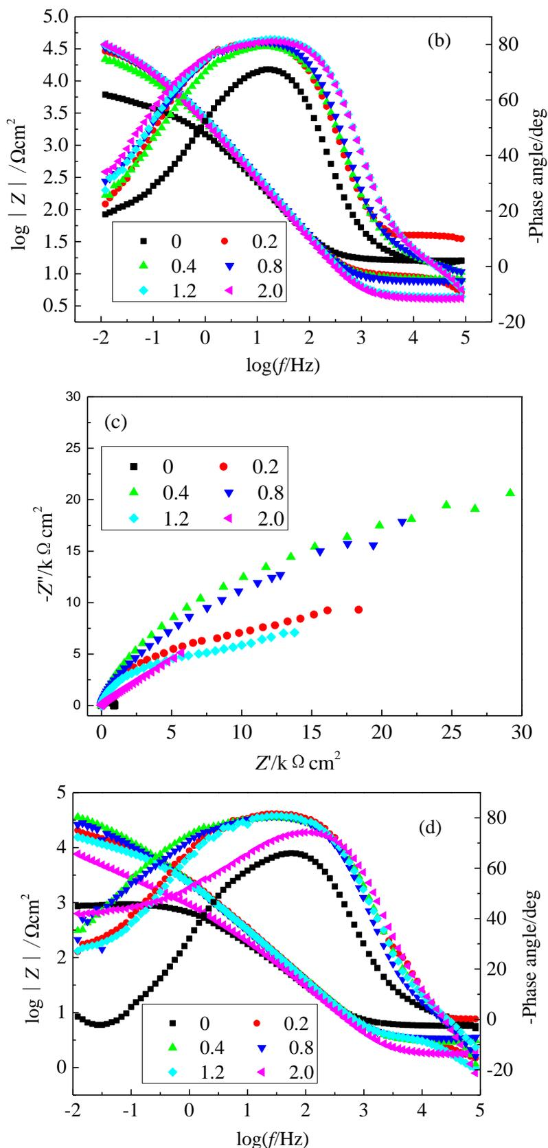
**Figure 4.** Effect of  $[\text{NO}_2^-]/[\text{Cl}^-]$  ratio on EIS diagrams for HRBF500 reinforcement in SCP solutions: (a) Nyquist diagrams and (b) Bode diagrams with 0.171 mol/L NaCl; (c) Nyquist diagrams and (d) Bode diagrams with 0.598 mol/L NaCl
