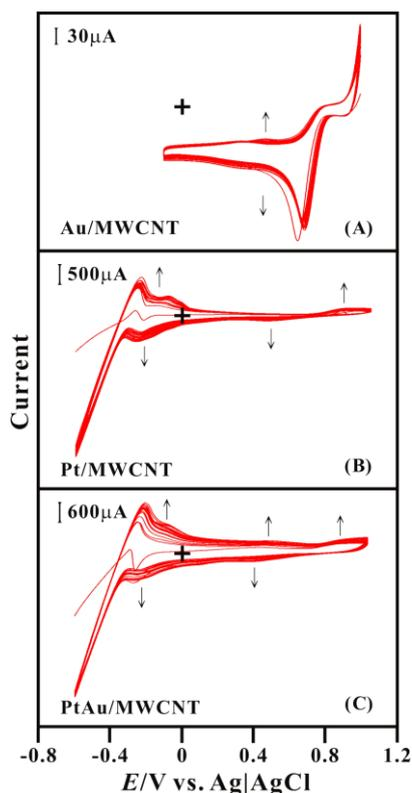
**Figure 1.** Consecutive cyclic voltammograms (20 cycles) of MWCNT modified electrode in  $0.5 \text{ M H}_2\text{SO}_4$  solution containing (A)  $2 \text{ mM H}_2\text{PtCl}_6$ , (B)  $1.8 \text{ mM HAuCl}_4$  and (C)  $2 \text{ mM H}_2\text{PtCl}_6 + 1.8 \text{ mM HAuCl}_4$ , respectively. Scan rate =  $0.1 \text{ Vs}^{-1}$ .
