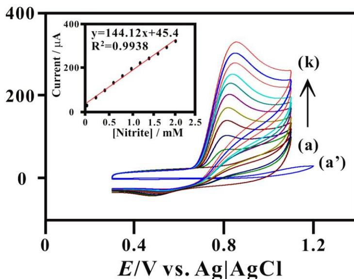
**Figure 4.** Cyclic voltammograms of MWCNT/PtAu modified electrode in PBS containing nitrite ((a) 0, (b) 0.2 mM, (c) 0.4 mM, (d) 0.6 mM, and (e) 0.8 mM, (f) 1.0 mM, (g) 1.2 mM, (h) 1.4 mM, (i) 1.6 mM, (j) 1.8 mM, (k) 2 mM). Scan rate = 0.1  $\text{Vs}^{-1}$ . Inset: the plot of the anodic peak current vs. [nitrite].
