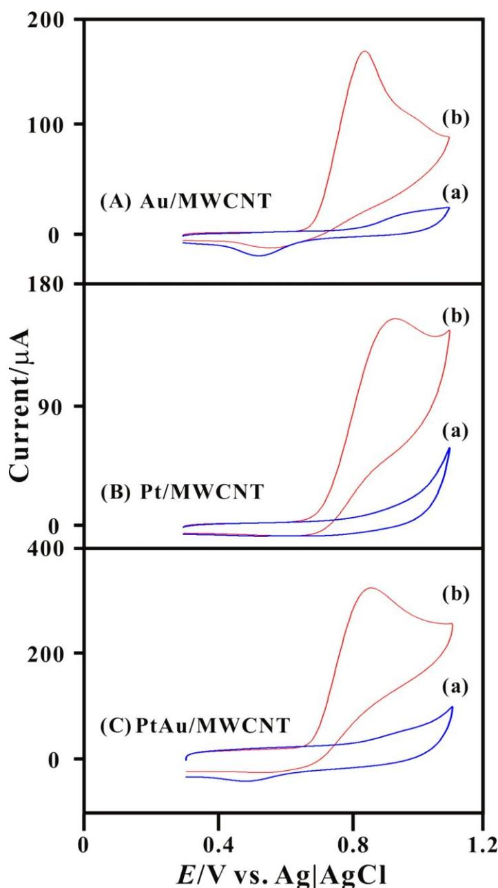
**Figure 3.** Cyclic voltammograms of (A) MWCNT/Pt, (B) MWCNT/Au, (C) MWCNT/PtAu modified electrodes in the (a) absence and (b) presence of 2 mM nitrite (pH 7 PBS). Scan rate = 0.1 Vs<sup>-1</sup>.
