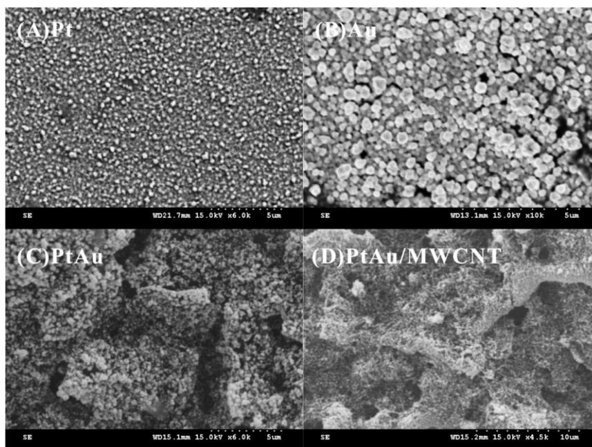
**Figure 2.** (A) SEM images of (A) Pt, (B) Au, (C) Pt/Au and (D) MWCNT/PtAu composite modified electrodes.
