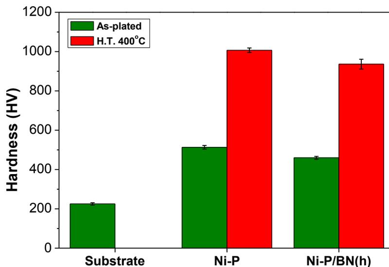
**Figure 4.** The effect of heat treatment on the hardness of iron substrate, Ni–P and Ni–P/BN(h) composite coatings.
