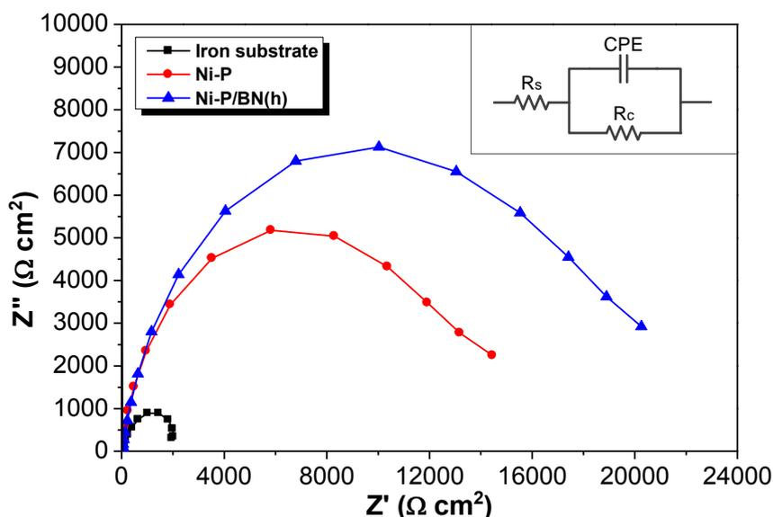
**Figure 6.** Nyquist plots of iron substrate, Ni–P and Ni–P/BN(h) composite coatings in the 3.5 wt.% NaCl solution.
