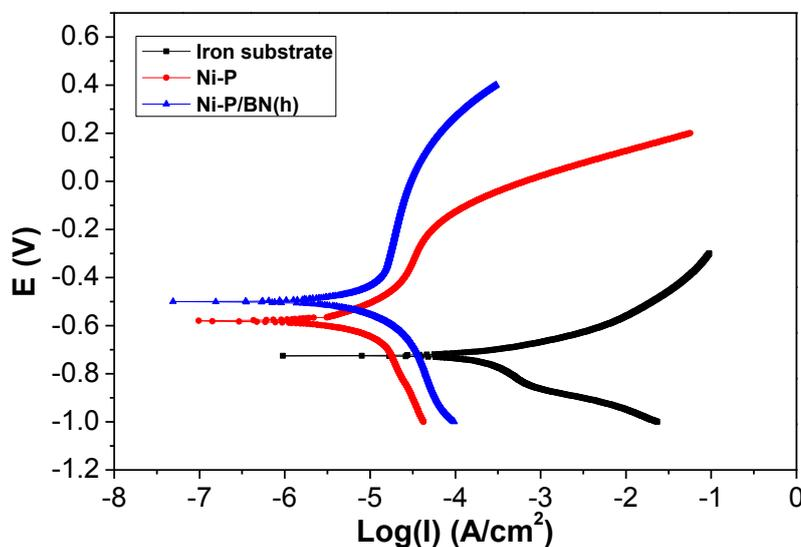
**Figure 5.** Potentiodynamic polarization curves of steel substrate, Ni-P coatings and Ni-P/BN(h) composite coatings in 3.5wt.% NaCl solution.
