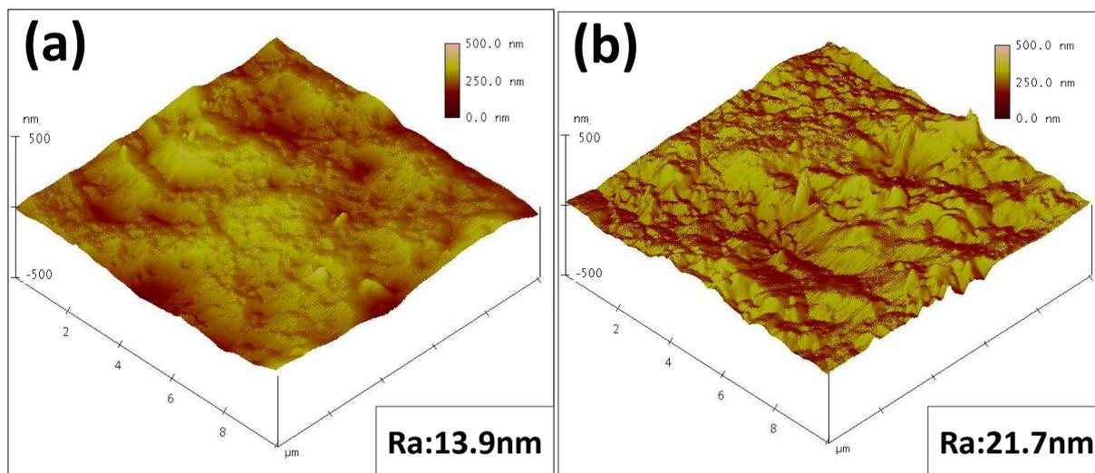
**Figure 2.** AFM images of the surface morphology of (a) Ni–P and Ni–P/BN(h) composite coatings.
