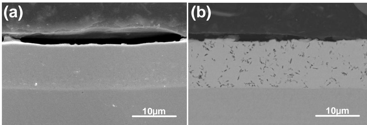
**Figure 1.** SEM images of the cross section of (a) Ni–P and Ni–P/BN(h) composite coatings.
