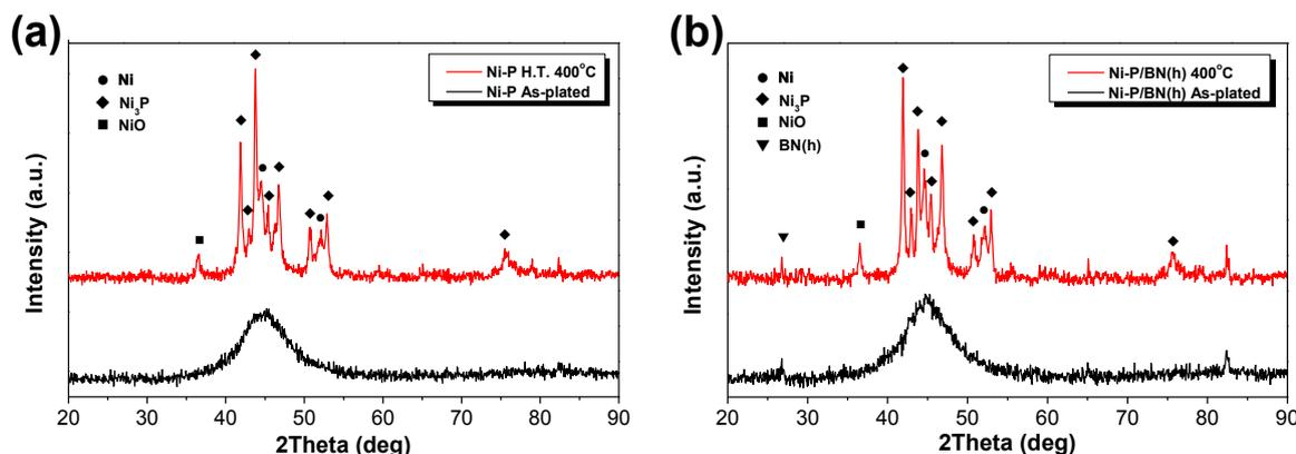
**Figure 3.** The XRD patterns of (a) Ni–P and (b) Ni–P/BN(h) composite coatings.
