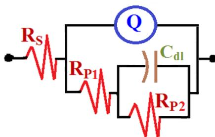
Figure 3. The equivalent circuit model that was used to fit the EIS data.
