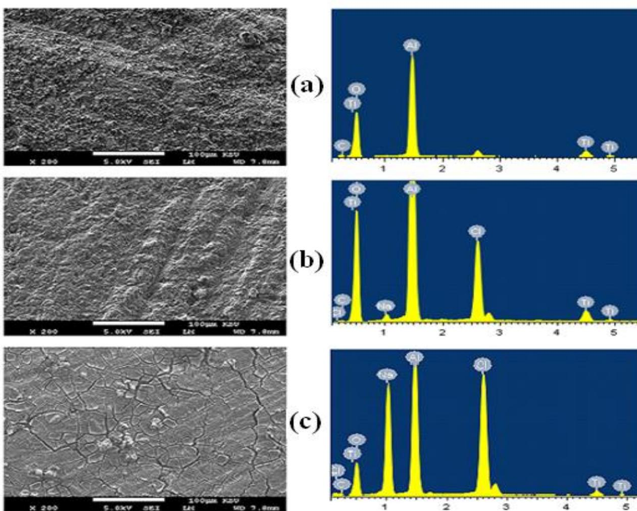
**Figure 8.** SEM images and EDX profile analyses obtained after 24 h immersion in 3.5% NaCl solutions for the surface of (a) Al-15%TiC, (b) Al-25%TiC and (c) Al-35%TiC composites, respectively before stepping their potential to  $-100$  mV(Ag/AgCl) for 1.0 h.
