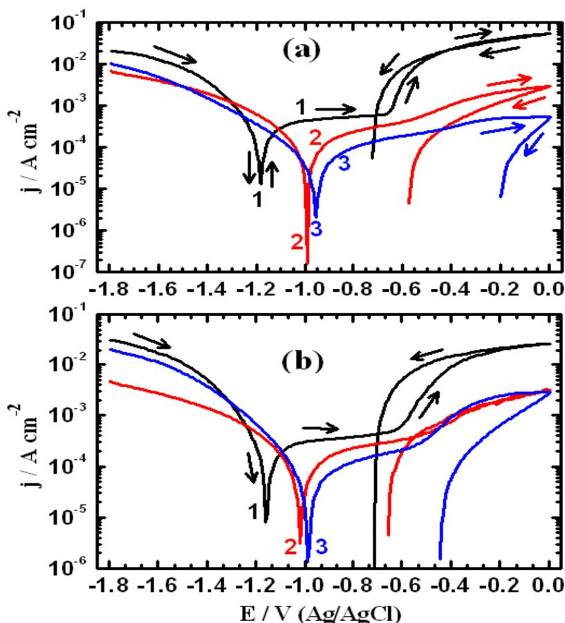
**Figure 6.** CPP curves of (1) Al-15%TiC, (2) Al-25%TiC and (3) Al-35%TiC composites after (a) 1 h and (b) 24 h immersions in 3.5% NaCl solutions.
