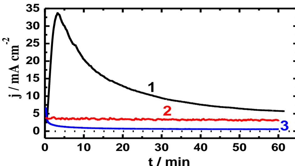
**Figure 7.** CCT curves recorded at  $-100$  mV/AgCl for (1) Al-15%TiC, (2) Al-25%TiC and (3) Al-35%TiC composites after 24 h immersion in 3.5% NaCl solutions.
