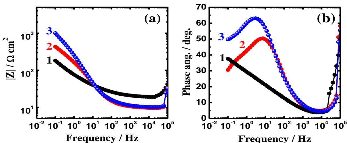
**Figure 5.** Bode (a) impedance and (b) phase angle plots of (1) Al-15%TiC, (2) Al-25%TiC and (3) Al-35%TiC composites after 24 h immersion in 3.5% NaCl solutions.
