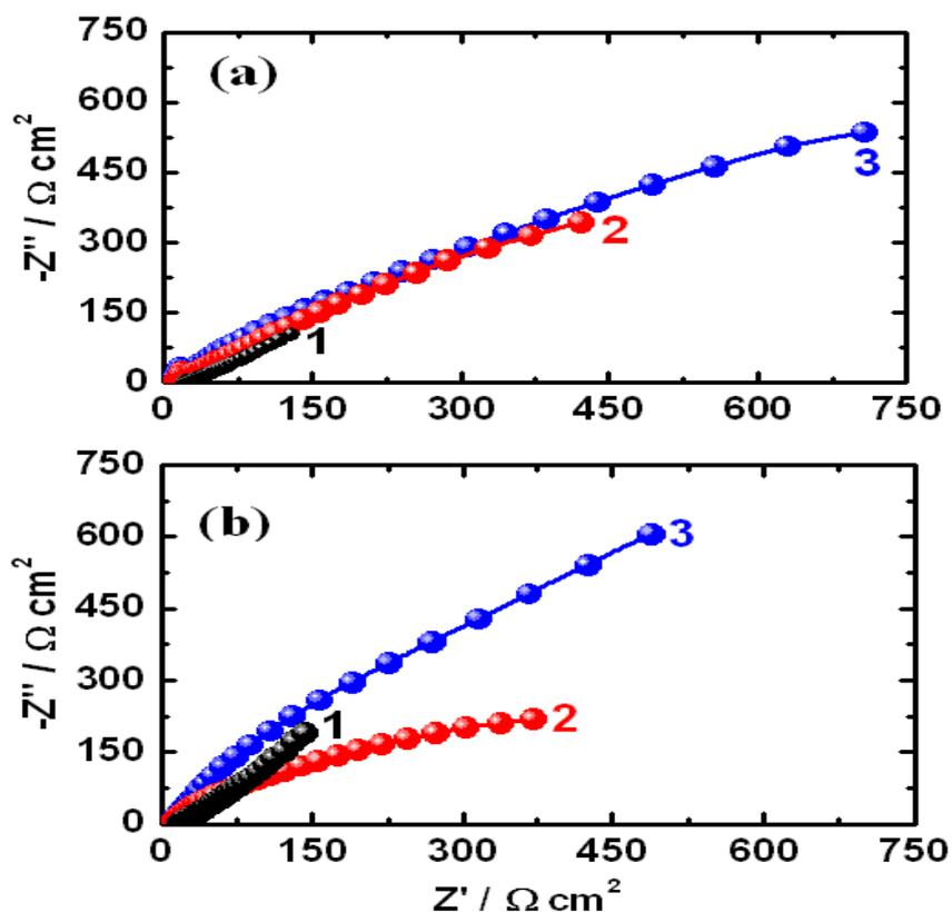
**Figure 2.** Nyquist plots of (1) Al-15%TiC, (2) Al-25%TiC and (3) Al-35%TiC composites after (a) 1.0 h and (b) 24 h immersions in 3.5% NaCl solutions, respectively.
