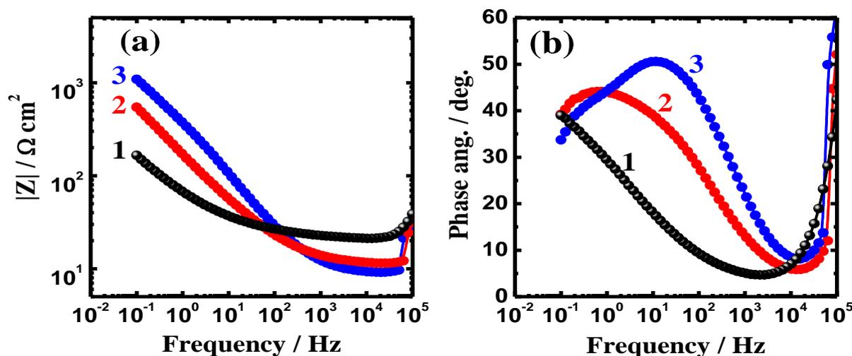
**Figure 4.** Bode (a) impedance and (b) phase angle plots of (1) Al-15% TiC, (2) Al-25% TiC and (3) Al-35% TiC composites after 1.0 h immersion in 3.5% NaCl solutions
