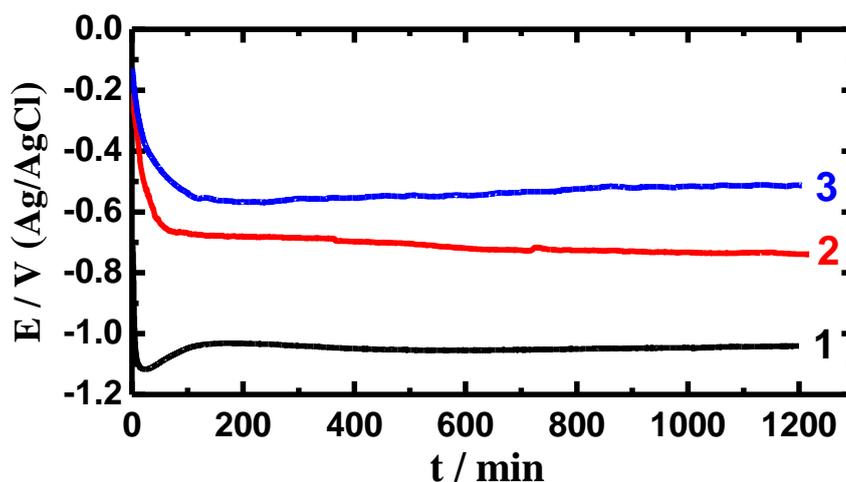
**Figure 1.** OCP curves obtained for (1) Al-15%TiC, (2) Al-25%TiC and (3) Al-35%TiC composites in 3.5% NaCl solutions.
