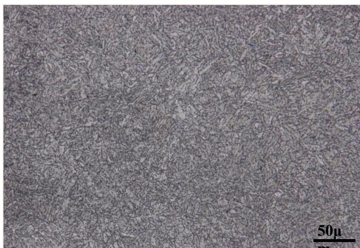
Figure 2. Microstructure of TP95S tube steel.
