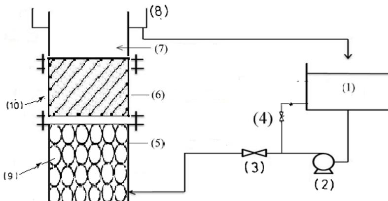
**Figure 1 .** Experimental setup. (1) Plastic storage tank , (2) Plastic centrifugal pump , (3) Control valve , (4) bypass plastic valve , (5) Inlet section , (6) Working section , (7) outlet section , (8) Overflow weir , (9) Glass spheres , (10) Copper Lessing rings or copper Raschig rings
