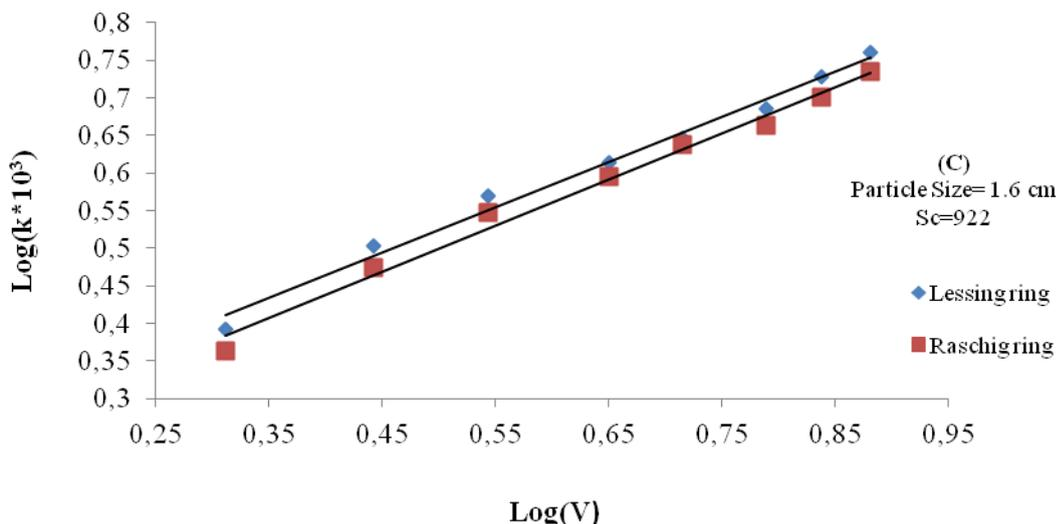
**Figure 6 .** Comparison between the mass transfer behaviour of beds of Lessing rings and beds of Raschig rings
