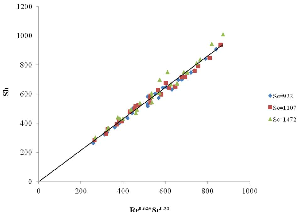
**Figure 4 .** Overall mass transfer correlation at a fixed bed of Lessing rings
