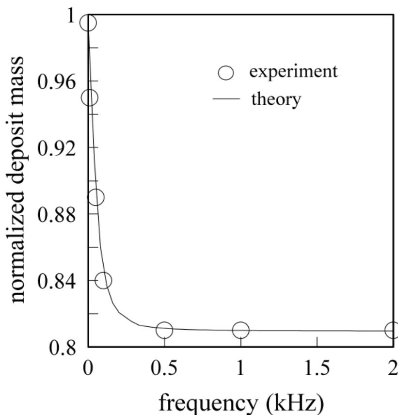
**Figure 3.** A plot of the normalized deposit mass vs. the low frequency for the Ni film at a solution temperature of 298 K. The open circles and solid curve show the measured deposit mass and the curve best fitted to the measured deposit mass using  $R_l=18.5 \Omega$ ,  $R_c=11 \Omega$ ,  $R_{ch}/r=5 \times 10^{-3}$ , and  $C_s=95 \mu\text{F}$ .
