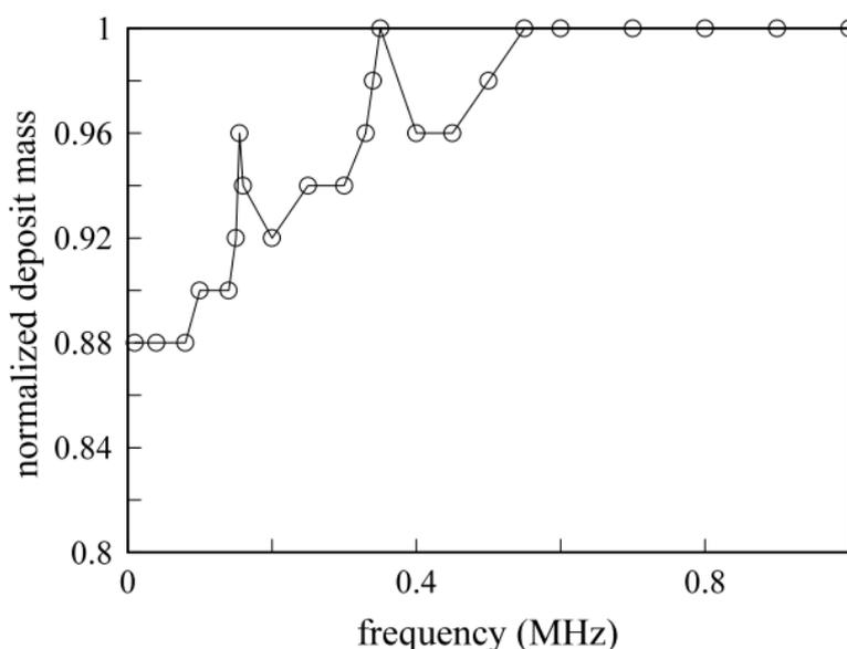
**Figure 5.** A plot of the normalized deposit mass vs. frequency for the Ni film at a solution temperature of 318 K. The solid line is drawn to help an eye.
