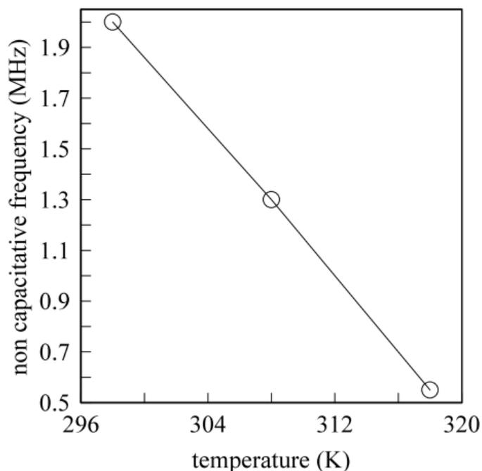
**Figure 6.** A plot of the non capacitive frequency vs. solution temperature.
