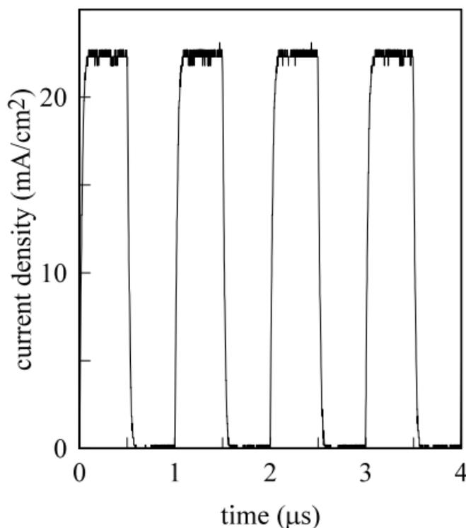
**Figure 1.** Typical rectangular current pulse having an amplitude of  $22.3 \text{ mA/cm}^2$  and a frequency of 1.0 MHz. The rectangular current pulse was determined by the voltage drop across the resistor measured with the digital storage oscilloscope.
