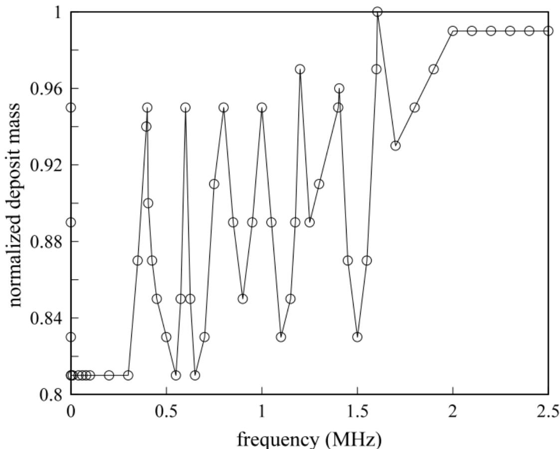
**Figure 2.** A plot of the normalized deposit mass vs. frequency for the Ni film at a solution temperature of 298 K. The solid line is drawn to help an eye.
