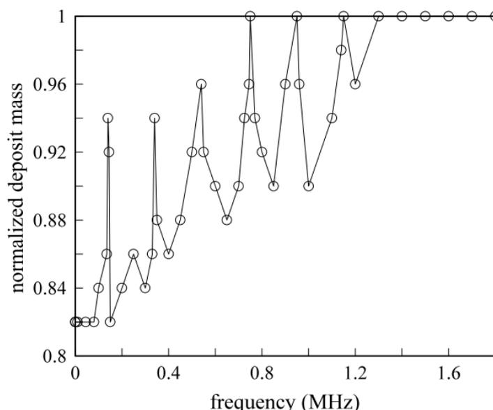
**Figure 4.** A plot of the normalized deposit mass vs. frequency for the Ni film at a solution temperature of 308 K. The solid line is drawn to help an eye.
