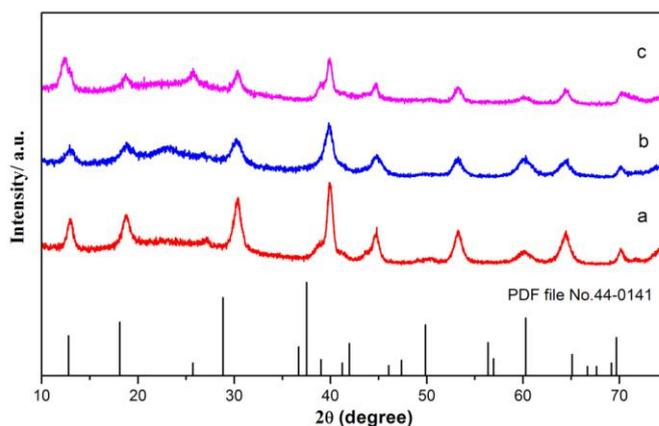
**Figure 2.** The XRD patterns of  $\text{MnO}_2$  materials. (a) (b) (c) are consistent with that listed in Table 1.
