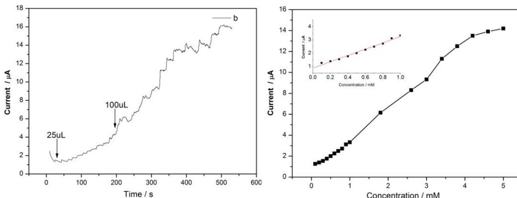
**Figure 8.** Current-time response of sample *b* modified electrode upon addition of H<sub>2</sub>O<sub>2</sub> at 0.8 V. Cell volume: 20 mL; firstly added H<sub>2</sub>O<sub>2</sub> solution 25µL(10<sup>th</sup>) (0.08mol L<sup>-1</sup>); then added H<sub>2</sub>O<sub>2</sub> solution 100µL(10<sup>th</sup>) (0.08mol L<sup>-1</sup>).
