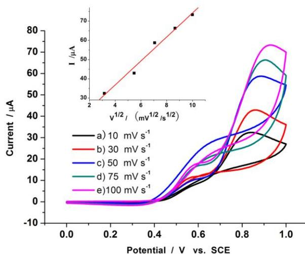
**Figure 4.** Cyclic voltammetric curves for sample a (urchin-like MnO<sub>2</sub> microsphere modified electrode) of 5 mmol L<sup>-1</sup> H<sub>2</sub>O<sub>2</sub> in 0.2 mol L<sup>-1</sup> PBS (pH=7.0) at different scan rates: (a) 10, (b) 30, (d) 50, (e) 75, (f) 100 (mV s<sup>-1</sup>). Inset: The relation between anodic peak currents of H<sub>2</sub>O<sub>2</sub> versus the square root of scan rate.
