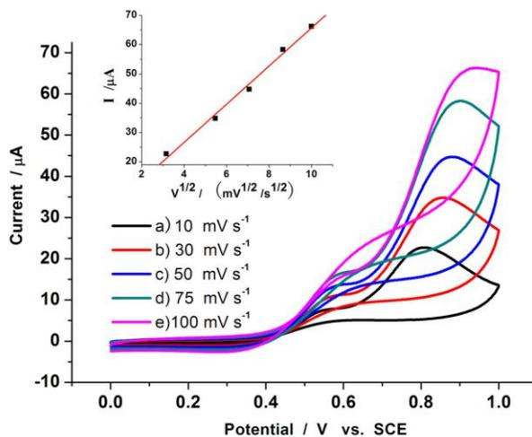
**Figure 5.** Cyclic voltammetric curves for sample b (caddice-clew like  $\text{MnO}_2$  micromaterials modified electrode) of  $5\text{mmol L}^{-1}$   $\text{H}_2\text{O}_2$  in  $0.2\text{ mol L}^{-1}$  PBS (pH=7.0) at different scan rates: (a) 10, (b) 30, (d) 50, (e) 75, (f) 100 ( $\text{mV s}^{-1}$ ). Inset: The relation between anodic peak currents of  $\text{H}_2\text{O}_2$  versus the square root of scan rate.
