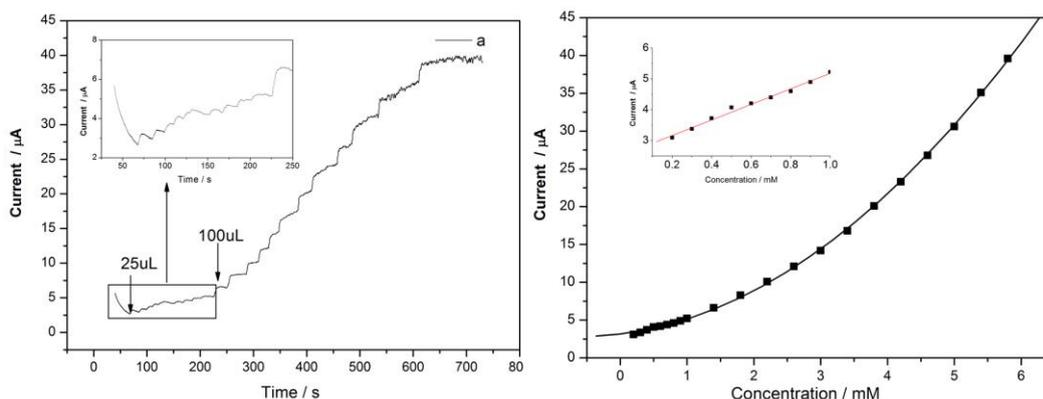
**Figure 7.** Current-time response of sample *a* modified electrode upon addition of H<sub>2</sub>O<sub>2</sub> at 0.8 V. Cell volume: 20 mL; firstly added H<sub>2</sub>O<sub>2</sub> solution 25µL(10<sup>th</sup>) (0.08mol L<sup>-1</sup>); then added H<sub>2</sub>O<sub>2</sub> solution 100µL(10<sup>th</sup>) (0.08mol L<sup>-1</sup>).
