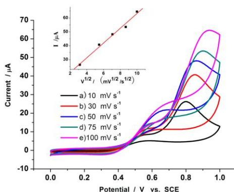
**Figure 6.** Cyclic voltammetric curves for sample c ( $\text{MnO}_2$  nanoflowers modified electrode) of  $5\text{mmol L}^{-1}$   $\text{H}_2\text{O}_2$  in  $0.2\text{ mol L}^{-1}$  PBS (pH=7.0) at different scan rates: (a) 10, (b) 30, (d) 50, (e) 75, (f) 100 ( $\text{mV s}^{-1}$ ). Inset: The relation between anodic peak currents of  $\text{H}_2\text{O}_2$  versus the square root of scan rate.
