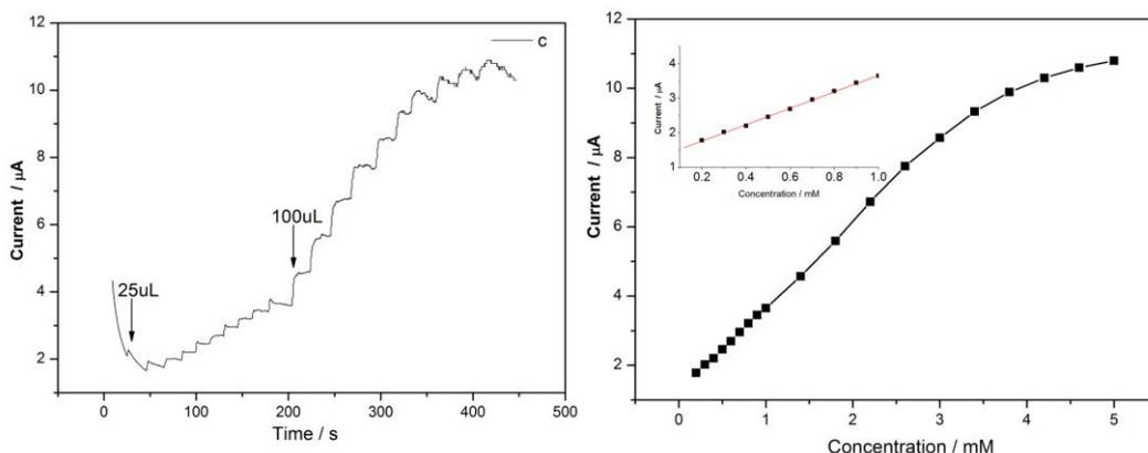
**Figure 9.** Current-time response of sample *c* modified electrode upon addition of  $\text{H}_2\text{O}_2$  at 0.8 V. Cell volume: 20 mL; firstly added  $\text{H}_2\text{O}_2$  solution 25  $\mu\text{L}$  ( $10^{\text{th}}$ ) ( $0.08 \text{ mol L}^{-1}$ ); then added  $\text{H}_2\text{O}_2$  solution 100  $\mu\text{L}$  ( $10^{\text{th}}$ ) ( $0.08 \text{ mol L}^{-1}$ ).
