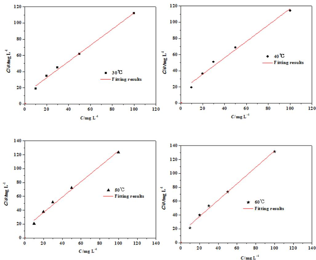
**Figure 6.** Langmuir’s adsorption plots for carbon steel in 0.25 M H<sub>2</sub>SO<sub>4</sub> solution containing various concentrations of HACC at different temperatures (30-60°C).
