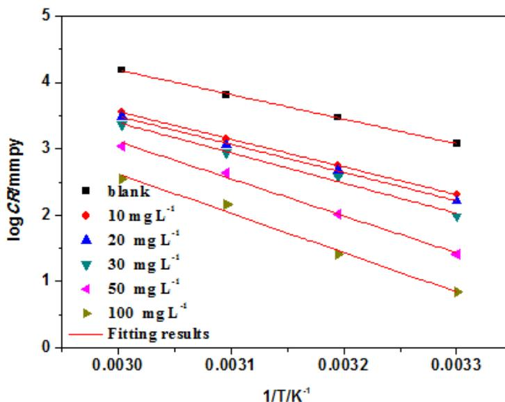
**Figure 7.** Arrhenius plots for carbon steel in 0.25 M H<sub>2</sub>SO<sub>4</sub> solution without and with different concentrations of HACC. **Table 4.** The calculated thermodynamic parameters of adsorption from weight loss measurements.
