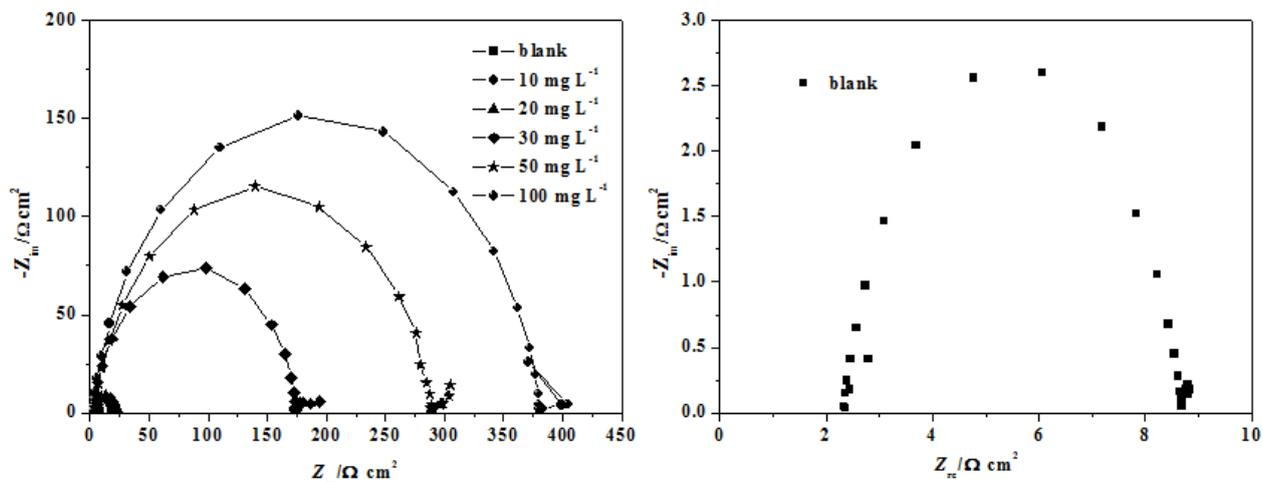
**Figure 4.** Nyquist plots of carbon steel electrode in 0.25 M H<sub>2</sub>SO<sub>4</sub> solution without and with different concentrations of HACC at 30°C.
