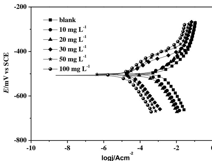
**Figure 3.** Anodic and cathodic curves of carbon steel electrode in 0.25 M H<sub>2</sub>SO<sub>4</sub> solution without and with HACC at 30°C.
