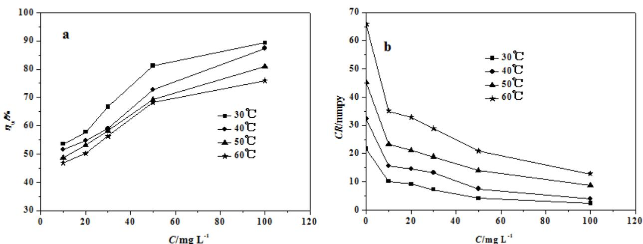
**Figure 2.** Plots of inhibition efficiency ( $\eta_w\%$ ) (a) and corrosion rate ( $CR$ ) (b) for carbon steel in uninhibited and inhibited 0.25 M H<sub>2</sub>SO<sub>4</sub> solutions at 30-60°C.
