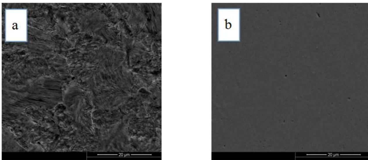
**Figure 8.** SEM images of carbon steel in 0.25 M H<sub>2</sub>SO<sub>4</sub> solution (a) blank; (b) with 100 mg L<sup>-1</sup> of HACC.
