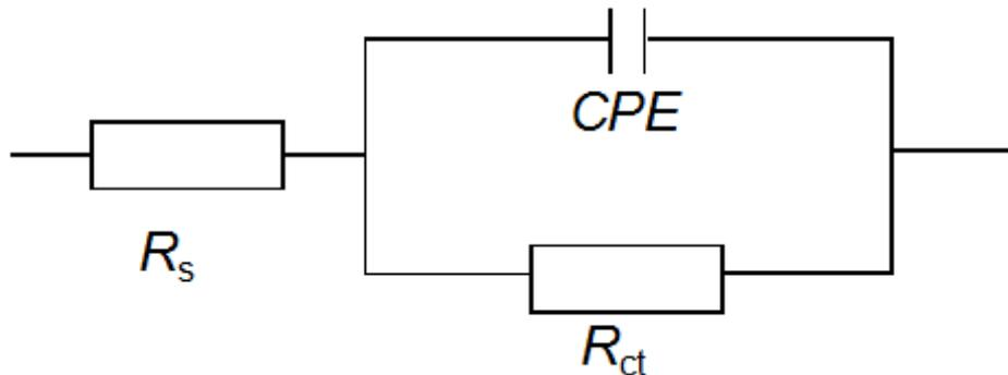
**Figure 5.** Suggested equivalent circuit model for the studied system.
