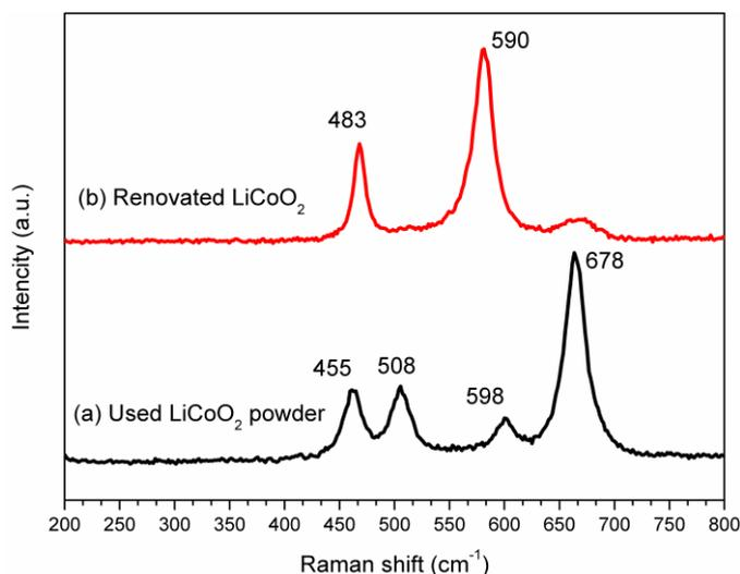
**Figure 6.** Raman spectra for (a) the spent LiCoO<sub>2</sub> powder and (b) the renovated LiCoO<sub>2</sub> powder.
