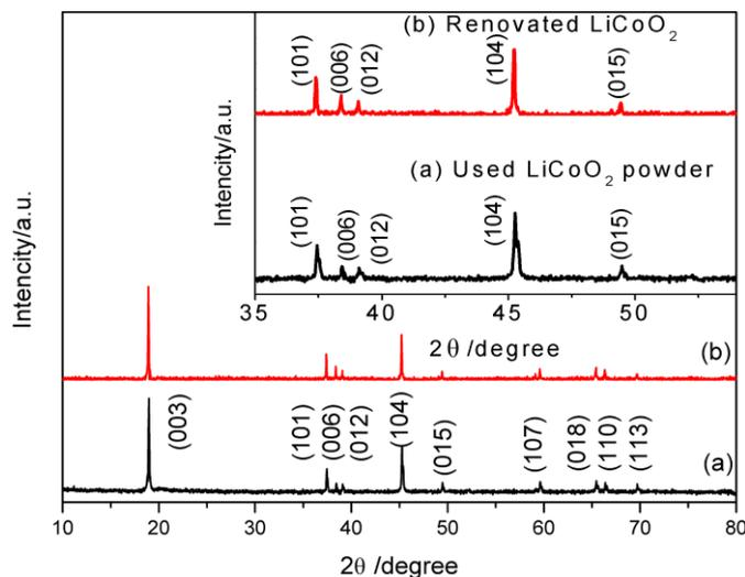
**Figure 3.** X-ray diffraction patterns for (a) the spent  $\text{LiCoO}_2$  powder and (b) the renovated  $\text{LiCoO}_2$  powder.
