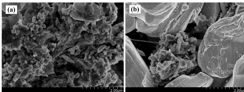
**Figure 4.** SEM images for the morphology of (a) the spent  $\text{LiCoO}_2$  powder and (b) the renovated  $\text{LiCoO}_2$  powder.
