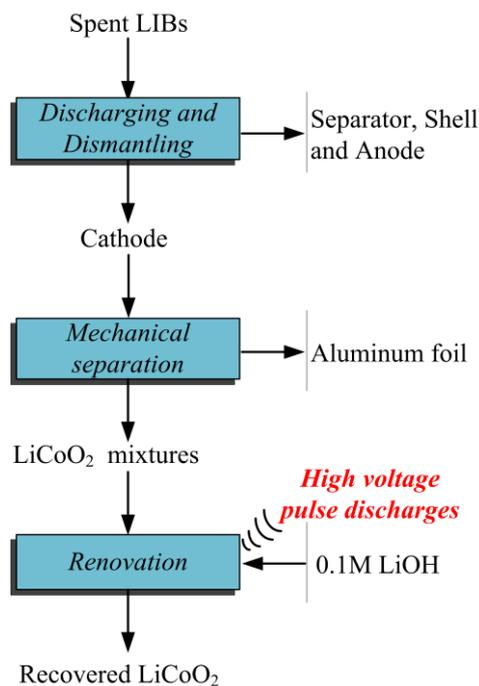
**Figure 1.** Schematization of renovated LiCoO<sub>2</sub> cathode material by an aqueous pulsed discharge plasma
