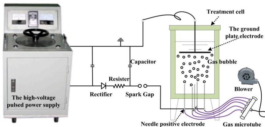
**Figure 2.** Schematic diagram of the experimental set-up
