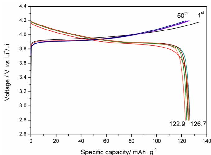
**Figure 7.** Charge-discharge characteristics of the renovated  $\text{LiCoO}_2$  powder at  $C/5$ .
