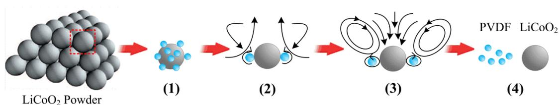
**Figure 5.** The flow field analysis of  $\text{LiCoO}_2$  particles and PVDF
