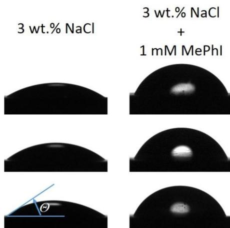
**Figure 7.** The shapes of the deionized water droplets (one out of three samples) for the contact angle ( $\theta$ ) analysis on the Cu surfaces previously immersed for 1h in non-inhibited solution and MePhI-inhibited solution (three replicate measurements for both cases).
