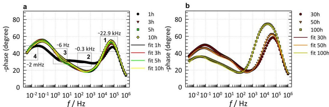
**Figure 5.** Measured (dotted) and fitted (solid lines) phase angle EIS spectra using the EEC model in Fig. 4 for the measurements after a) 1h, 3h, 5h, and 10h and b) 30h, 50h, and 100h of immersion.
