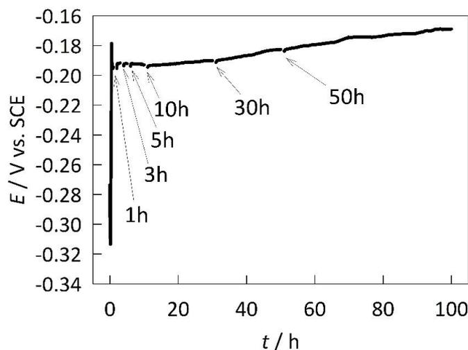
**Figure 2.** Chronopotentiometric measurements of Cu in 3 wt.% NaCl containing 1 mM MePhI.
