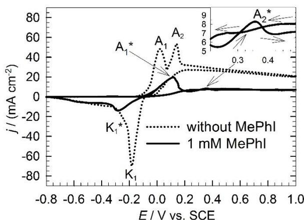
**Figure 1.** Cyclic voltammograms for Cu in 3 wt.% NaCl with or without 1 mM MePhI.
