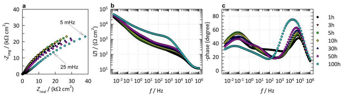
**Figure 3.** EIS measurements for Cu in 3 wt.% NaCl containing 1 mM MePhI measured after 1, 3, 5, 10, 30, 50, and 100h of immersion: a) Nyquist and b, c) Bode plots.
