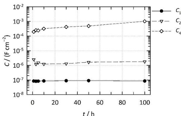
**Figure 6.** Calculated  $C$  values according to  $C_x = (R_x Q_x) n_x / R_x$  using the ascertained  $Q, R,$  and  $n$  values in the fitting procedure in Table 1.
