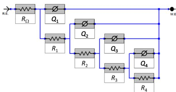
**Figure 4.** The  $R_{\Omega}(Q_1(R_1(Q_2(R_2(Q_3(R_3(R_4Q_4)))))))$  model used to fit the experimental EIS spectra obtained after 1, 3, 5, 10, 30, 50, and 100h of immersion. This model induced the lowest  $\chi^2$ . R.E. and W.E. represent the reference and working electrodes, respectively.
