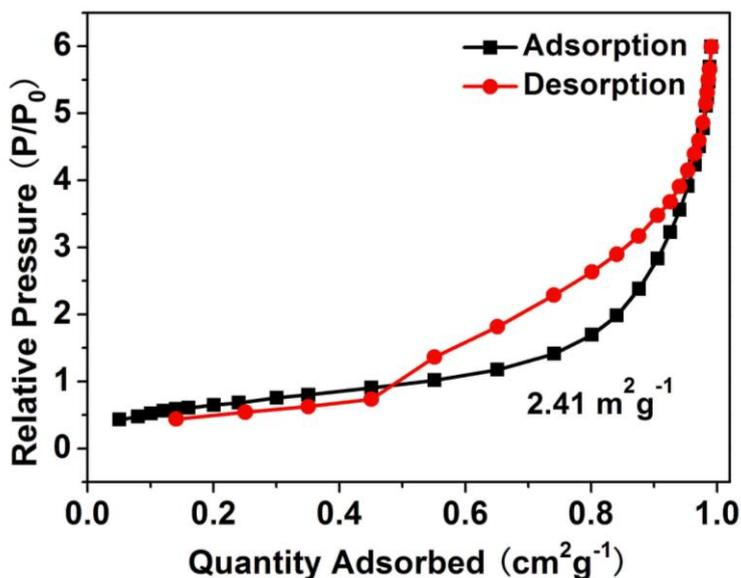
**Figure 2.** Nitrogen adsorption-desorption isotherm of CoS<sub>2</sub> nanodendrites.
