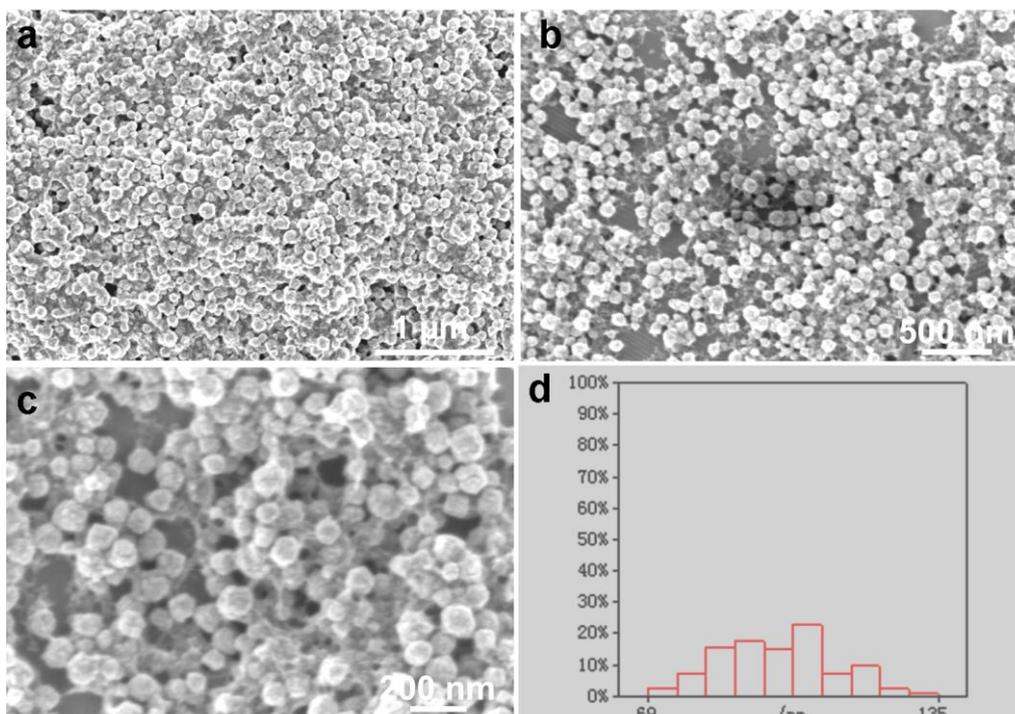
**Figure 3.** (a-c) FESEM image of ultrathin CoS<sub>2</sub> nanodendrite with different magnification prepared at 180 °C for 24 h. (d) The size distribution of CoS<sub>2</sub> nanodendrites.
