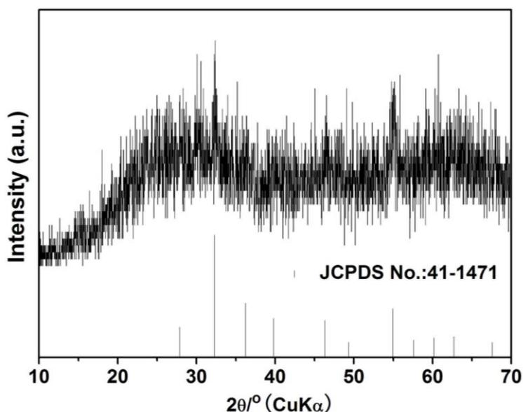
**Figure 1.** XRD patterns of CoS<sub>2</sub> nanodendrite. Vertical lines at the bottom represent the standard PDF card of α-CoS<sub>2</sub>.
