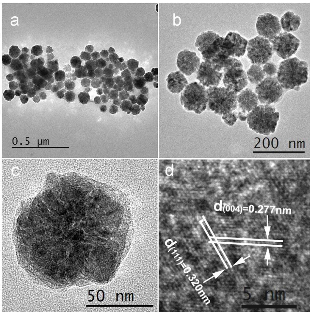
**Figure 4.** (a-b) Low and high magnification TEM image of  $\text{CoS}_2$  nanodendrites. (c) TEM image of a single  $\text{CoS}_2$  nanodendrite (d) HRTEM image of a single  $\text{CoS}_2$  nanodendrite.
