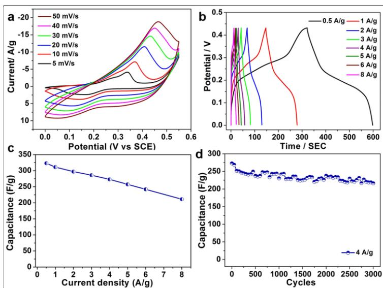
**Figure 5.** Electrochemical performance characterization of CoS<sub>2</sub> nanodendrites: (a) CV curves of CoS<sub>2</sub> nanodendrites modified electrode at different scan rates ranging from 5 to 50 mV s<sup>-1</sup>. (b) Galvanostatic charge-discharge curves of CoS<sub>2</sub> with various current densities. (c) The influence of current density to discharge rate performance. (d) Cycling performance of CoS<sub>2</sub> at a fixed current density of 4 A g<sup>-1</sup>.
