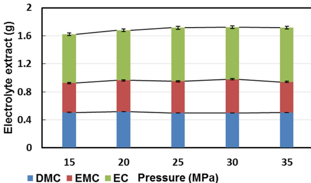
**Figure 3.** Compositions of the extracts corresponding to Fig. 2. green, top: EC; crimson, middle: EMC; blue, bottom: DMC
