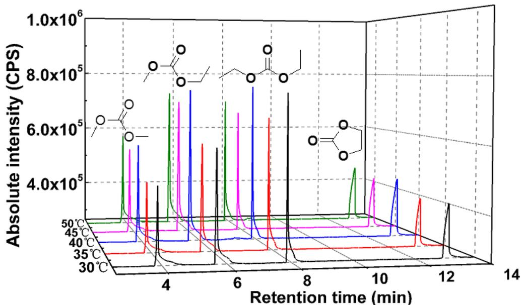
Figure 4. Chromatograms (GC-FID) of extracts with the course of temperature from carbonate mixture by supercritical CO<sub>2</sub>.
