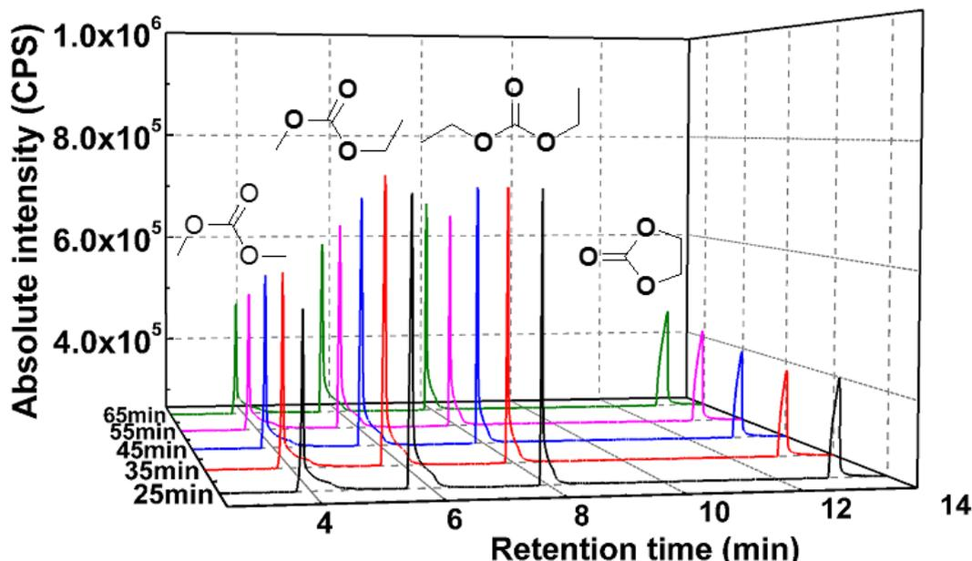
Figure 6. Chromatograms (GC-FID) of extracts with the course of time from carbonate mixture by supercritical CO<sub>2</sub>.
