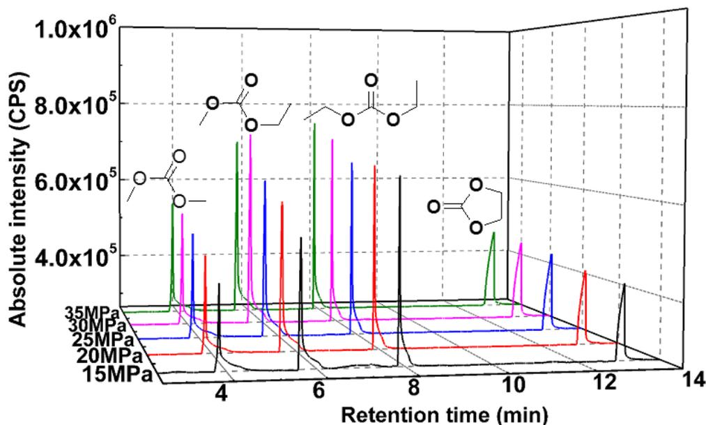
**Figure 2.** Chromatograms (GC-FID) of extracts with the course of pressure from carbonate mixture by supercritical CO<sub>2</sub>.
