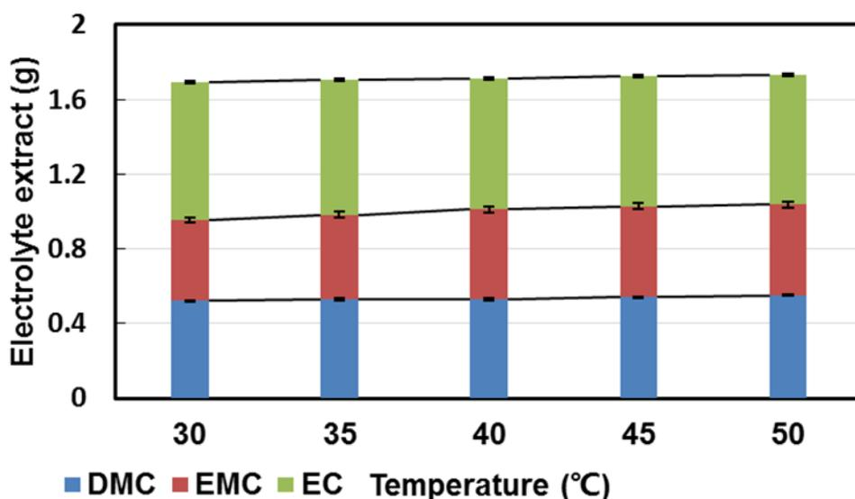
Figure 5. Compositions of the extracts corresponding to Fig. 4. green, top: EC; crimson, middle: EMC; blue, bottom: DMC.
