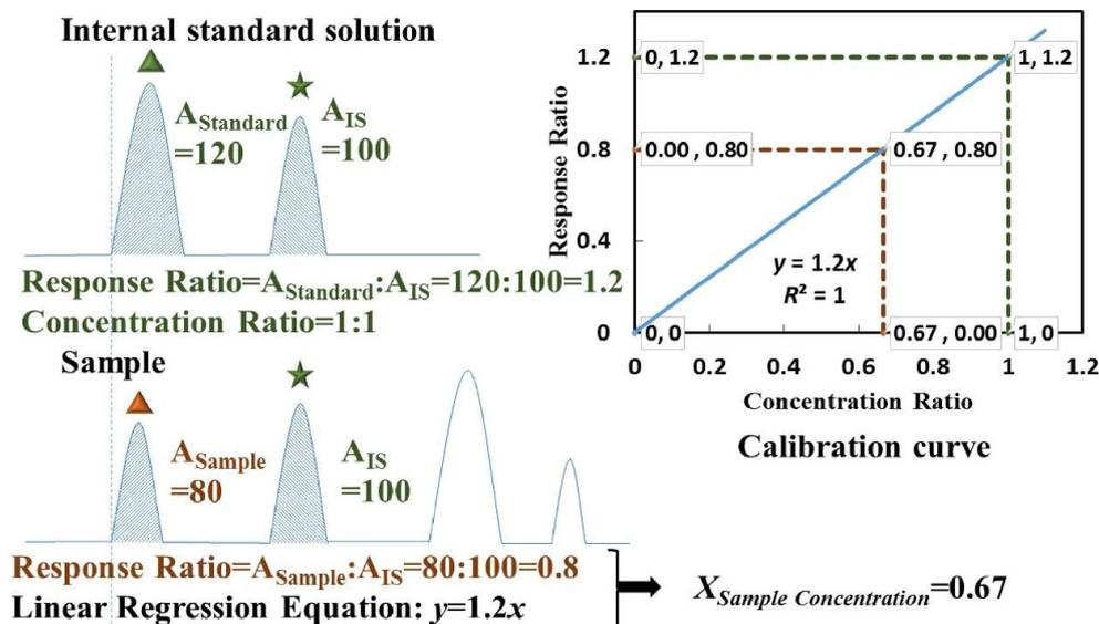
**Figure 1.** Schematic diagram of quantitate by internal standard calibration. The internal standard solution to be tested was first profiled by GC-FID. The peak area of the standard and internal standard was recorded as  $A_{Standard}$  and  $A_{IS}$ , respectively. Internal standard solutions were subsequently spiked into the extract. Their peak areas were recorded again as  $A_{Sample}$  and  $A_{IS}$ .
