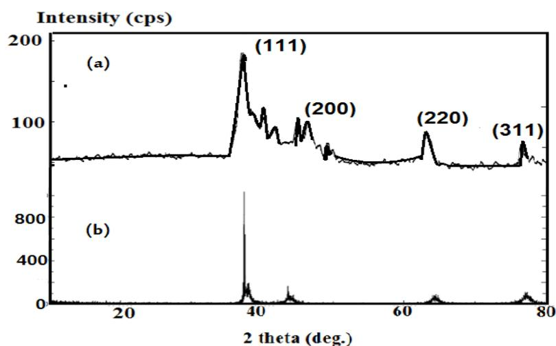
**Figure 6.** XRD patterns of Ag NPs prepared a) in the presence of glucose and b) in absence of glucose.
