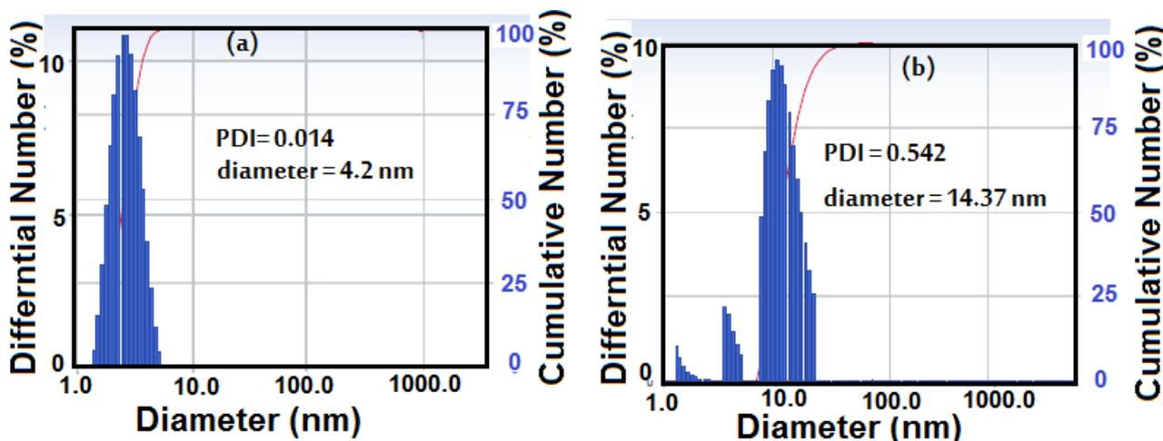
**Figure 3.** Particle size analysis of Ag NPs prepared a) in the presence of glucose and b) in absence of glucose.
