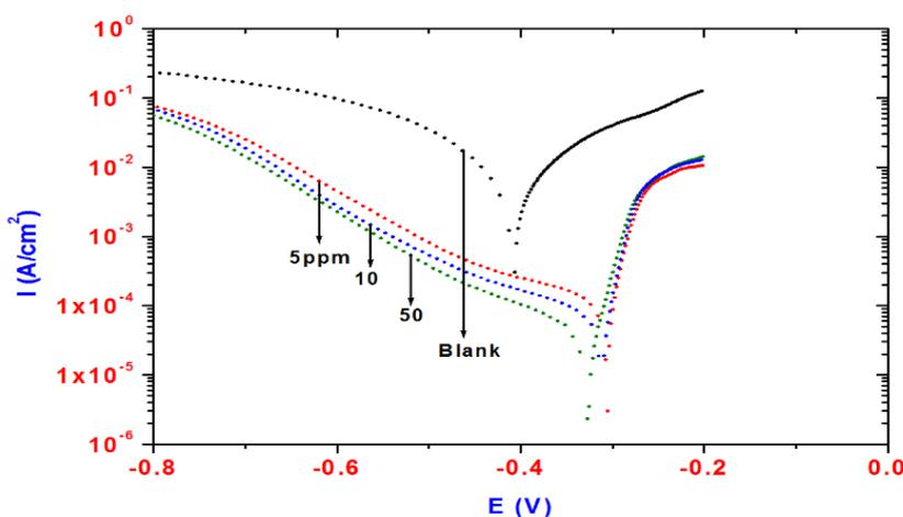
**Figure 8.** Polarization curves for steel in 1.0 M HCl in the presence of different concentrations of Ag NPs prepared in the presence of glucose.
