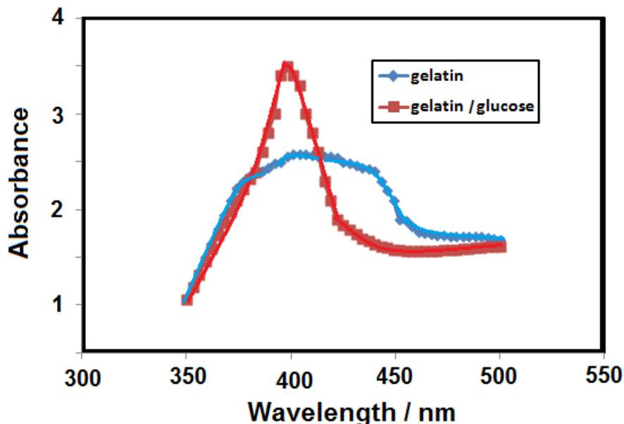
**Figure 2.** UV-visible Plasmon of the prepared Ag NPs in the presence of gelatin and glucose as capping and reducing agents.
