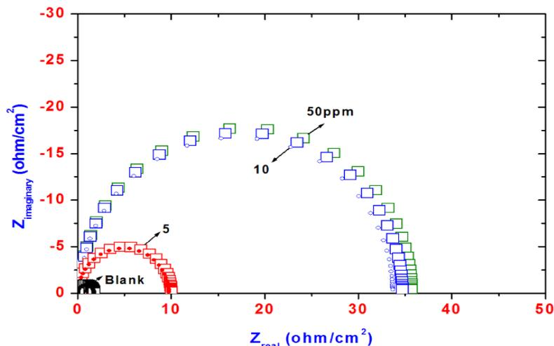
**Figure 9.** Nyquist plot for steel in 1.0 M HCl in the presence of different concentrations of Ag NPs prepared in the presence of glucose.
