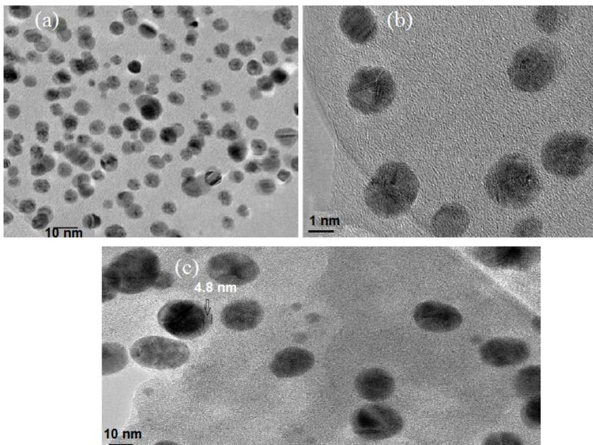
**Figure 4.** HRTEM micrographs of Ag NPs prepared of a) in the existence of glucose b) in absence of glucose and c) in presence of glucose and PVP.
