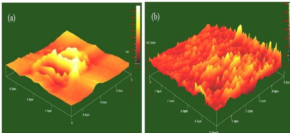
**Figure 5.** AFM photo of Ag NPs prepared a) in the presence of glucose and b) in absence of glucose.
