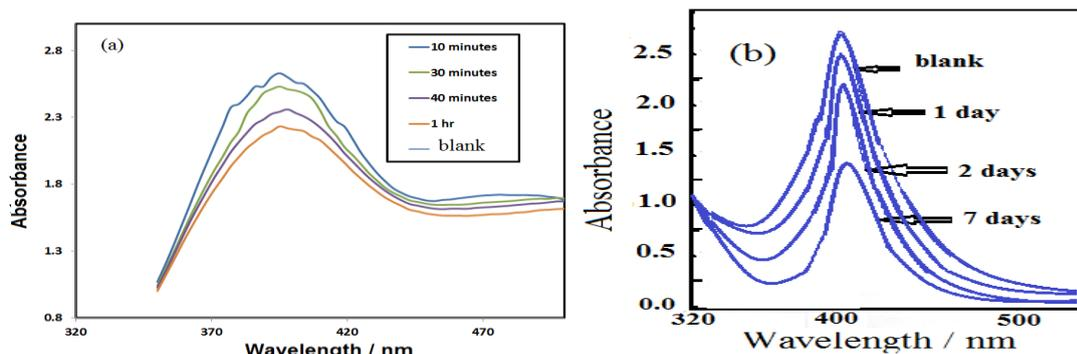
**Figure 7.** UV- visible spectra of Ag NPs prepared in a) absence of glucose and b) in the presence of glucose using 1 M HCl aqueous solution at different times.
