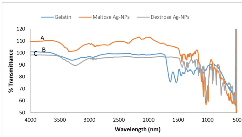
**Figure 4.** FT-IR spectra of gelatin (A), maltose-reduced Ag-NPs (B) and dextrose-reduced Ag-NPs (C).
