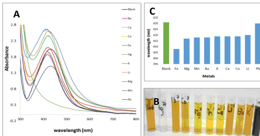
**Figure 5.** (A) Absorption spectra, (B) colorimetric response after addition of various metal ions to maltose-reduced Ag-NPs (From far left: Blank,  $\text{Hg}^{2+}$ ,  $\text{Pb}^{2+}$ ,  $\text{Co}^{2+}$ ,  $\text{Mg}^{2+}$ ,  $\text{Mn}^{2+}$ ,  $\text{Ca}^{2+}$ ,  $\text{Li}^+$ ,  $\text{Ba}^{2+}$ ,  $\text{K}^+$ , and  $\text{Fe}^{2+}$ ) and (C) the change in the SPR peak position.
