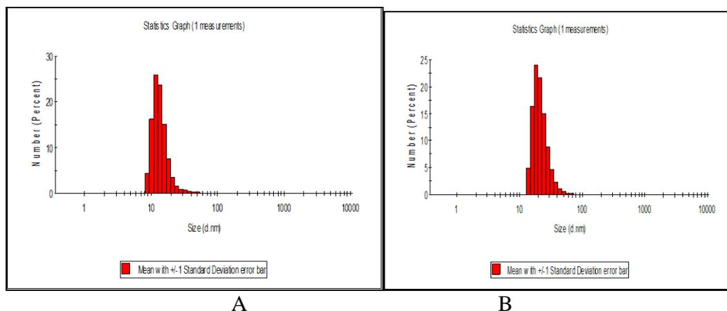
**Figure 3.** Hydrodynamic particle size distribution of maltose (A) and dextrose (B)-reduced Ag-NPs.
