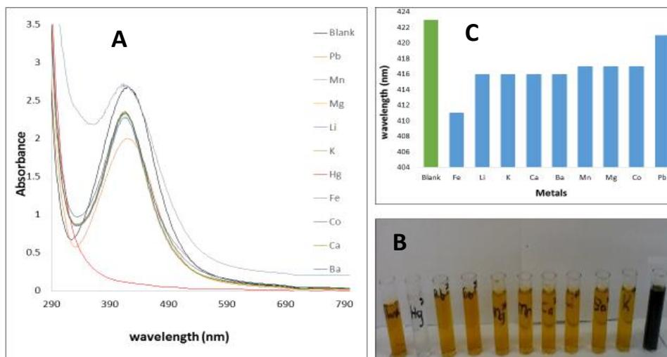
**Figure 6.** (A) Absorption spectra, (B) colorimetric response after addition of various metal ions to dextrose-reduced Ag-NPs (From far left: Blank,  $\text{Hg}^{2+}$ ,  $\text{Pb}^{2+}$ ,  $\text{Co}^{2+}$ ,  $\text{Mg}^{2+}$ ,  $\text{Mn}^{2+}$ ,  $\text{Ca}^{2+}$ ,  $\text{Li}^+$ ,  $\text{Ba}^{2+}$ ,  $\text{K}^+$ ,  $\text{Cr}^{3+}$  and  $\text{Fe}^{2+}$ ) and (C) the change in the SPR peak position.
