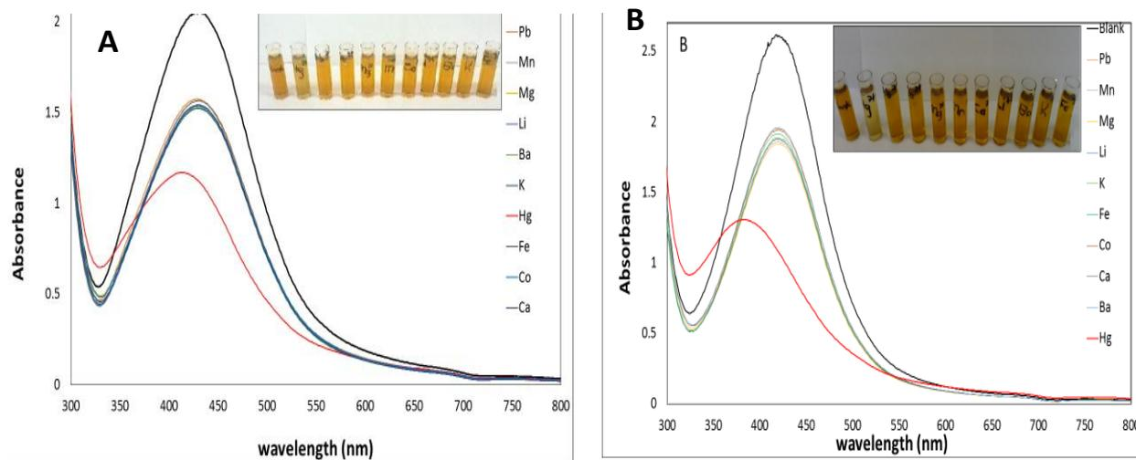
**Figure 7.** Absorption spectra of (A) Maltose and (B) dextrose reduced Ag-NPs after the addition of  $10^{-3}$  M metal ions (inset: colorimetric response; From far left: Blank,  $\text{Hg}^{2+}$ ,  $\text{Pb}^{2+}$ ,  $\text{Co}^{2+}$ ,  $\text{Mg}^{2+}$ ,  $\text{Mn}^{2+}$ ,  $\text{Ca}^{2+}$ ,  $\text{Li}^{+}$ ,  $\text{Ba}^{2+}$ ,  $\text{K}^{+}$ ,  $\text{Cr}^{3+}$  and  $\text{Fe}^{2+}$ ).
