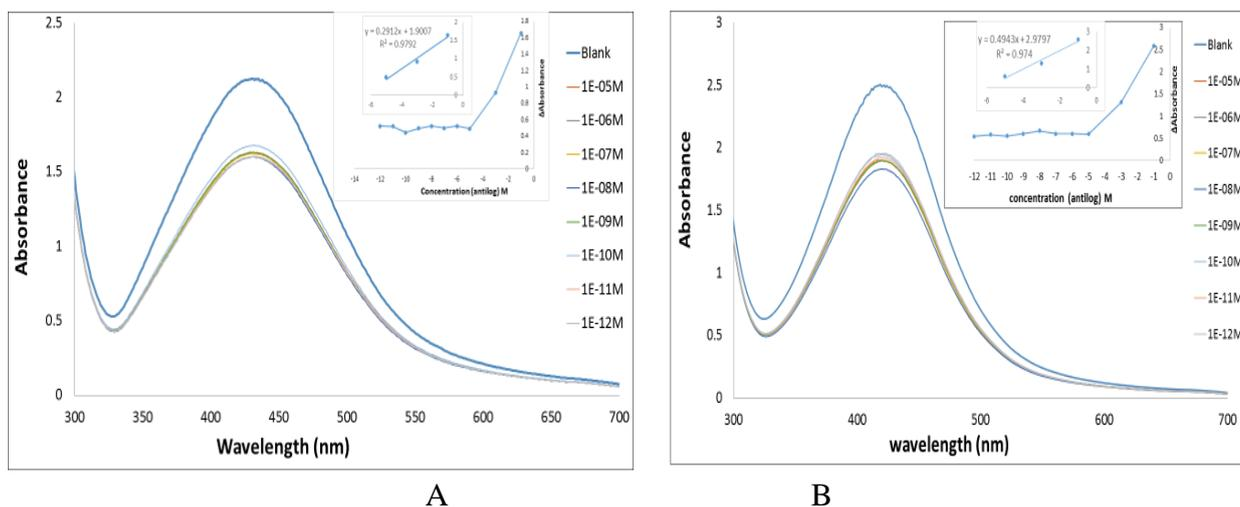
**Figure 8.** Absorption spectra of (A) maltose and (B) dextrose- reduced Ag-NPs after addition of various concentrations of  $Hg^{2+}$  ions. (Inset: Linear plot of change in absorbance at different concentrations)
