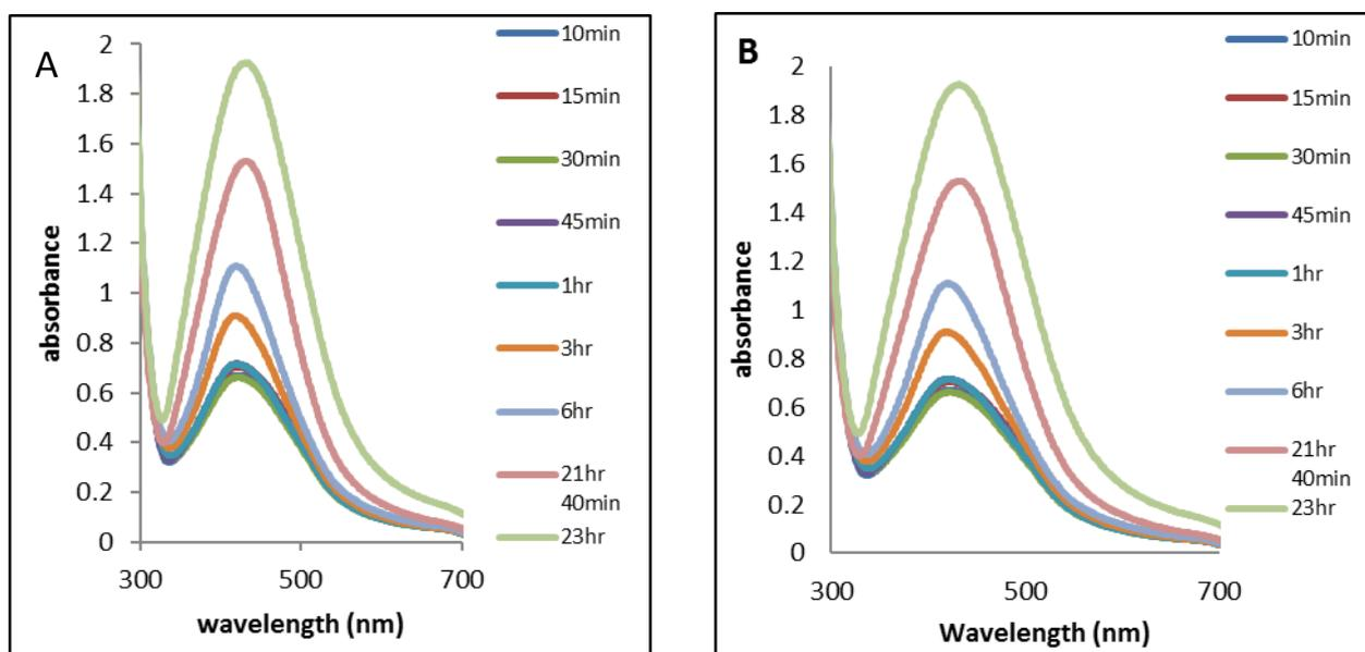
**Figure 1.** Absorption spectra of maltose (A) and dextrose-reduced (B) Ag-NPs at different reaction time.
