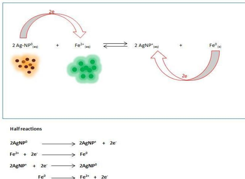
**Scheme 5.** Mechanism for the formation of green colour after addition of  $\text{Fe}^{2+}$  to the solution of Ag-NPs.
