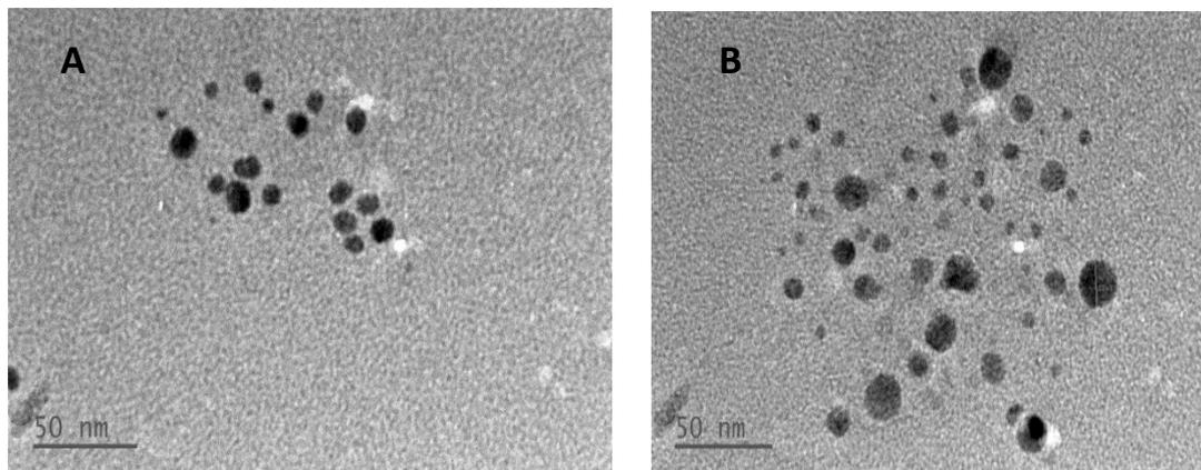
**Figure 2.** Typical TEM micrographs of maltose (A) and dextrose (B) -reduced Ag-NPs.
