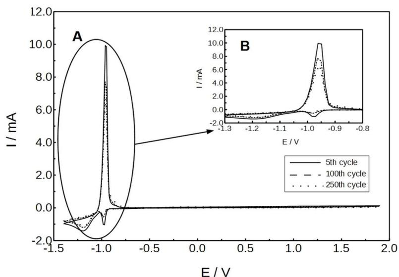
**Figure 6.** Cyclic voltammograms (0.5 V/s) for Pb/Cu/RVC electrode subjected to continuous potential cycling in 4.9 M (37.5 wt %) H<sub>2</sub>SO<sub>4</sub> (A). Sulfate region in greater detail (B).
