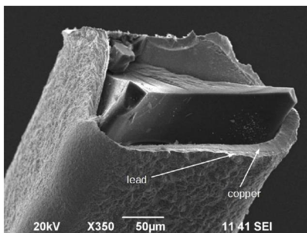
**Figure 4.** SEM image of a cross-section of the RVC matrix modified with double-metal copper-lead layer.
