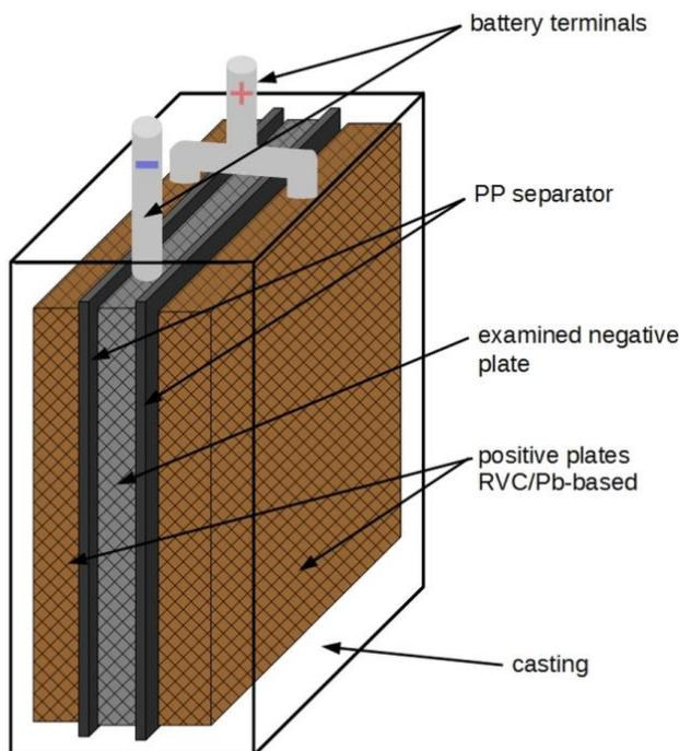
**Figure 2.** Scheme of three-plate lead-acid cell for negative plate testing.
