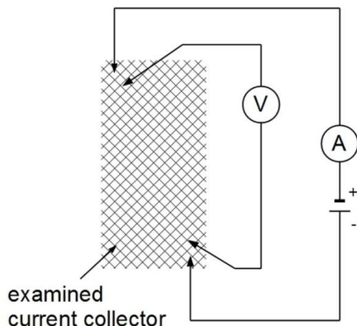
**Figure 1.** Scheme of the system for measuring the electrical conductivity.
