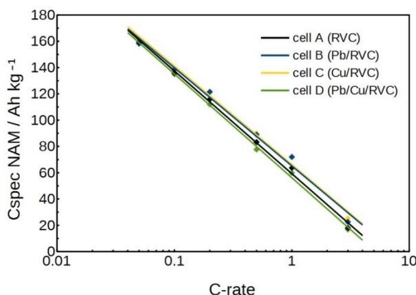
**Figure 9.** Dependence of apparent specific capacity on discharging current for different batteries.
