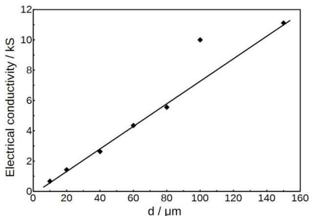
**Figure 7.** Dependence of electrical conductivity on thickness of the copper layer (d) for Cu/RVC.
