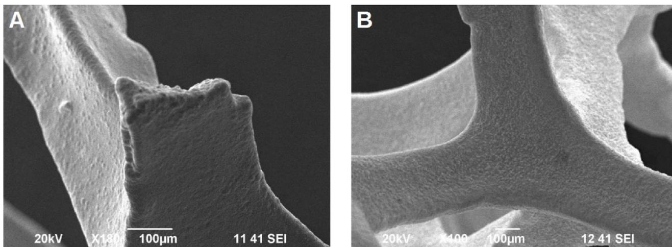
**Figure 3.** SEM images of RVC matrix modified with copper (A) and double-metal, copper-lead layer(B).
