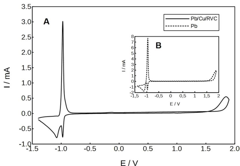
**Figure 5.** Cyclic voltammogram in 4.9 M (37.5 wt %) H<sub>2</sub>SO<sub>4</sub> in the full potential range (-1.4 to 1.9 V), scan rate 0.05 V s<sup>-1</sup> for Pb/Cu/RVC electrode (A) for solid Pb electrode (B).
