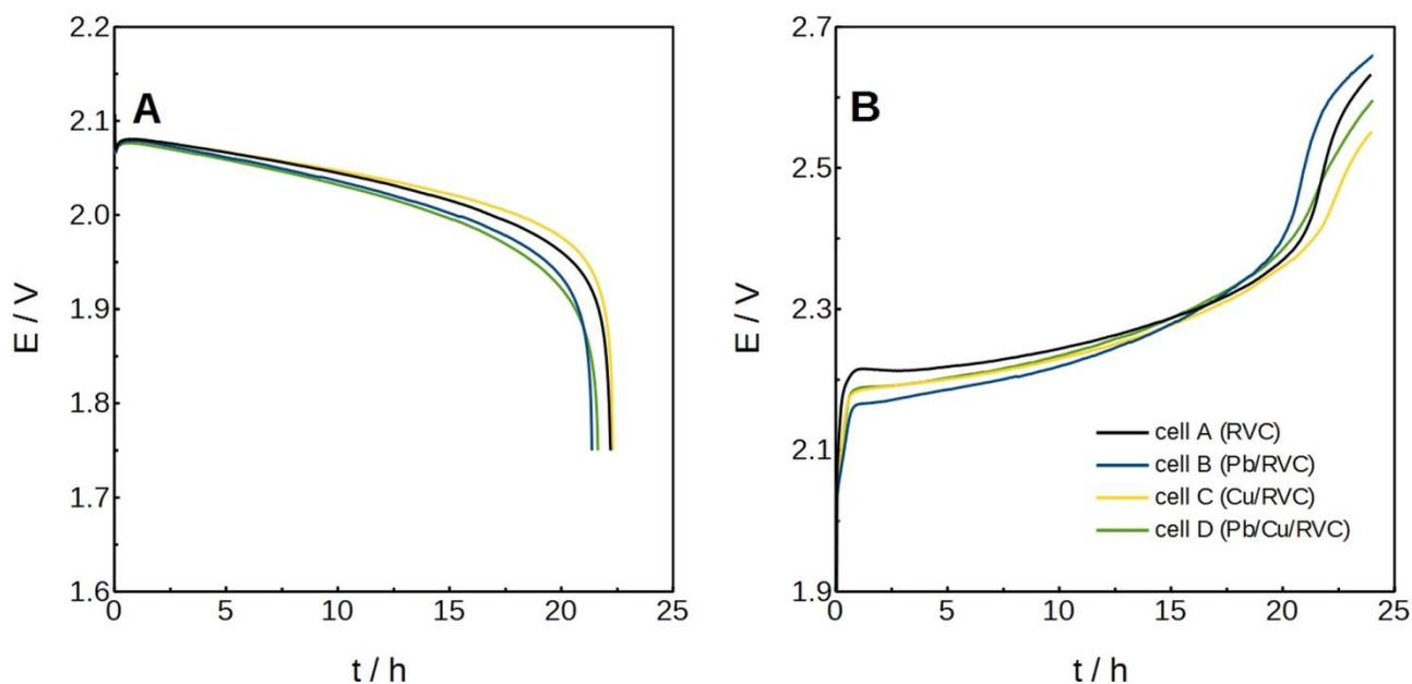
**Figure 8.** Discharging (A) / charging (B) characteristic of different batteries at constant discharging/charging current 0.05 C.
