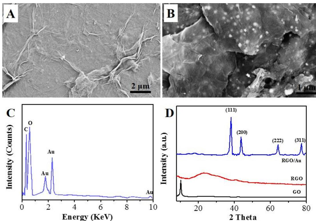
**Figure 2.** (A) SEM image of RGO, (B) SEM image and (C) EDX spectrum of RGO/Au composite, (D) XRD patterns of GO, RGO and RGO/Au.
