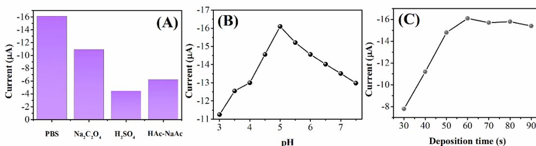
**Figure 5.** Effects of (A) electrolyte types, (B) pH values of PBS and (C) electrodeposition time on the reduction performance of ternatin.
