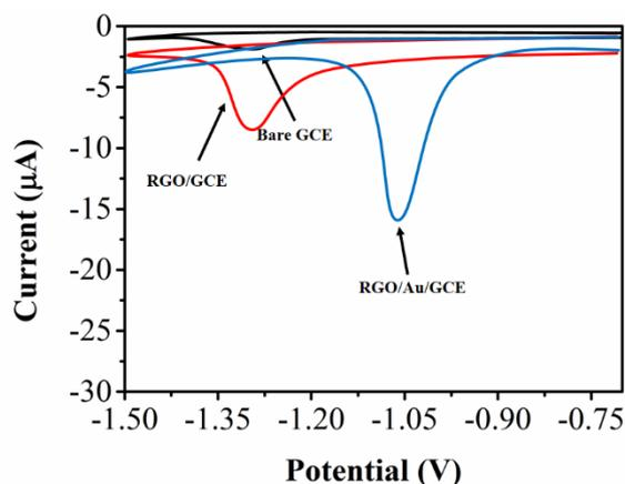
**Figure 4.** Cyclic voltammograms of 100  $\mu\text{M}$  ternatin in PBS obtained on bare GCE, RGO/GCE and RGO/Au/GCE electrodes.
