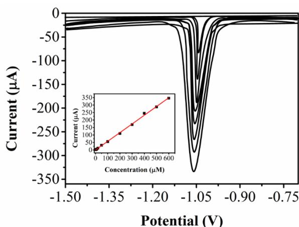
**Figure 6.** DPV curves of ternatin under various concentrations obtained on RGO/Au/GCE electrode. Inset: plot of reductive peak current in the function of ternatin concentration.
