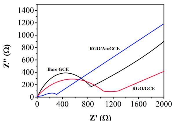
**Figure 3.** Nyquist diagrams obtained on bare GCE, RGO/GCE and RGO/Au/GCE electrodes.
