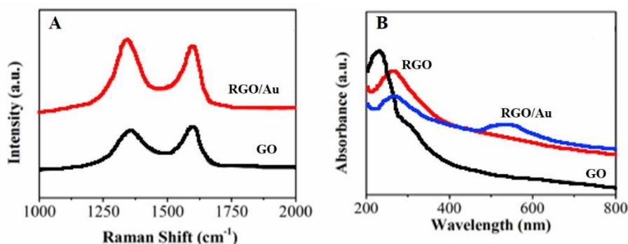
**Figure 1.** (A) Raman spectra of GO and RGO/Au. (B) UV-vis spectra of GO, RGO and RGO/Au nanocomposite.
