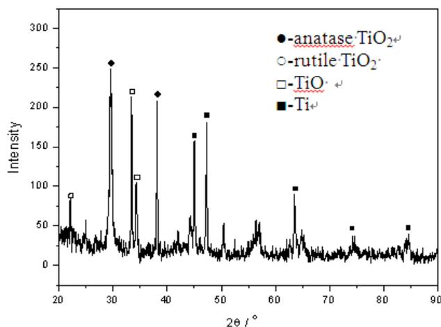
**Figure 1.** XRD patterns of Ti/TiO<sub>2</sub> electrode
