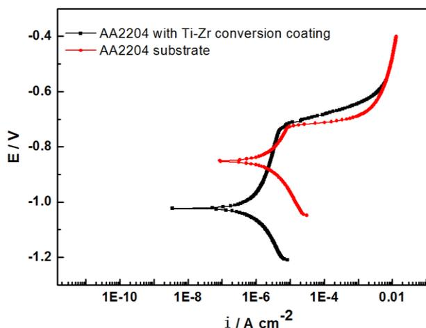
**Figure 4.** Polarization curves for AA2024 with and without Ti-Zr conversion in 5% NaCl solution
