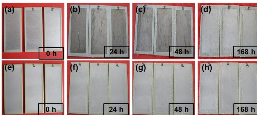
**Figure 1.** Photographs of AA2024 substrate (a-d) and AA2024 with Ti-Zr conversion coating (e-h) suffering the NSS test with different times.
