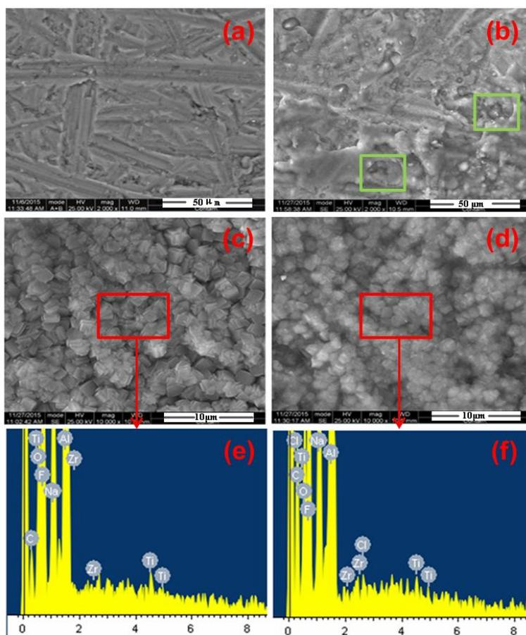
**Figure 2.** SEM images of AA2024 substrate before (a) and after (b) the 168h NSS test; SEM images of AA2024 with Ti-Zr conversion coating before (c) and after (d) the 168 h NSS test and the corresponding EDS spectra (e) and (f).
