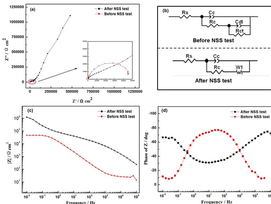
**Figure 6.** Nyquist diagram (a), Bode plots (c-d) of AA2024 Ti-Zr conversion coating in 5% NaCl solution before and after the 168 h NSS test, and the corresponding equivalent circuits (b).
