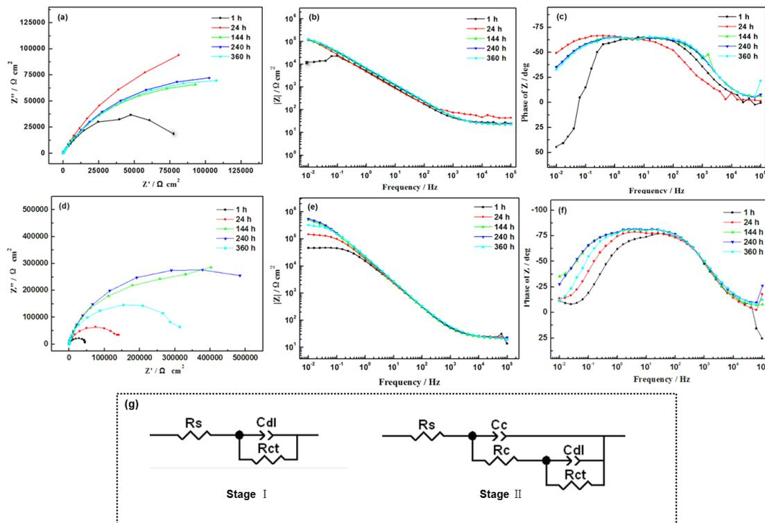
**Figure 7.** Nyquist and bode plots of AA2024 substrate (a-c) and AA2024 with Ti-Zr conversion coating (d-f) in 5% NaCl solution with different immersion time, and the corresponding equivalent circuits for different stages (g)
