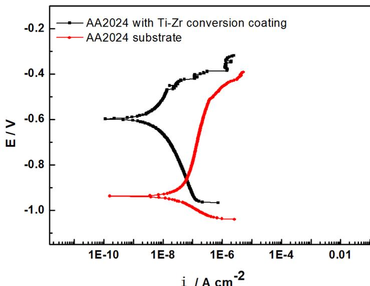
**Figure 5.** Polarization curves for AA2024 with and without the Ti-Zr conversion coating in 5% NaCl solution after the 168 h NSS test
