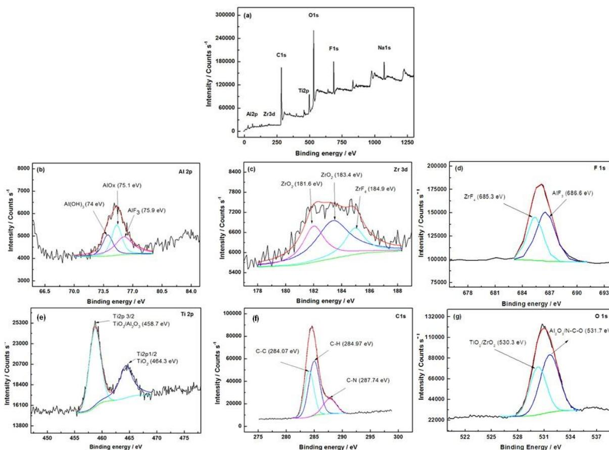
**Figure 3.** XPS spectrum of AA2024 with Ti-Zr conversion coating (a) and the corresponding high resolution de-convoluted spectra of Al 2p (b), Zr 3d (c), F 1s (d), Ti 2p (e), C 1s (f) and O 1s (g).
